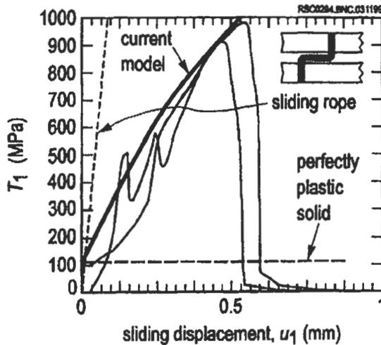
**Figure 8.29** Comparison of the Cox model for the shear traction in a single stitch (thick curve) with two experimental curves showing measured traction in a Kevlar stitch in a carbon/epoxy laminate determined by Turrentini (1996) (from Cox, 1999).
