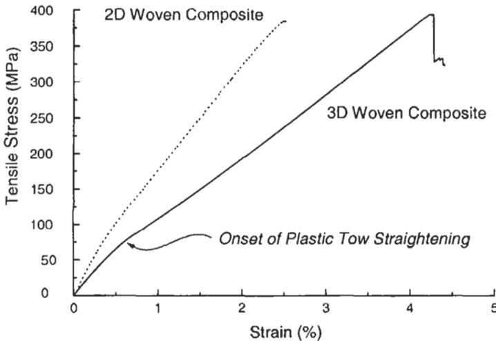
**Figure 5.7** Tensile stress-strain curves for a 2D and 3D woven composite.
