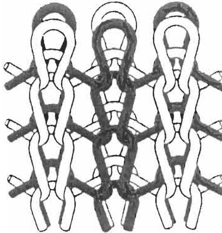
**Figure 2.24** Schematic of a multilayer knitted fabric
