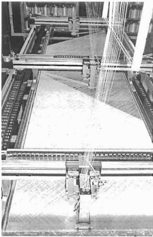
**Figure 2.29** Examples of the fibre placement heads (courtesy of LIBA-Maschinenfabrik GmbH)
