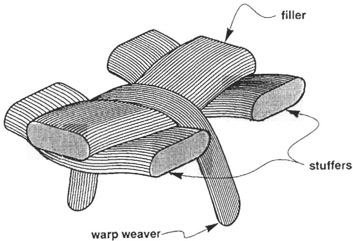
**Figure 5.4** Schematic of crimping of a surface tow (or filler) by a z-binder yarn (or warp weaver) Cox et al. (1994).
