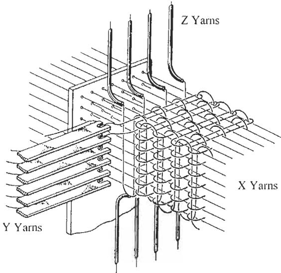
**Figure 2.9** Illustration of Fukuta's et al. (1974) equipment for the manufacture of 3D non-woven preforms.
