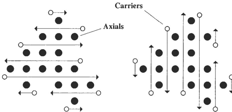
**Figure 2.17** Schematic of the 2-Step braiding process
