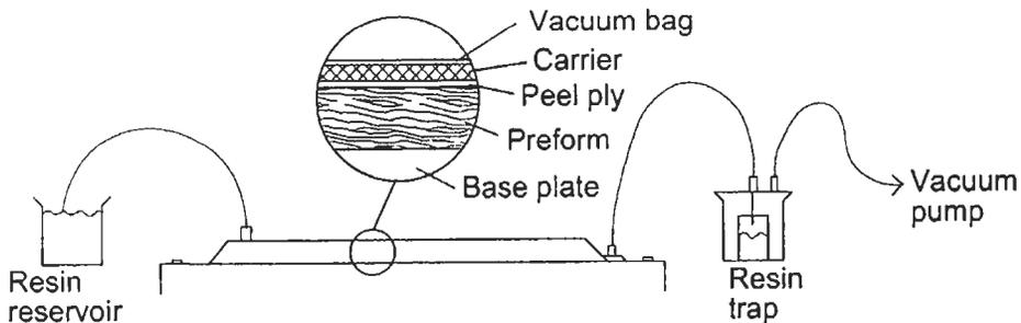
**Figure 3.3** Schematic of the SCRIMP process
