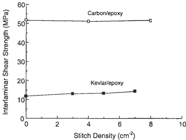
**Figure 8.9** Effect of stitch density on the apparent interlaminar shear strength,  $\tau$ , of Kevlar/epoxy and carbon/epoxy composites (data for the Kevlar/epoxy and carbon/epoxy is from Cholarkara et al. (1989) and Jain and Mai (1997) respectively).
