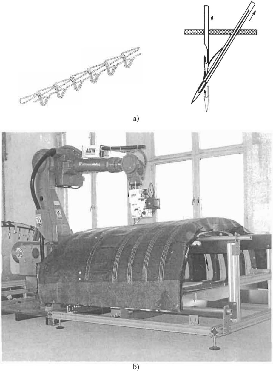
**Figure 2.32** a) Illustration of one-sided stitching technique, b) Example of commercially available robotic, one-sided stitching machine (courtesy of Altin Nähtechnik GmbH)
