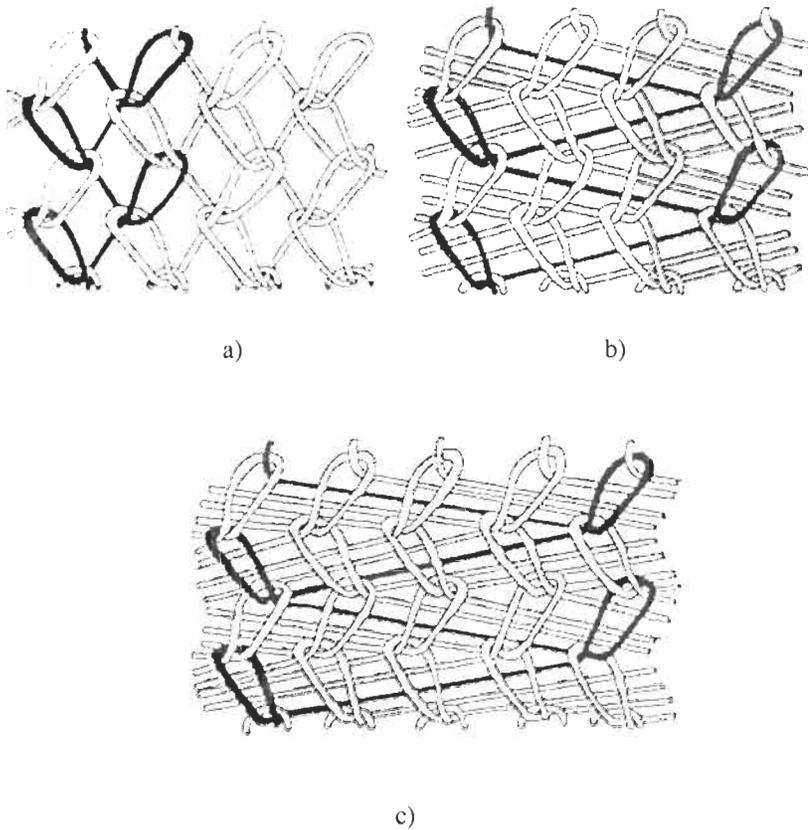
**Figure 7.5** Illustration of warp knit a) denbigh, b) 1x3 single cord, and c) 1x4 single cord architectures
