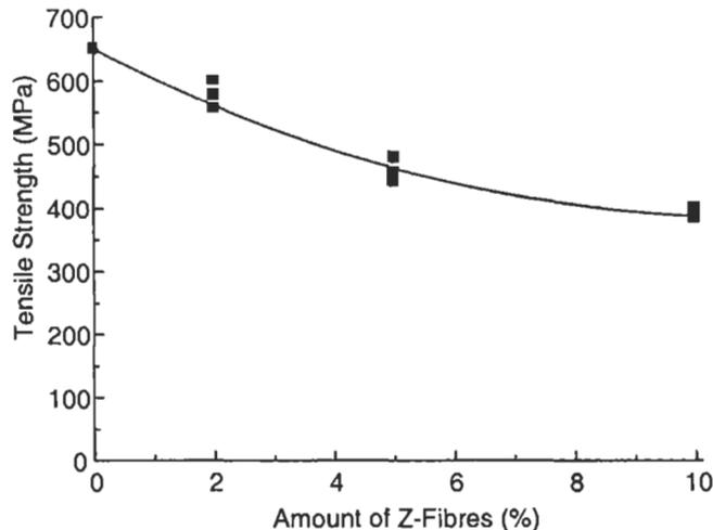
**Figure 9.6** Effect of Z-fiber<sup>TM</sup> content on the tensile strength of a carbon/epoxy composite. Adapted from Freitas et al. (1996)
