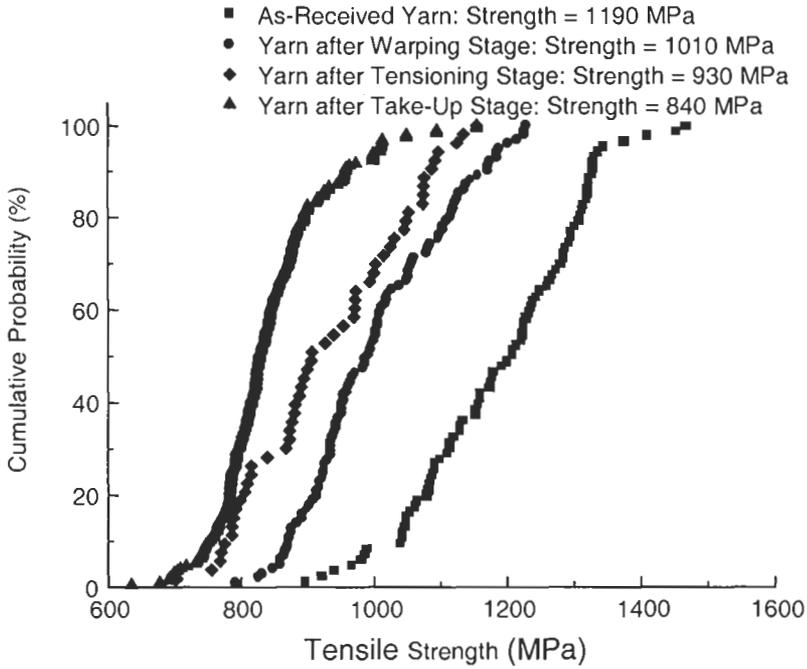
**Figure 5.3** Cumulative probability distribution plots of the tensile strength of a 300 tex E-glass yarn determined after different stages of the 3D weaving process. The average tensile strength value of the yarn after each weaving stage is shown (Adapted from Lee et al., 2002).
