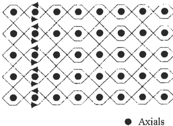
**Figure 2.20** Schematic of the multilayer interlock braiding process
