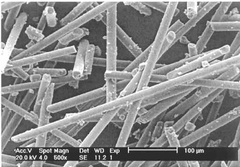
**Figure 5.2** Fragments of broken glass fibres caused by 3D weaving.
