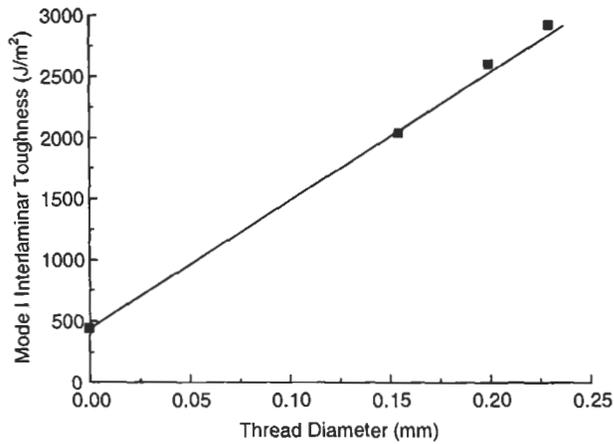
**Figure 8.20** The effect of stitch denier on the mode I interlaminar fracture toughness of a carbon/epoxy composite. The composite was stitched with Kevlar thread to an areal density of  $4/\text{cm}^2$  (Data from Jain & Mai, 1997).
