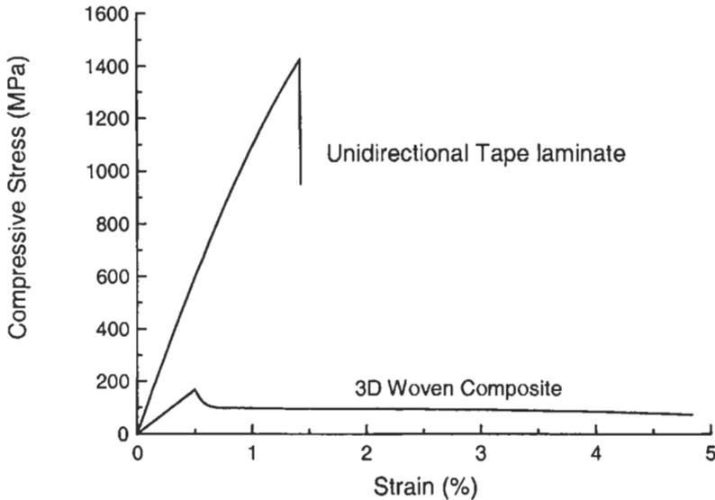
**Figure 5.17** Compression stress-strain curves for a unidirectional tape laminate and a 3D woven composite (The curves for the laminate and 3D composite are from Daniel and Ishai (1994) and Cox et al. (1992), respectively).
