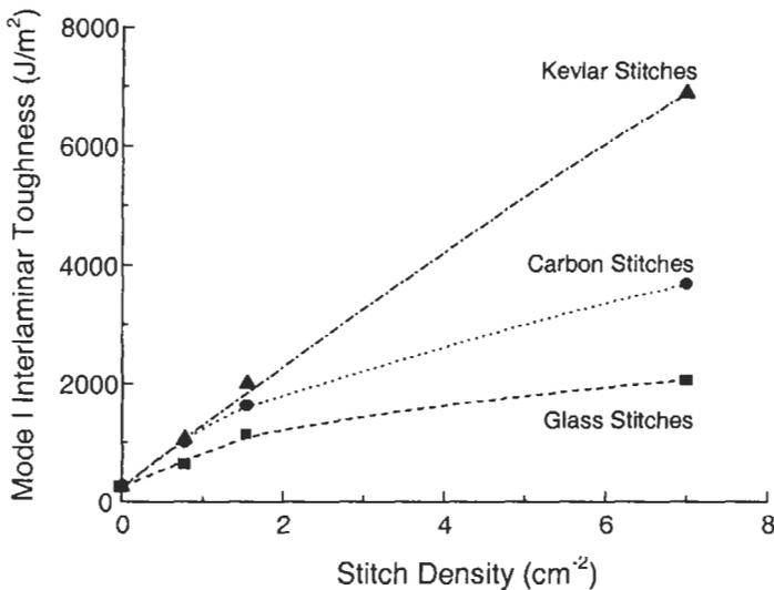
**Figure 8.19** The effect of stitch density and stitch material on the mode I interlaminar fracture toughness of a carbon/epoxy composite (Data from Morales, 1990).
