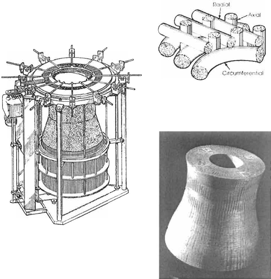
**Figure 2.8** Illustration of Aerospatiale method for producing 3D orthogonal non-woven preforms and an example of a consolidated preform
