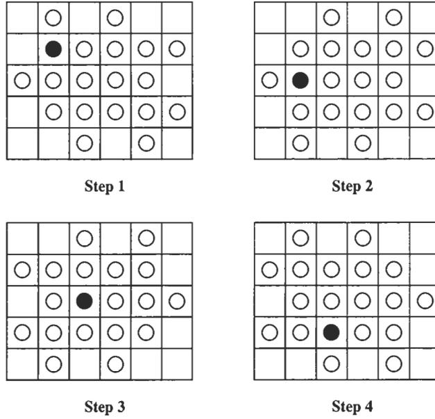
**Figure 2.15** Schematic of the 4-Step braiding process
