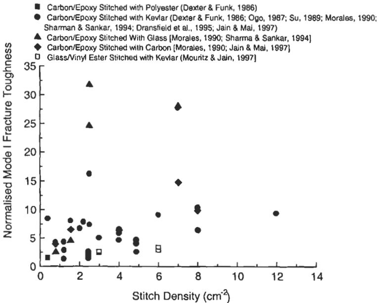
**Figure 8.21** The effect of stitch density on the normalised mode I interlaminar fracture toughness ( $G_{IR}/G_{IC}$ ) for a variety of stitched composites (Mouritz and Jain, 1999).
