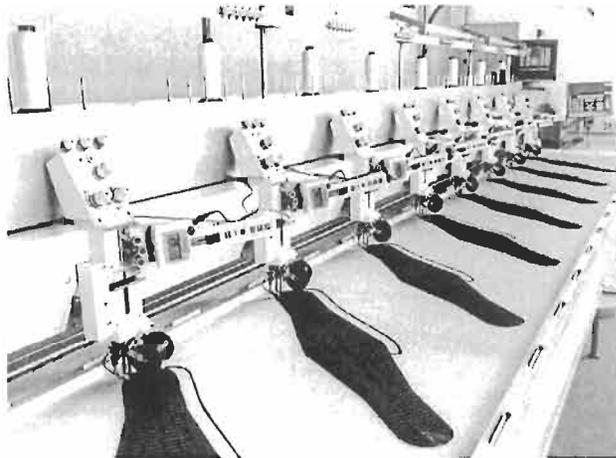
**Figure 2.35** Multiple preform manufacture with automated technical embroidery equipment (courtesy of Hightex GmbH)
