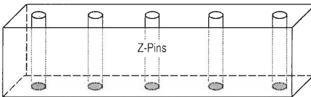
**Figure 9.1** Schematic illustration of a z-pinned composite
