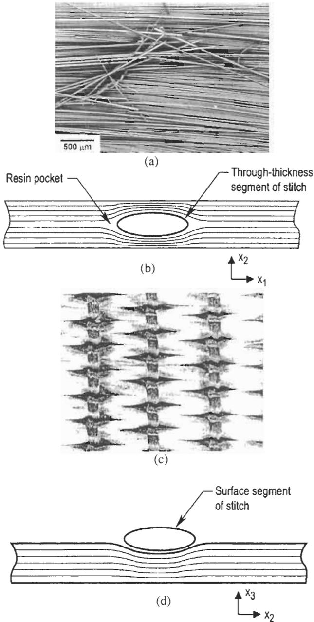
**Figure 8.4** Photographs and illustrations of stitching damage. (a) Dry woven fabric showing broken fibres caused by stitching. (b) Schematic and (c) photograph showing the local misalignment of fibres around a stitch. From Mouritz and Cox (2000) and Wu and Liao (1994), respectively. (d) Schematic of fibre crimping caused by stitching. (From Mouritz and Cox, 2000).
