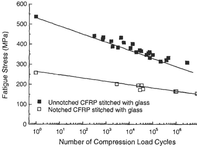
**Figure 8.13** A comparison of measured fatigue data points against theoretical S-N curves for two types of stitched carbon/epoxy composites fatigued under compression-compression loading (Data for the upper and lower data points are from Vandermeij et al. (1991) and Portanova et al. (1992), respectively).
