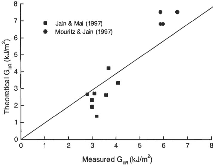
**Figure 8.28** Plot of measured against theoretical  $G_{IIIR}$  values for stitched composites. The theoretical  $G_{IIIR}$  values were determined using the Jain and Mai models. The closer the data points are to the straight line the better the agreement between the measured and theoretical  $G_{IIIR}$  value (from Mouritz and Jain, 1999).
