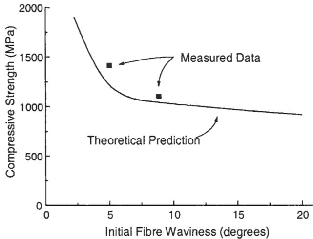
**Figure 9.8** Effect of maximum fibre misalignment angle caused by z-pin reinforcement on the compressive strength of a unidirectional carbon/epoxy composite. The curve shows a theoretical prediction and the points are experimentally measured values (Adapted from Steeves and Fleck, 1999a).
