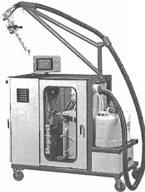
**Figure 3.4** Megaject RTM-Pro injection machine (photo courtesy of Plastech T.T. Ltd, UK)
