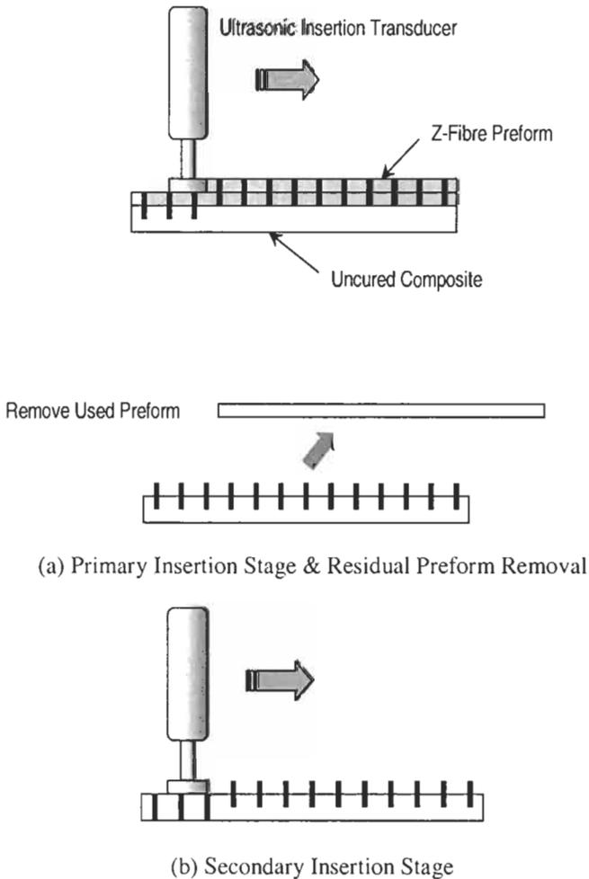
**Figure 9.3** Schematic of the Z-fibre<sup>TM</sup> insertion process using UAZ. (Adapted from Freitas et al., 1996)
