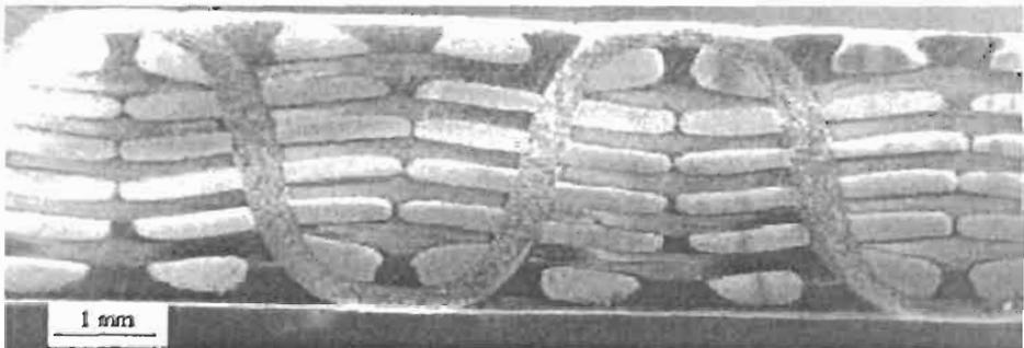
(c) Micrograph of cross section B-B showing true path of the z-binder and distorted filler yarns
