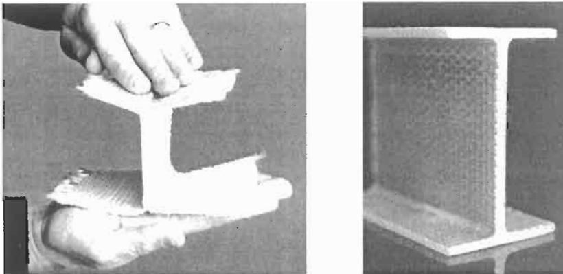
**Figure 2.7** Formation of composite I-beam from a flat multilayer preform (courtesy of the Cooperative Research Centre for Advanced Composite Structures, Ltd)
