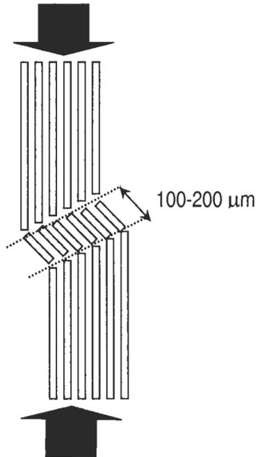
**Figure 5.15** Schematic of a kink band in a compressed fibre tow
