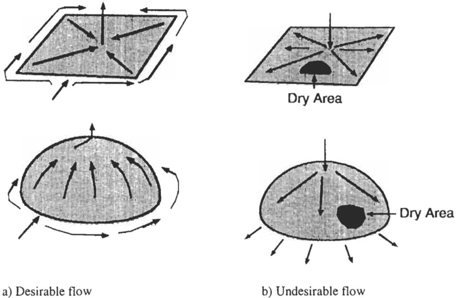
**Figure 3.6** Desirable and undesirable resin flow paths
