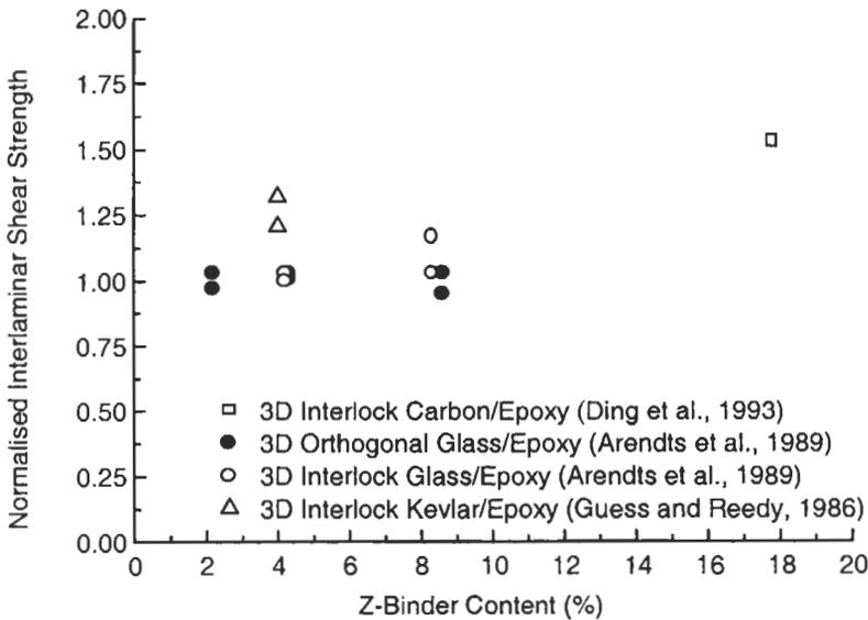
**Figure 5.18** Plot of normalised interlaminar shear strength against z-binder content for various 3D woven composites.
