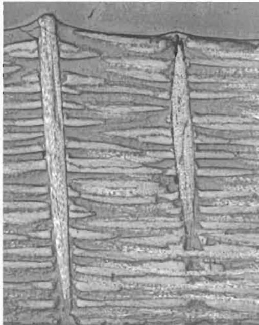
**Figure 9.4** Z-pins in a composite (Courtesy of the Cooperative Research Centre for Advanced Composite Structures Ltd)
