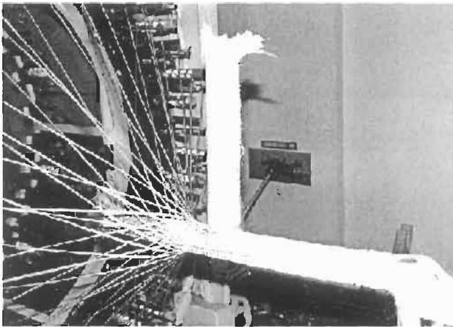
**Figure 2.14** (a) Schematic of braiding over a moving mandrel, b) Example of braiding over a T-shaped mandrel (courtesy of the Cooperative Research Centre for Advanced Composite Structures, Ltd)
