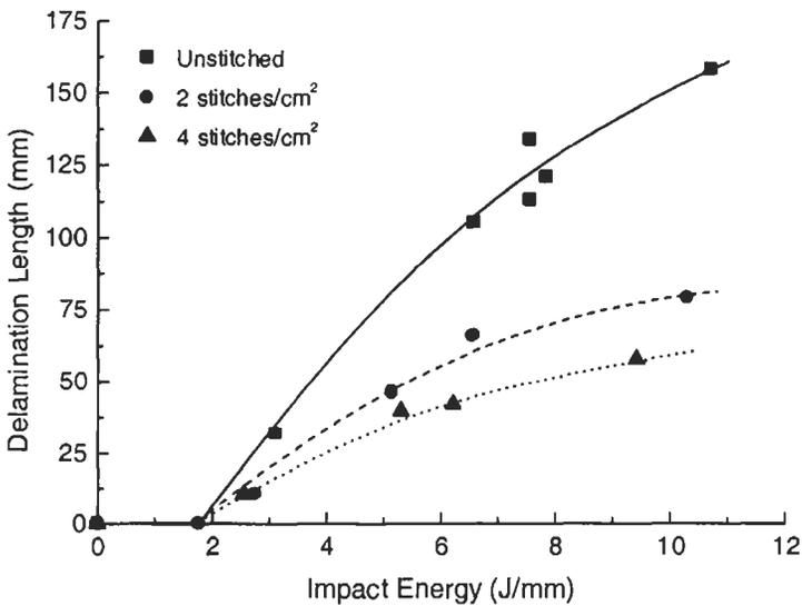
**Figure 8.31** Effect of low energy impact loading on the amount of delamination damage caused to stitched and unstitched composites (Data from Wu and Liao, 1995).
