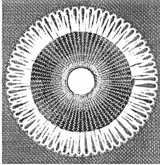
**Figure 2.34** Example of a fibre oriented reinforcement manufactured via technical embroidery (courtesy of Hightex GmbH)
