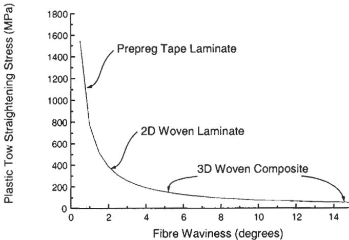
**Figure 5.10** Effect of in-plane tow waviness on the tensile stress for plastic tow straightening. Representative tow straightening stresses for 2D and 3D woven composites are indicated. The comparison is made for composites with identical fibre content ( $f_s = 0.3$ ) and shear strength ( $|\tau_{13}| = 45$  MPa) values.
