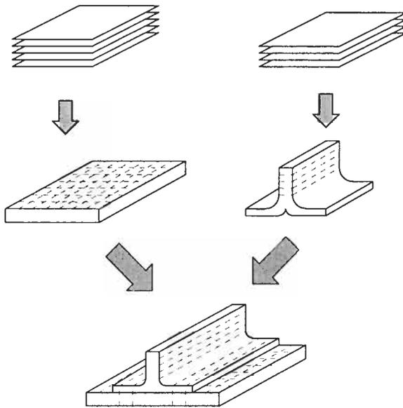
**Figure 2.33** Illustration of complex preform manufacture via stitching
