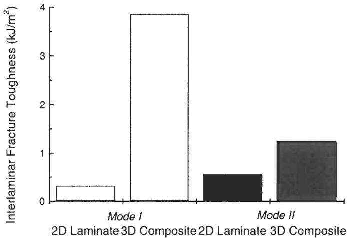
**Figure 5.24** Comparison of the delamination resistance of 2D and 3D composites for mode I and II loading (The modes I and II data is from Guénon et al. (1989) and Liu et al. (1989), respectively).
