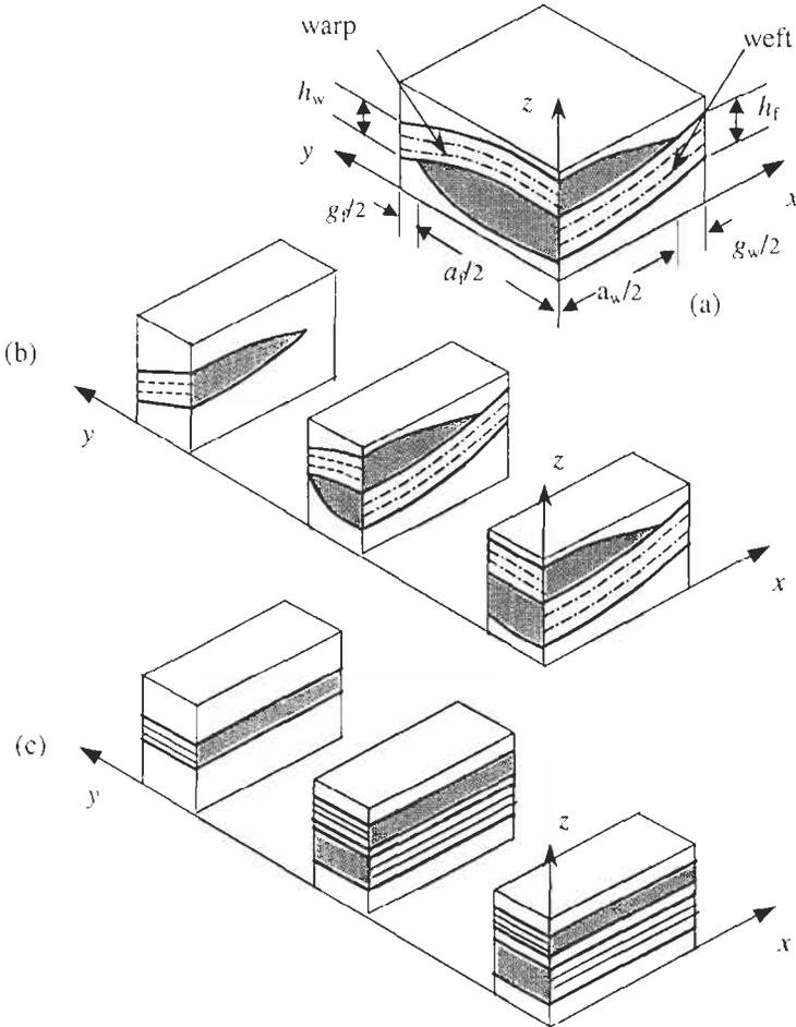
**Figure 4.7** Slice array model for unit cell of plain weave: (a) Unit cell of plain weave lamina, (b) actual slices along  $y$  coordinate of the unit cell, (c) idealised slices for the actual slices (Naik and Ganesh, 1992)
