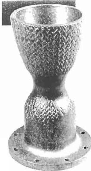
**Figure 1.4** 3D braided preform for a rocket nozzle (Courtesy of the Atlantic Research Corporation)
