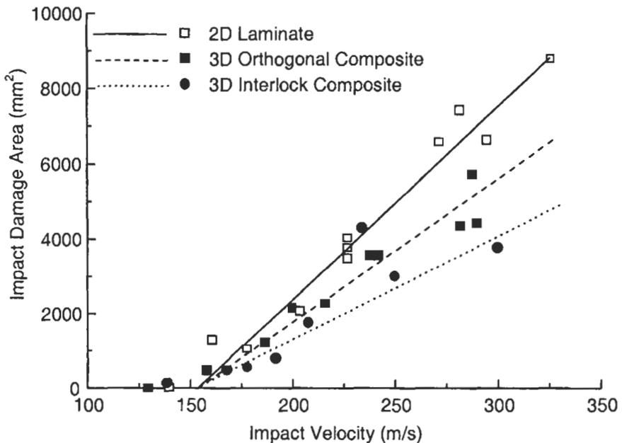
**Figure 5.25** Effect of impact velocity on the amount of delamination damage to 2D and 3D woven composites (Data from Billaut and Rousell, 1995).
