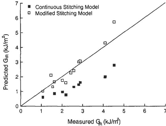
**Figure 8.24** Plot of measured against theoretical  $G_{IR}$  values for stitched composites. The theoretical  $G_{IR}$  values were determined using the modified and continuous stitching models by Jain and Mai. The closer the data points are to the straight line the better the agreement between the measured and theoretical  $G_{IR}$  value (Adapted from Mouritz and Jain, 1999).
