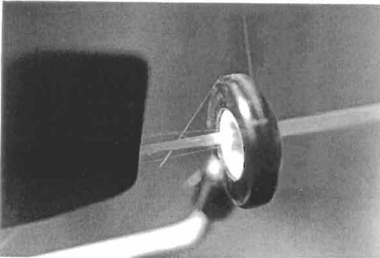
**Figure 5.1** Broken fibres caused by 3D weaving.
