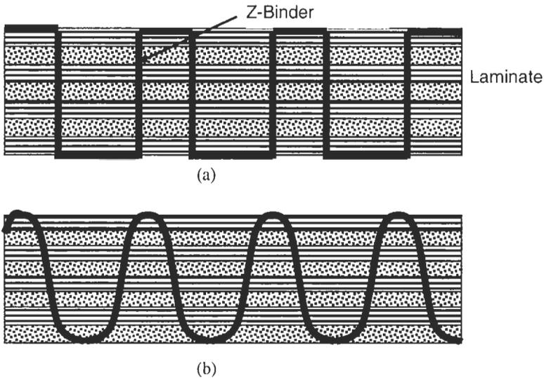
**Figure 5.5** (a) Idealised and (b) actual profiles of a z-binder yarn in a 3D orthogonal composite. The z-binder is supposed to have a square-wave profile, but in reality can be distorted into a quasi-sinusoidal profile.
