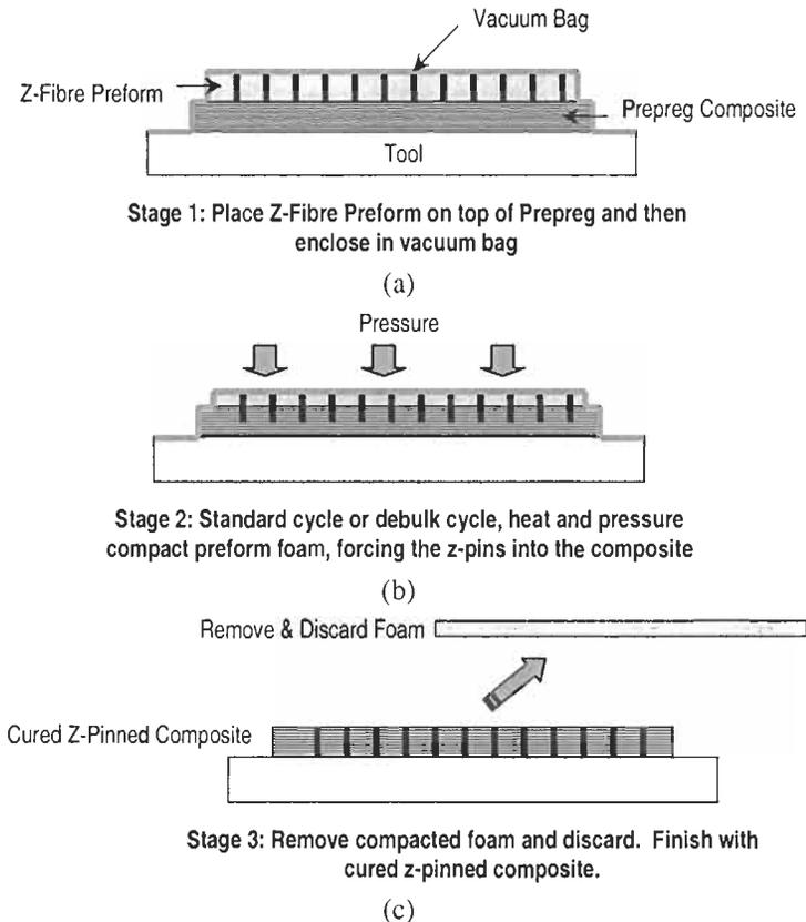
**Figure 9.2** Schematic of the Z-fiber™ insertion process using an autoclave (Adapted from Freitas et al., 1994)
