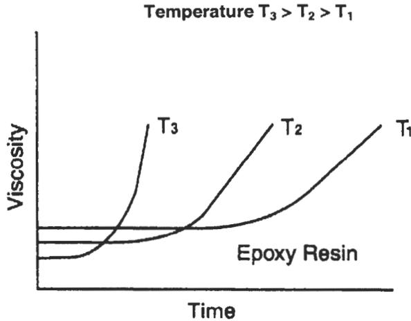
**Figure 3.5** Illustration of resin viscosity versus time
