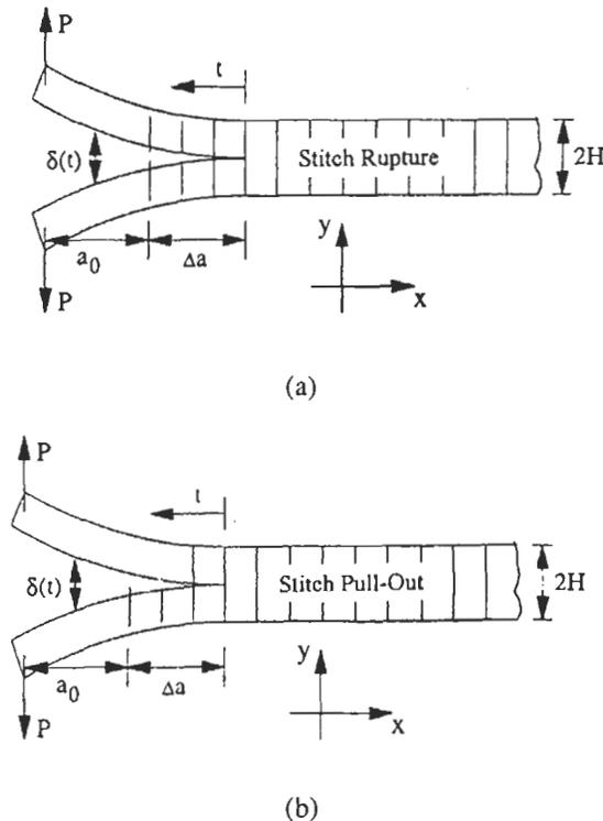
**Figure 8.22** The DCB specimen geometry used as the basis for the Jain and Mai model for mode I interlaminar fracture toughness of stitched composites. Models have been developed for the cases where the stitches (a) rupture along the delamination crack path (continuous stitching model) and (b) failure at the surface and then pull-out from the composite (discontinuous stitching model) (From Jain and Mai, 1997).
