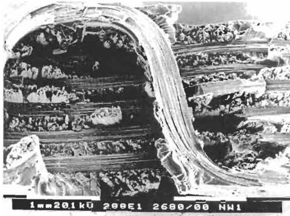
(c) Micrograph of the fracture surface for a CFRP specimen loaded in filler direction
