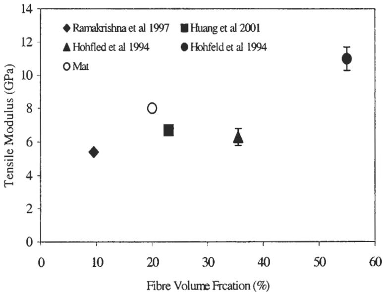
**Figure 7.4** Variation in tensile modulus of E-glass/epoxy, plain knit composites with fibre volume fraction
