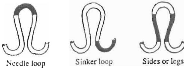
**Figure 7.2** Illustration of the main segments in a knit loop
