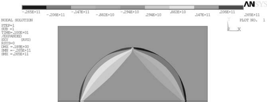
Figure 2.82. Shear stresses in the homogenisation problem \chi^{12}
