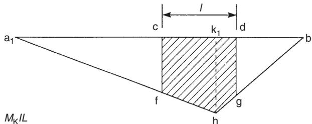
**FIGURE 20.8** Load position for maximum bending moment at K
