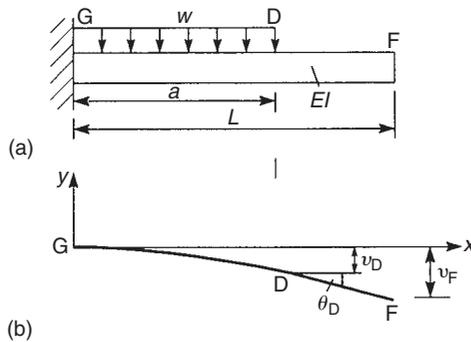
**FIGURE 13.4** Cantilever beam of Ex. 13.3
