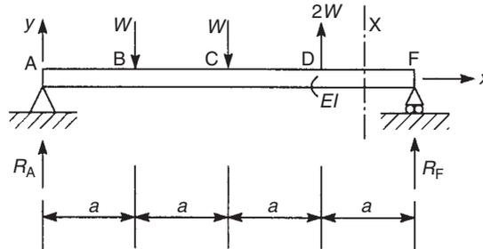
**FIGURE 13.9** Macauley's method for the deflection of a simply supported beam (Ex. 13.8)
