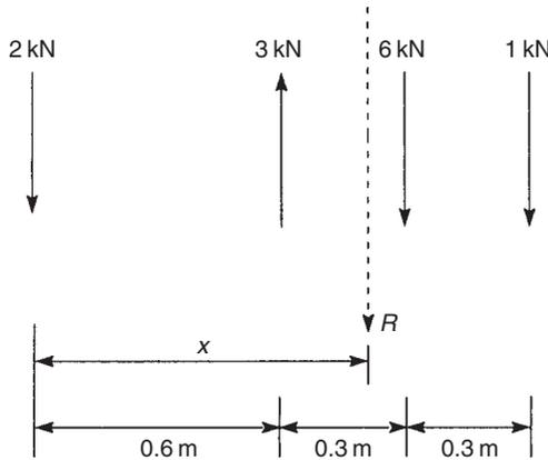
FIGURE 2.18 Force system of Ex. 2.1
