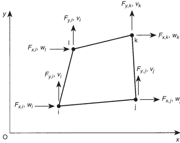
FIGURE 17.14 Quadrilateral element subjected to nodal in-plane forces and displacements
