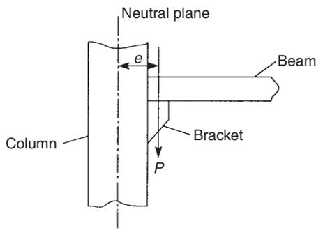
FIGURE 9.8 Combined bending and axial load on a column
