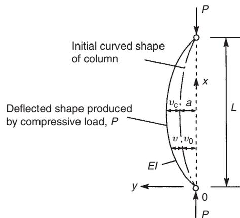
FIGURE 21.10 Failure of an initially curved column
