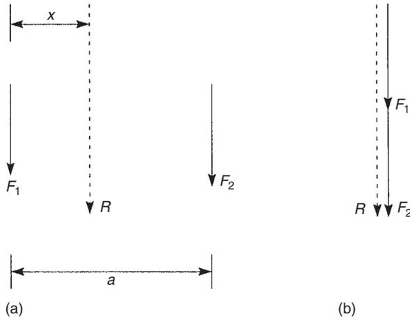
**FIGURE 2.17** Resultant of a system of parallel forces
