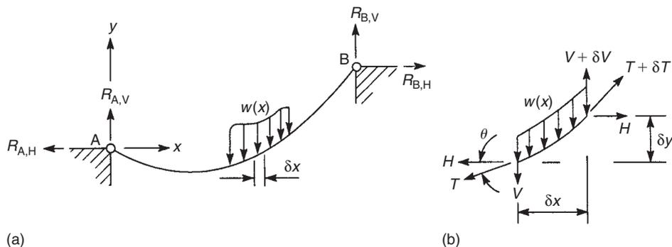
FIGURE 5.4 Cable subjected to a distributed load
