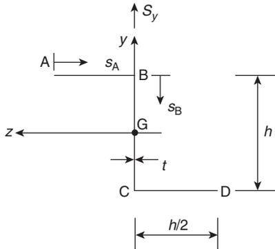
FIGURE 10.13 Beam section of Ex. 10.4
