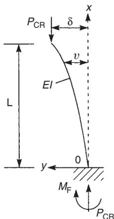
FIGURE 21.6 Determination of buckling load for a column with one end fixed and one end free
