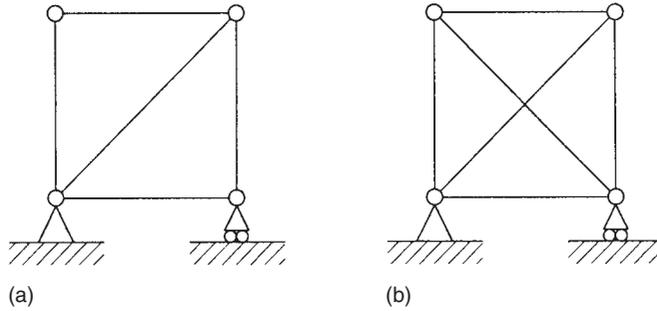
the members whereas the truss shown in Fig. 1.17(b) is statically determinate only as far as the calculation of support reactions is concerned.
