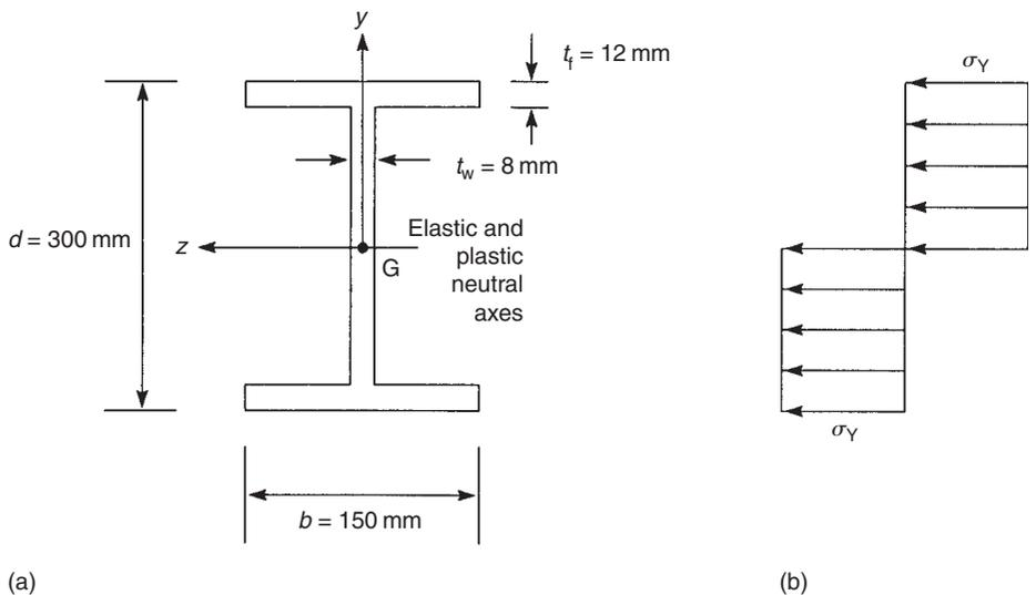
FIGURE 18.5 Beam section of Ex. 18.2 (a)
