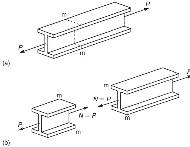
FIGURE 7.1 Structural member with axial load
