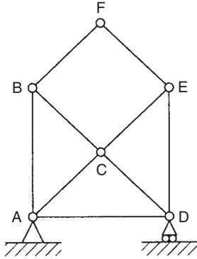
FIGURE 4.9 Investigation into truss stability
