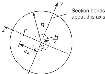
FIGURE 9.12 Core of a circular section beam
