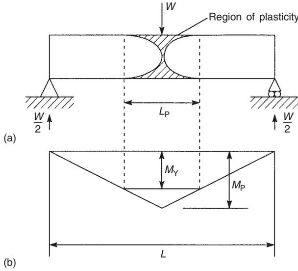
FIGURE 18.9 Formation of a plastic hinge in a simply supported beam
