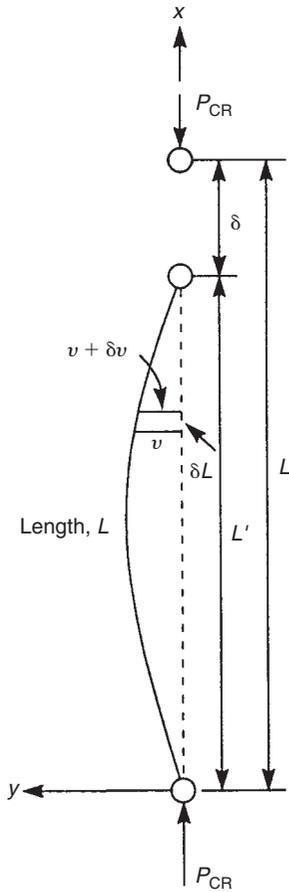
FIGURE 21.16 Shortening of a column due to buckling
