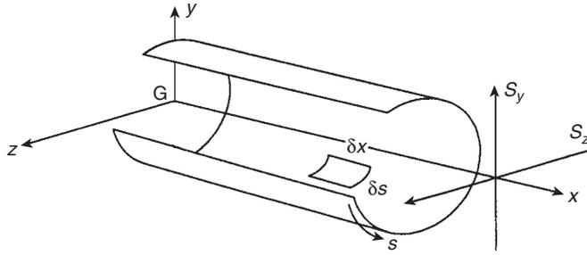
FIGURE 10.11 Shear of a thin-walled open section beam
