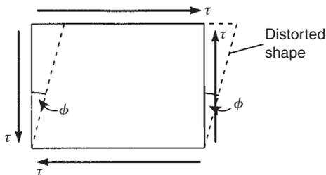
FIGURE 7.6 Shear strain in an element
