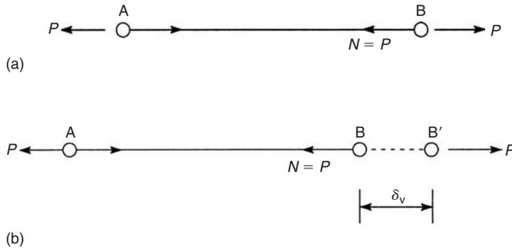
**FIGURE 15.6** Sign of the internal virtual work in an axially loaded member
