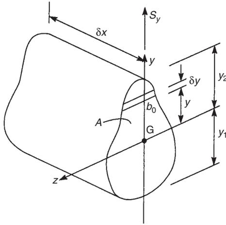
FIGURE 13.20 Determination of form factor  $\beta$
