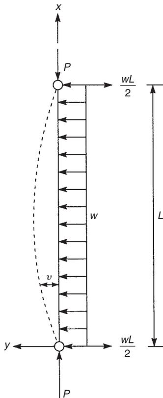
FIGURE 21.13 Bending of a uniformly loaded beam-column
