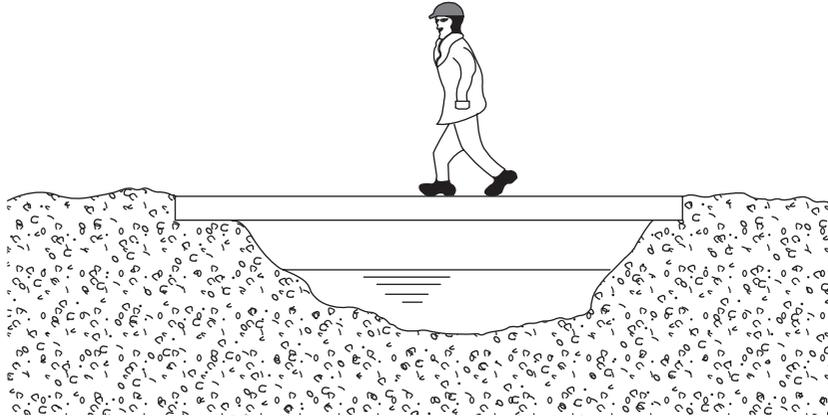
FIGURE 1.1 Beam as a simple bridge
