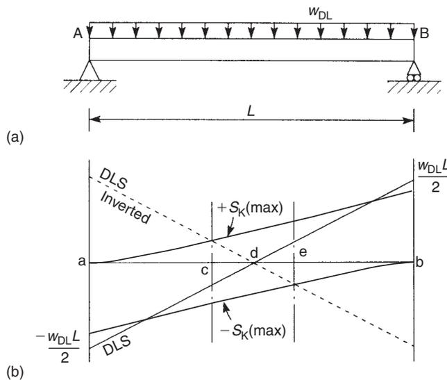
FIGURE 20.11 Reversal of shear force in a beam
