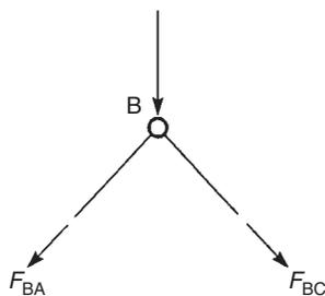
FIGURE 4.5 Joint equilibrium in a triangular structure
