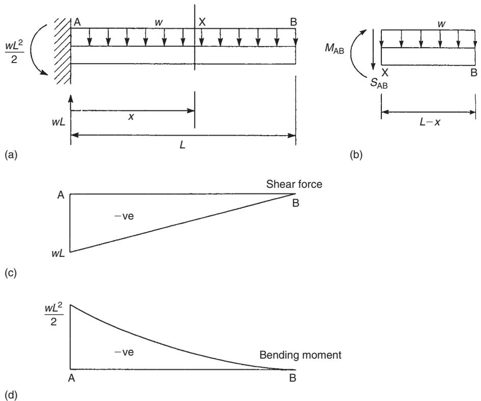
**FIGURE 3.12** Shear force and bending moment diagrams for the beam of Ex. 3.5
