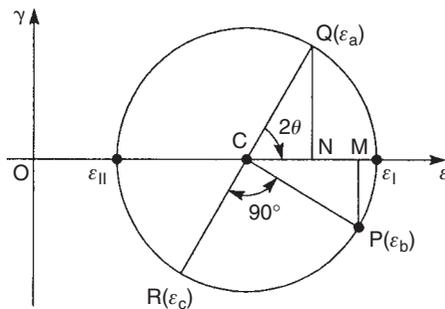
**FIGURE 14.17** Mohr's circle of strain for a 45° strain gauge rosette
