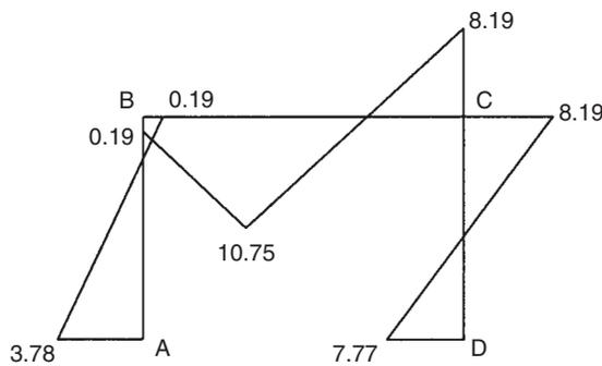
**FIGURE 16.48** Bending moment diagram for the portal frame of Ex. 16.22. Bending moments (kNm) drawn on tension side of members
