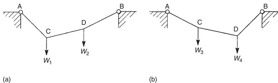
FIGURE 5.2 Effect on cable geometry of load variation
