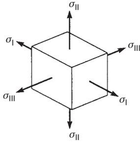
**FIGURE 14.18** Reduction of a complex three-dimensional stress system
