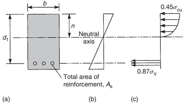
**FIGURE 12.10** Stress and strain distributions in a reinforced concrete beam
