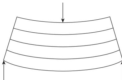
we have noted this earlier in Section 7.3 where we saw that shear stresses applied in one plane induce equal complementary shear stresses on perpendicular planes which is exactly the same situation as in the connected planks. This is important in the design of the connections between, say, a concrete slab and the flange of a steel I-section beam where the connections, usually steel studs, are subjected to this horizontal shear.
