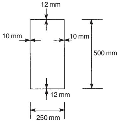
FIGURE 14.22 Box girder beam section of Ex. 14.8
