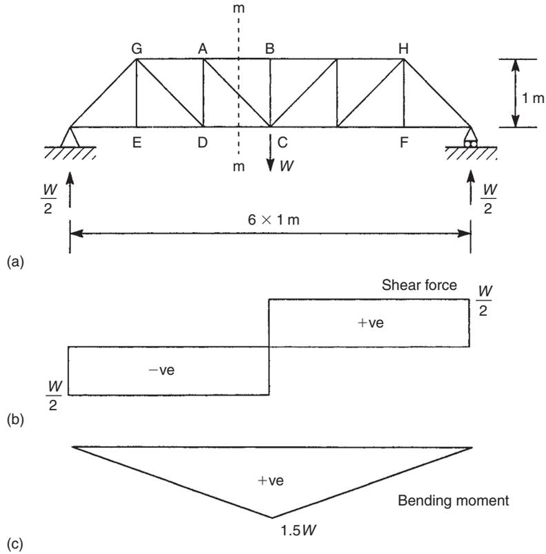
FIGURE 4.10 Shear forces and bending moments in a truss
