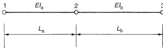
accomplished by merely specifying nodes at points along the beam such that any element lying between adjacent nodes carries, at the most, a uniform shear and a linearly varying bending moment. For example, the beam of Fig. 17.7 would be idealized into beam-elements 1–2, 2–3 and 3–4 for which the unknown nodal displacements are  $v_2$ ,  $\theta_2$ ,  $\theta_3$ ,  $v_4$  and  $\theta_4$  ( $v_1 = \theta_1 = v_3 = 0$ ).
