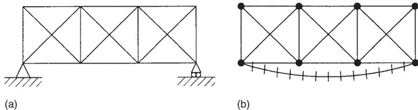
The completely stiff structure is shown in Fig. 16.11(b) in which we see that  $M = 17$  and  $N = 8$ . However, since the truss is pin-jointed, we can obtain the internal statical indeterminacy directly from Eq. (16.5) in which  $M = 16$ , the actual number of truss members. Thus
