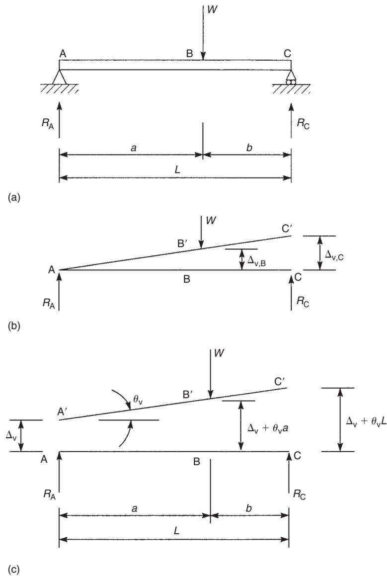
**FIGURE 15.4** Use of the principle of virtual work to calculate support reactions
