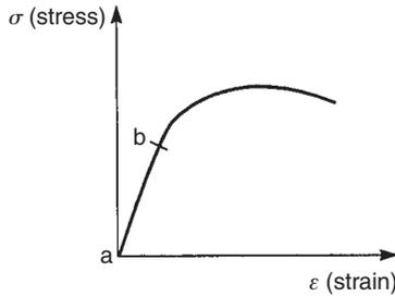
FIGURE 7.8 Typical stress–strain curve
