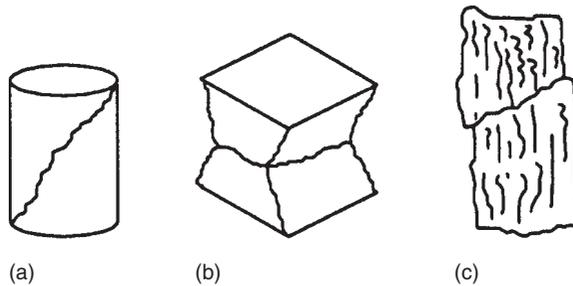
**FIGURE 8.15** Failure of brittle materials
