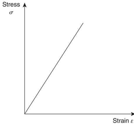
**FIGURE 8.16** Stress–strain curve for a fibre composite
