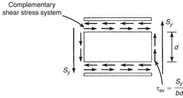
**FIGURE 12.5** Shear stresses between steel plates and timber beam (side view of a length of beam)
