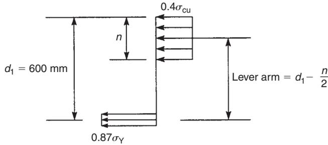
FIGURE 12.12 Stress distribution in beam of Ex. 12.7
