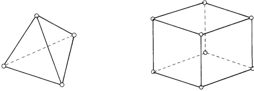
in  $x$ ,  $y$  and  $z$ ; for the tetrahedron the displacement function is of the first degree with 12 constant coefficients, while that for the prism may be of a higher order to accommodate the 24 degrees of freedom. A development in the solution of three-dimensional problems has been the introduction of curvilinear coordinates. This enables the tetrahedron and prism to be distorted into arbitrary shapes that are better suited for fitting actual boundaries.
