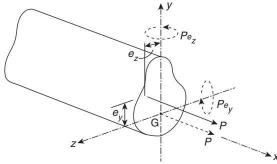
**FIGURE 9.9** Combined bending and axial load on a beam section
