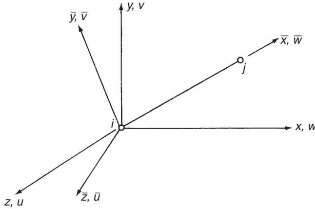
FIGURE 17.5 Local and global coordinate systems for a member in a space truss
