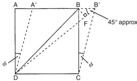
FIGURE 7.13 Distortion due to shear in element
