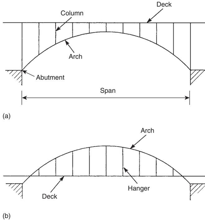
**FIGURE 1.6** Arches as bridge deck supports
