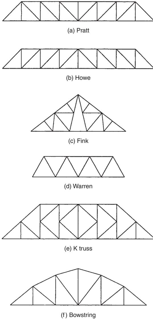
FIGURE 4.1 Types of plane truss
