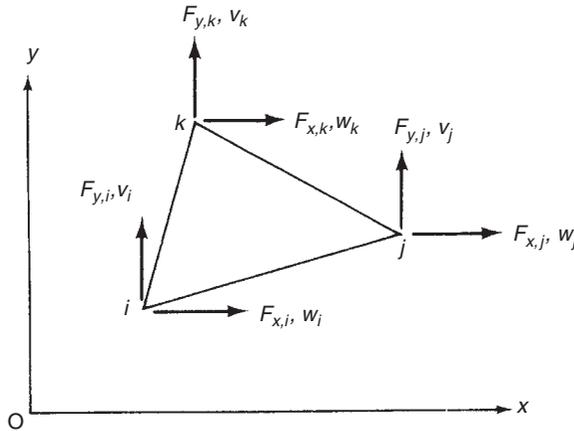
**FIGURE 17.13** Triangular element for plane elasticity problems
