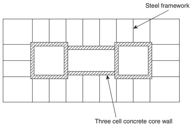
FIGURE 1.10 Sectional plan of core wall and steel structure
