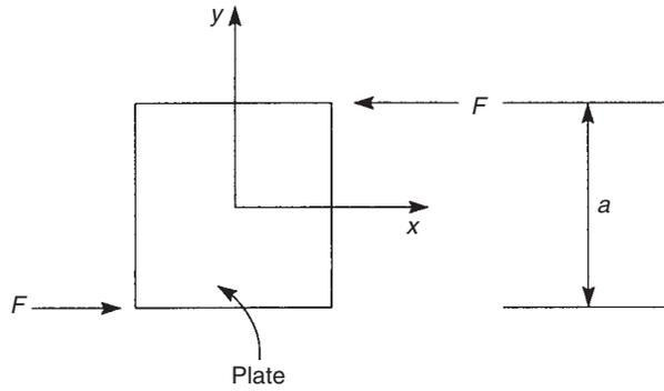
**FIGURE 2.19** Couple produced by out-of-line forces
