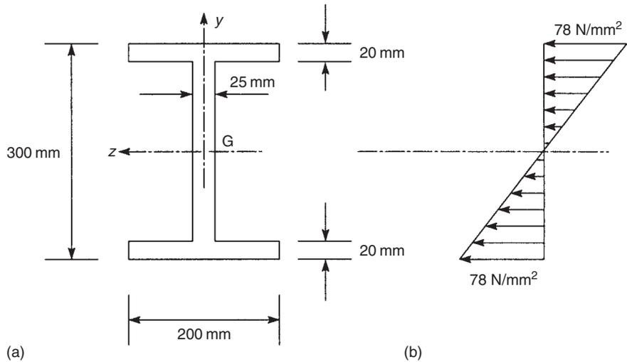
**FIGURE 9.6** Direct stress distribution in beam of Ex. 9.2
