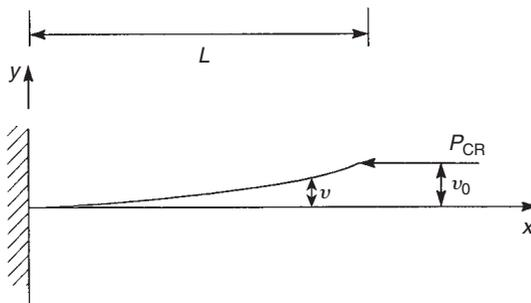
**FIGURE 21.17** Buckling load for a built-in column by the energy method
