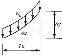
FIGURE 5.5 Elemental length of cable under its own weight
