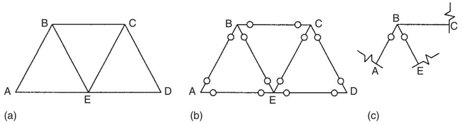
so that if  $r$  is the total number of releases required, the degree of static indeterminacy,  $n_s$ , of the actual structure is
