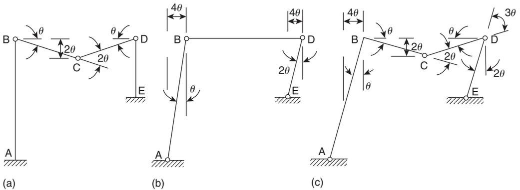
FIGURE 18.17 Collapse mechanisms for the frame of Ex. 18.8
