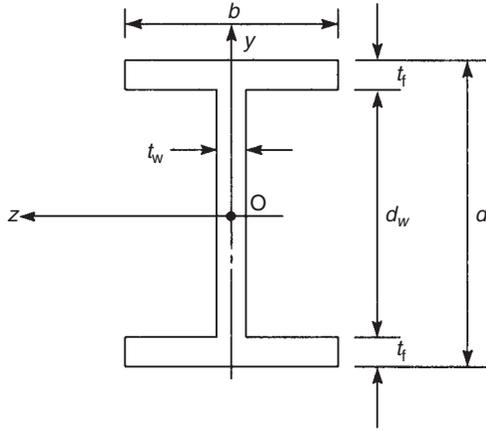
**FIGURE 9.22** Second moments of area of an I-section
