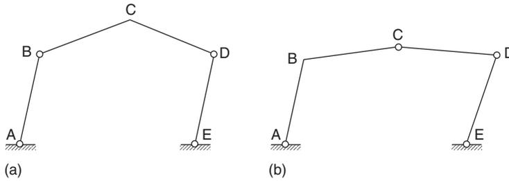
failure mechanisms would have to be investigated; two such mechanisms are shown in Fig. 18.22. Note that in Fig. 18.22(a) there is a hinge cancellation at C and in Fig. 18.22(b) there is a hinge cancellation at B. In determining the collapse loads of such frames the method of instantaneous centres still applies.
