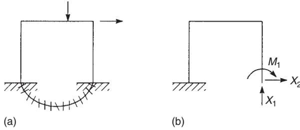
FIGURE 16.23 Indeterminacy of a portal frame
