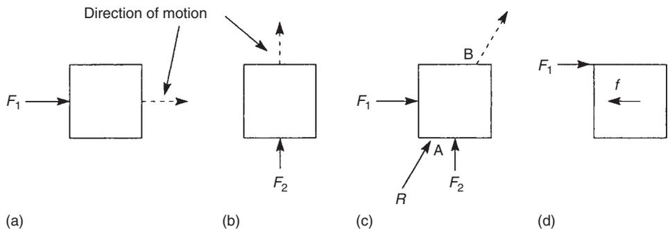
is applied as shown in Fig. 2.2(b) the cube will move in the direction of  $F_2$ . It follows that if  $F_1$  and  $F_2$  were applied simultaneously, the cube would move in some inclined direction as though it were acted on by a single inclined force  $R$  (Fig. 2.2(c));  $R$  is called the *resultant* of  $F_1$  and  $F_2$ .
