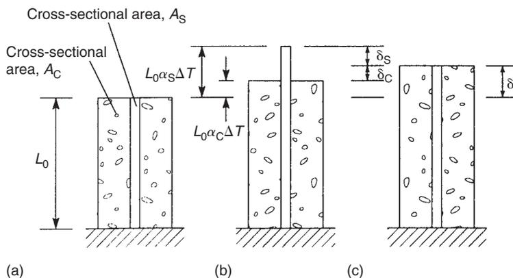
Suppose now that expansion is completely prevented so that the final length of the member after the temperature rise is still  $L_0$ . The member has, in effect, been compressed by an amount  $L_0\alpha\Delta T$ , thereby producing a compressive strain,  $\epsilon$ , which is given by (see Eq. (7.4))
