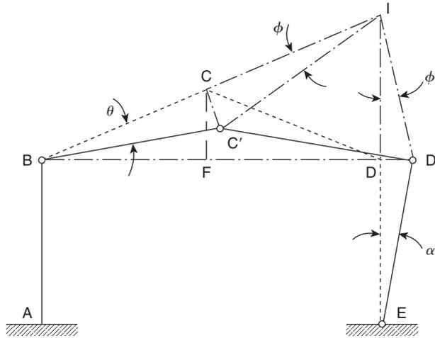
FIGURE 18.21 Method of instantaneous centres for the frame of Ex. 18.10
