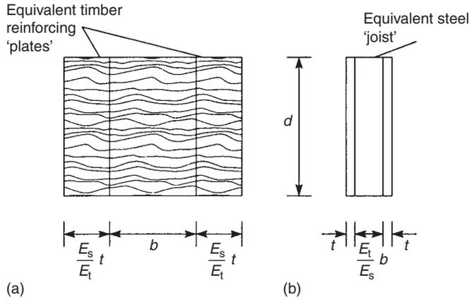
FIGURE 12.2 Equivalent beam sections
