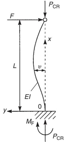
FIGURE 21.7 Determination of buckling load for a column with one end fixed and the other end pinned
