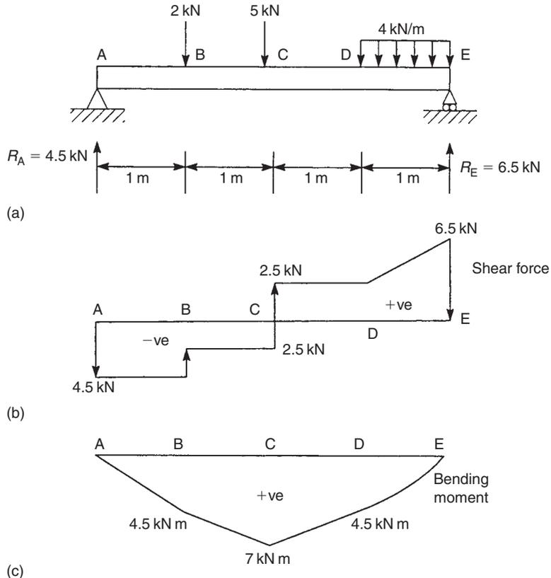
**FIGURE 3.19** Shear force and bending moment diagrams for the beam of Ex. 3.10
