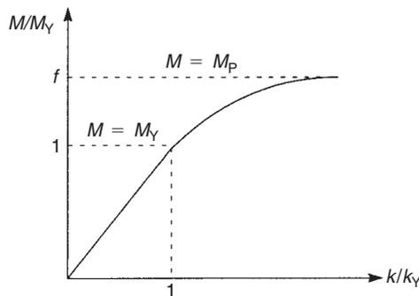
FIGURE 18.7 Moment–curvature diagram for a beam
