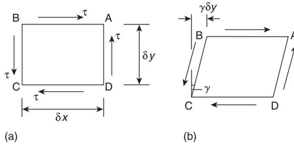
FIGURE 10.9 Determination of strain energy due to shear
