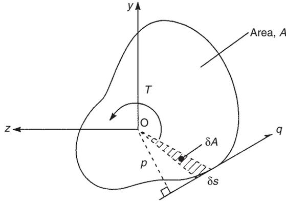
**FIGURE 11.12** Torque–shear flow relationship in a thin-walled closed section beam
