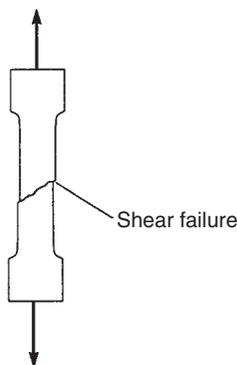
FIGURE 14.3 Mode of failure in an aluminium alloy test piece
