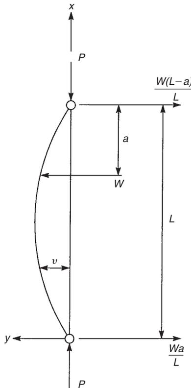
**FIGURE 21.14** Beam-column supporting a point load
