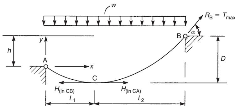
FIGURE 5.7 Cable carrying a uniform horizontally distributed load
