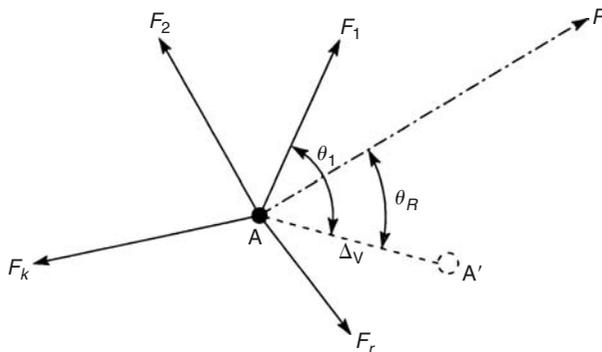
FIGURE 15.2 Virtual work for a system of forces acting on a particle
