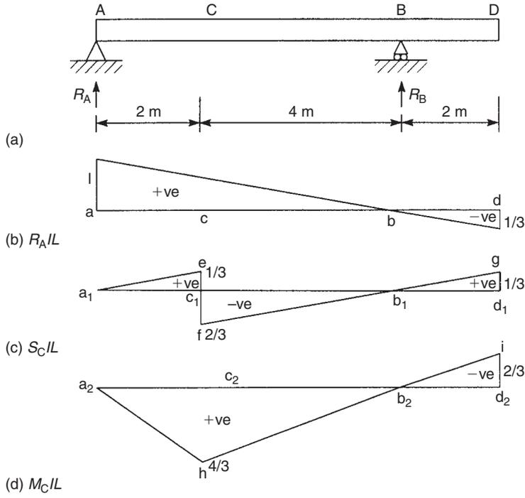
FIGURE 20.2 Shear force and bending moment influence lines for the beam of Ex. 20.1
