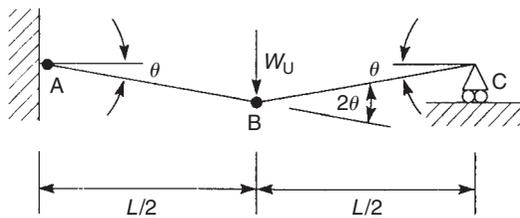
FIGURE 18.12 Virtual displacements in propped cantilever of Fig. 18.11
