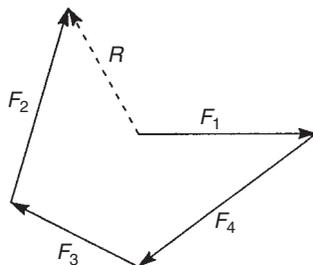
FIGURE 2.7 Alternative construction of force diagram for system of Fig. 2.6(a)
