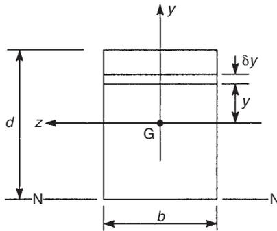
FIGURE 9.21 Second moments of area of a rectangular section
