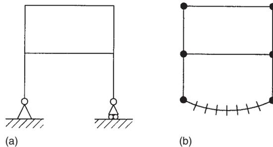
In the completely stiff structure shown in Fig. 16.12(b),  $M = 7$  and  $N = 6$ . The number of releases,  $r$ , required to return the completely stiff structure to its original state is 3. Thus, from Eq. (16.3)
