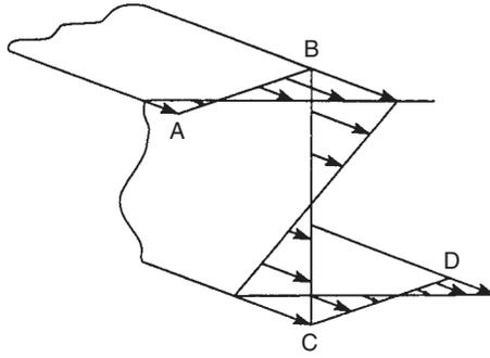
FIGURE 9.28 Distribution of direct stress in beam section of Ex. 9.10
