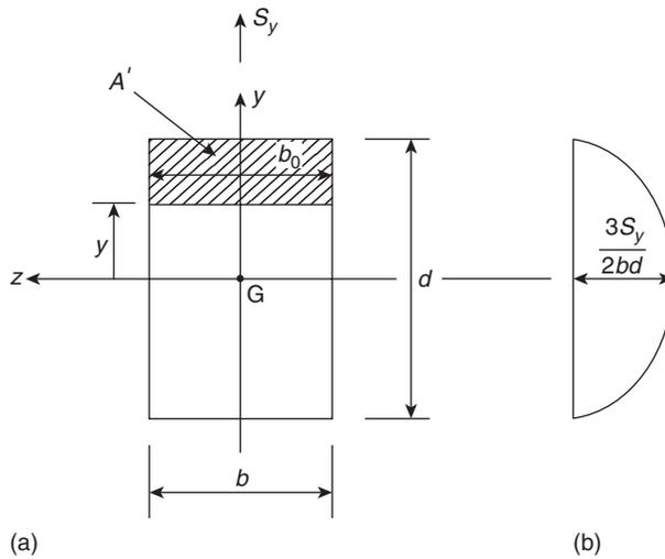
**FIGURE 10.5** Shear stress distribution in a rectangular section beam
