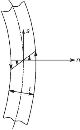
**FIGURE 11.15** Shear stress distribution due to torsion in a thin-walled open section beam
