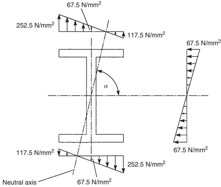
FIGURE 9.7 Direct stress distribution in beam of Ex. 9.4
