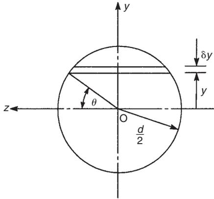
**FIGURE 9.23** Second moments of area of a circular section
