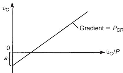
**FIGURE 21.11** Experimental determination of the buckling load of a column from a Southwell plot
