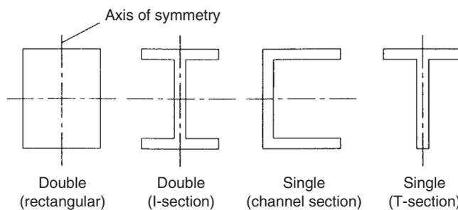
FIGURE 9.2 Symmetrical section beams
