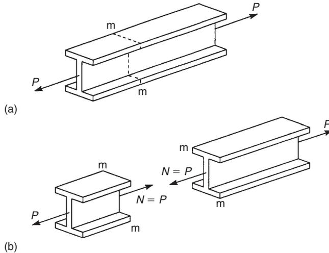
FIGURE 7.1 Structural member with axial load
