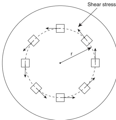
**FIGURE 11.3** Shear stresses produced by a pure torque
