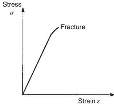
**FIGURE 8.14** Stress–strain curve for a brittle material
