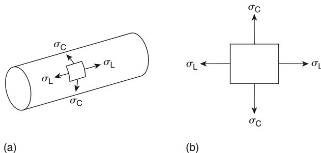
FIGURE 7.25 Two-dimensional stress system
