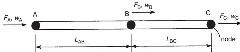
FIGURE 17.2 Two axially loaded members in line
