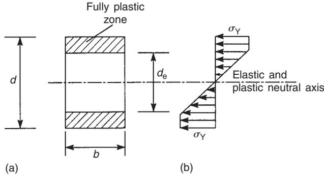
**FIGURE 18.8** Plastic bending of a rectangular-section beam
