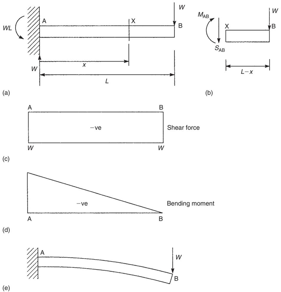
**FIGURE 3.11** Shear force and bending moment diagrams for the beam of Ex. 3.4
