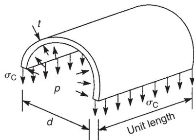
FIGURE 7.24 Circumferential stress due to internal pressure
