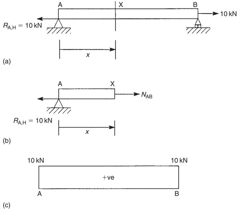
FIGURE 3.8 Normal force diagram for the beam of Ex. 3.1
