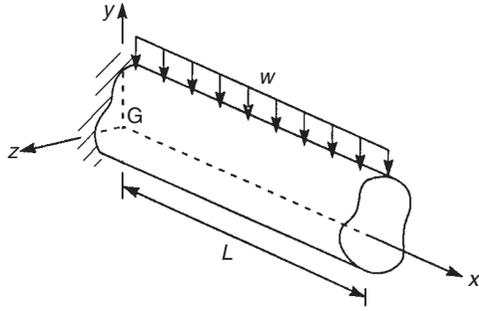
**FIGURE 13.19** Deflection of a cantilever of unsymmetrical cross section carrying a uniformly distributed load (Ex. 13.16)
