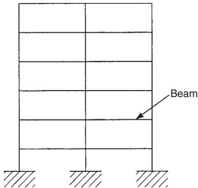
FIGURE 1.2 Beam as a structural element
