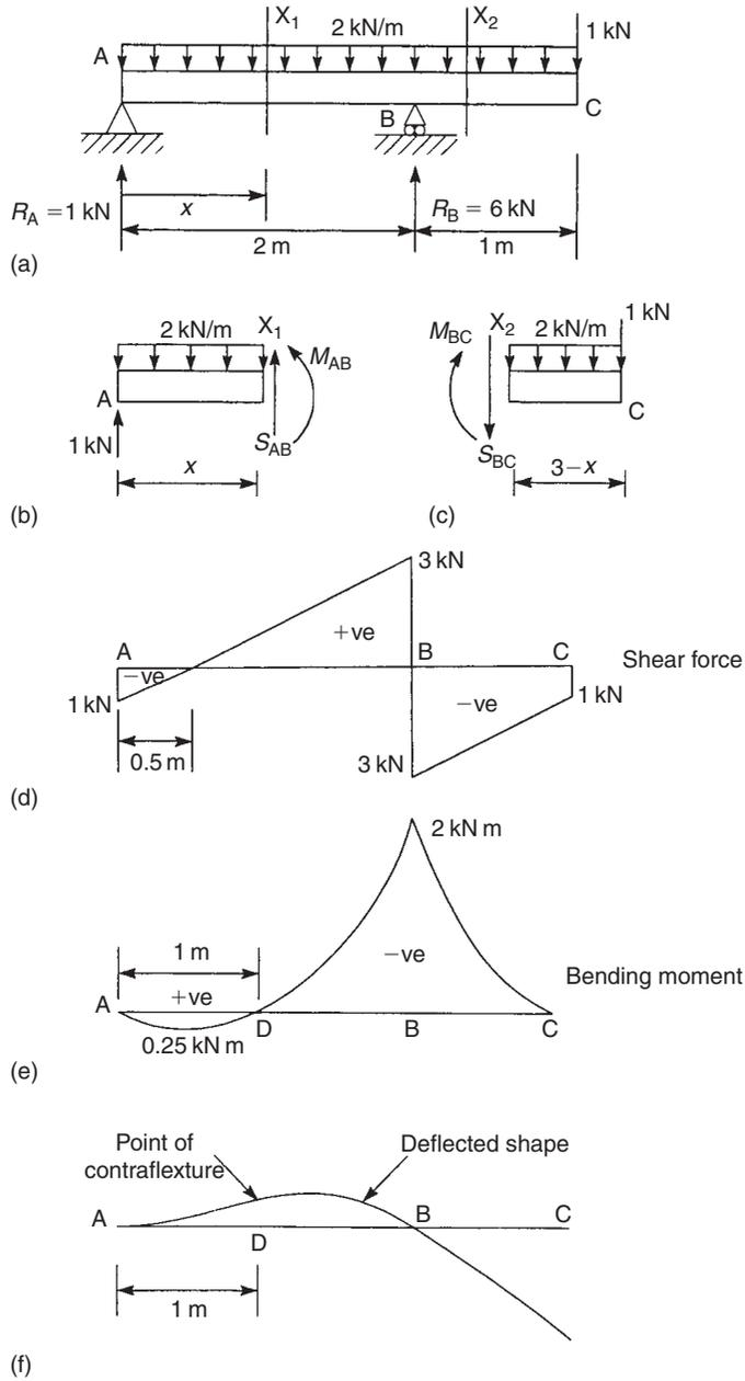
**FIGURE 3.16** Shear force and bending moment diagrams for the beam of Ex. 3.8
