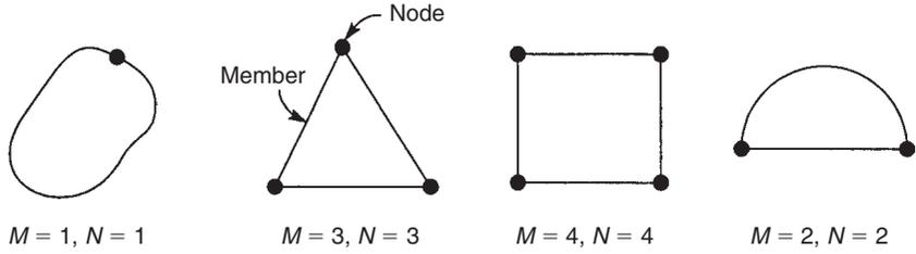
**FIGURE 16.4** Effect on members and nodes of cutting a ring
