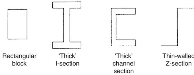
**FIGURE 11.13** Examples of solid beam sections
