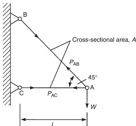
FIGURE 7.16 Deflection of a simple truss
