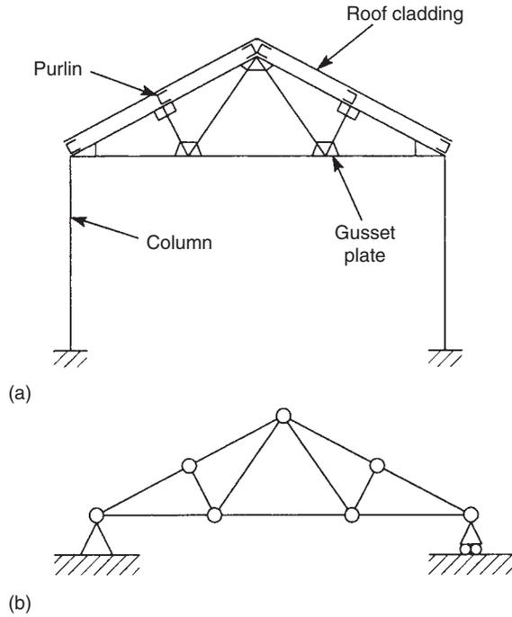
**FIGURE 1.18** (a) Actual truss and (b) idealized truss
