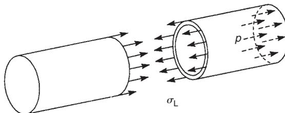
FIGURE 7.23 Longitudinal stresses due to internal pressure
