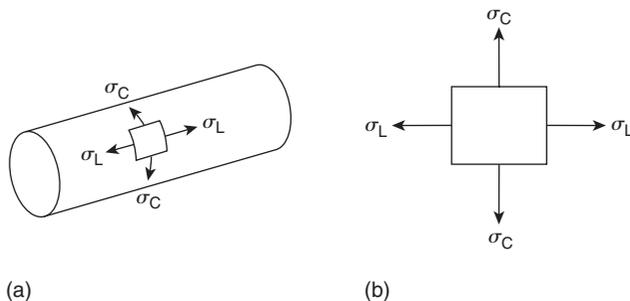
FIGURE 7.25 Two-dimensional stress system
