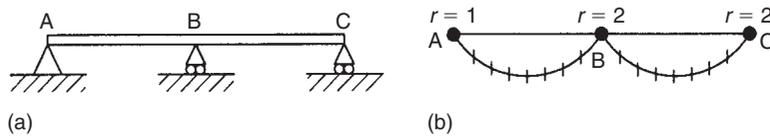
The completely stiff structure is shown in Fig. 16.10(b) where we see that  $M = 4$  and  $N = 3$ . The number of releases,  $r$ , required to return the completely stiff structure to its original state is 5, as indicated in Fig. 16.10(b); these comprise a moment release at each of the three supports and a translational release at each of the supports B and C. Therefore, from Eq. (16.3)
