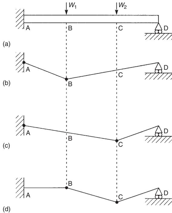
**FIGURE 18.13** Possible collapse mechanisms in a propped cantilever supporting two concentrated loads
