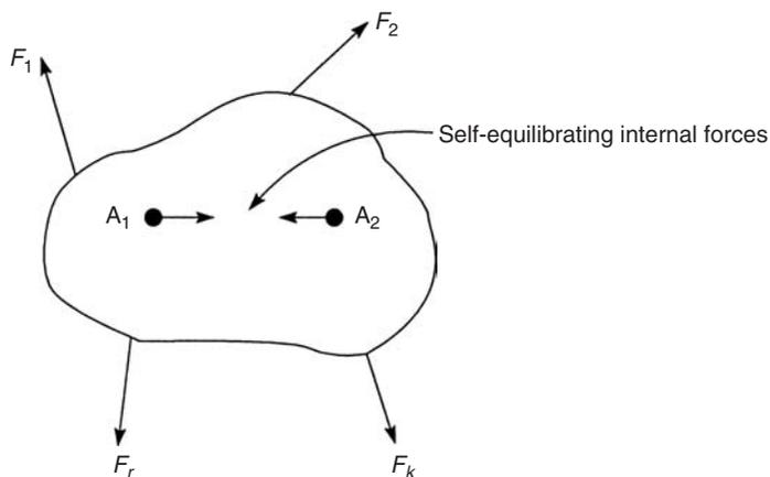
FIGURE 15.3 Virtual work for a rigid body
