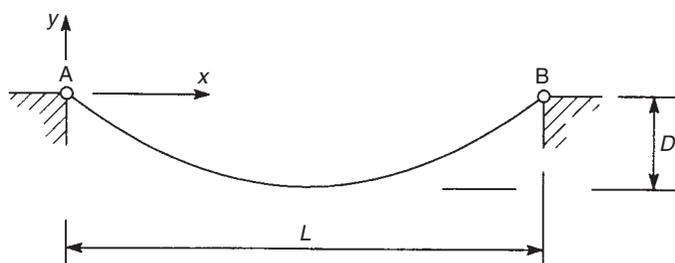
**FIGURE 5.6** Deflected shape of a symmetrically supported cable
