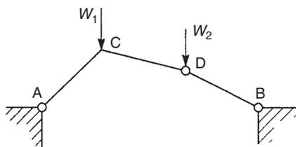
FIGURE 6.2 Linear three-pinned arch
