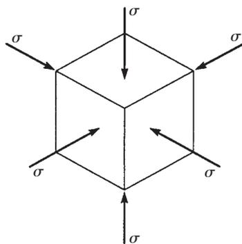
FIGURE 7.7 Cube subjected to hydrostatic pressure
