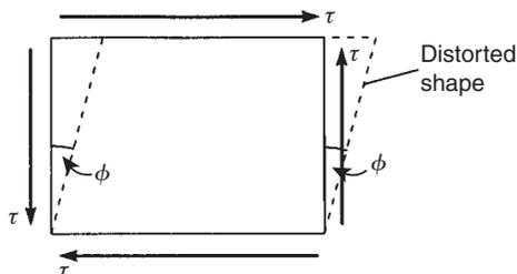
FIGURE 7.6 Shear strain in an element
