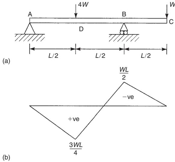
FIGURE 18.10 Beam of Ex. 18.5
