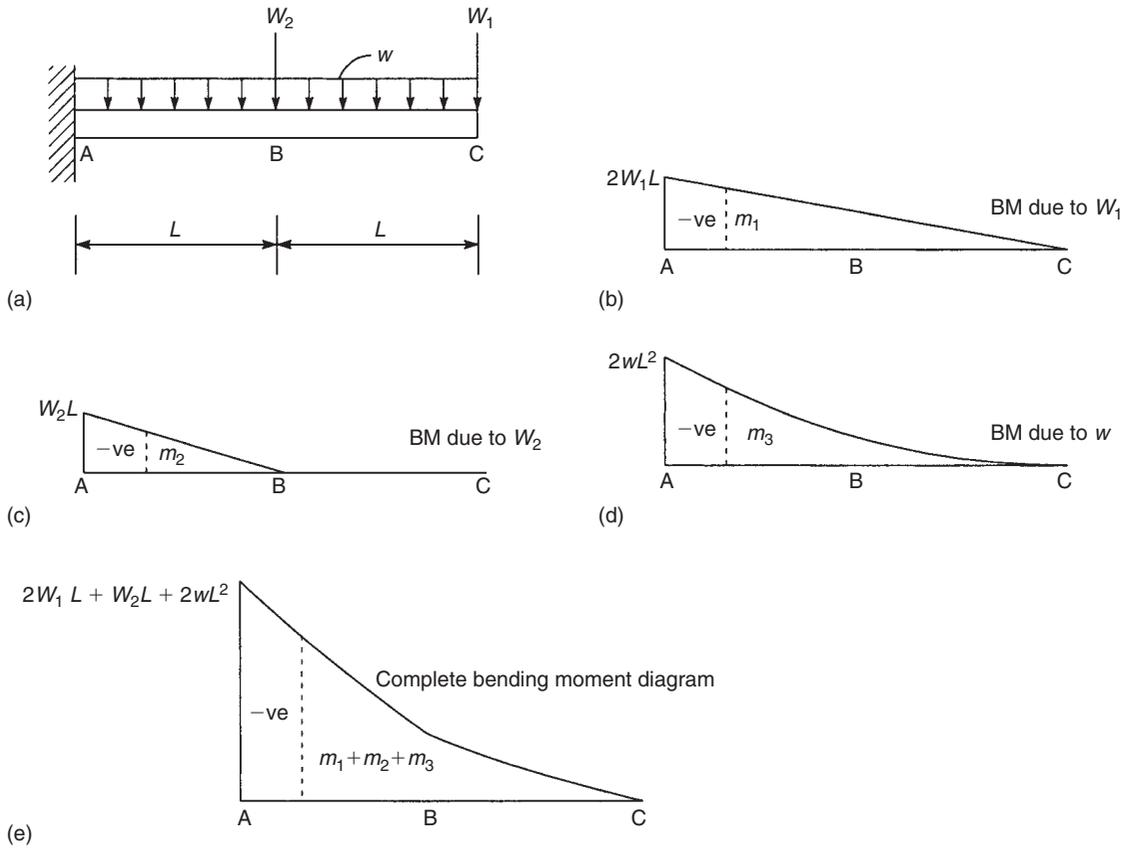
FIGURE 3.24 Bending moment (BM) diagram using the principle of superposition
