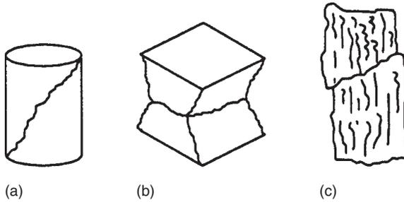
**FIGURE 8.15** Failure of brittle materials
