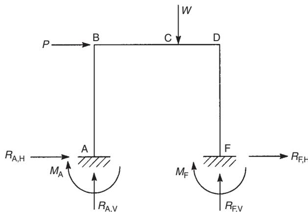
**FIGURE 16.1** Statical indeterminacy of a portal frame
