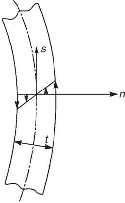
**FIGURE 11.15** Shear stress distribution due to torsion in a thin-walled open section beam
