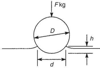
FIGURE 8.5 Brinell hardness test
