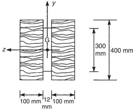
FIGURE 12.3 Steel-reinforced timber beam of Ex. 12.1
