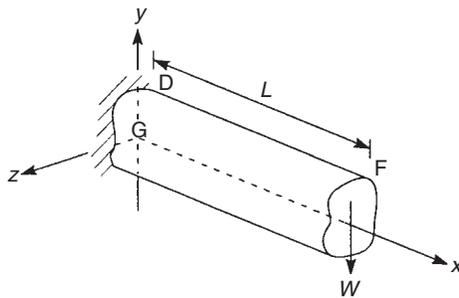
**FIGURE 13.18** Deflection of a cantilever of unsymmetrical cross section carrying a concentrated load at its free end (Ex. 13.15)
