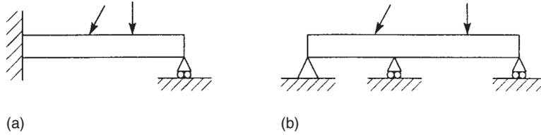
We shall now use the results of the previous work in this chapter to investigate methods of solving statically indeterminate beam systems. Having determined the reactions, diagrams of shear force and bending moment follow in the normal manner.
