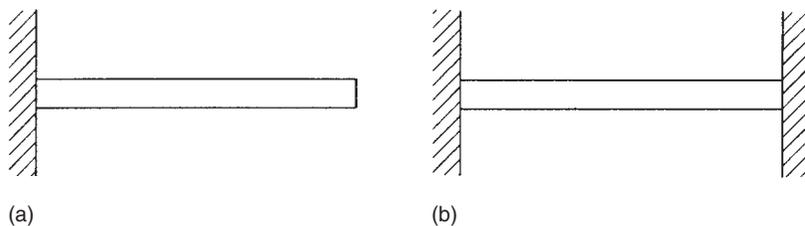
**FIGURE 1.15** (a) Cantilever beam and (b) fixed or built-in beam
