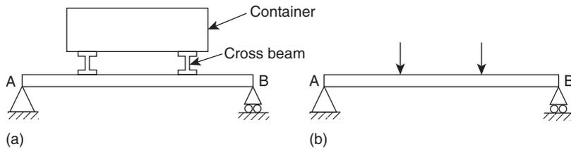
**FIGURE 1.19** Idealization of a load system
