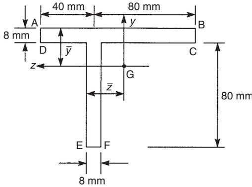
FIGURE 9.25 Beam section of Ex. 9.8
