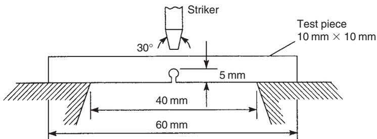
FIGURE 8.7 Charpy impact test
