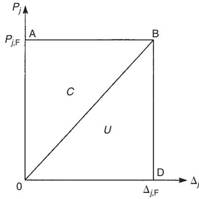
FIGURE 15.14 Load–deflection curve for a linearly elastic member
