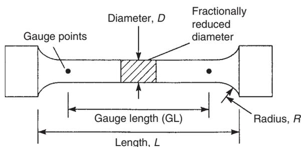
FIGURE 8.1 Standard cylindrical test piece
