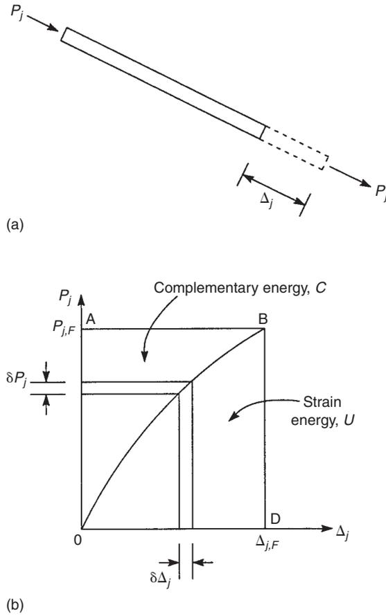
**FIGURE 15.13** Load–deflection curve for a non-linearly elastic member
