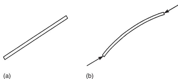
FIGURE 21.1 Buckling of a slender column
