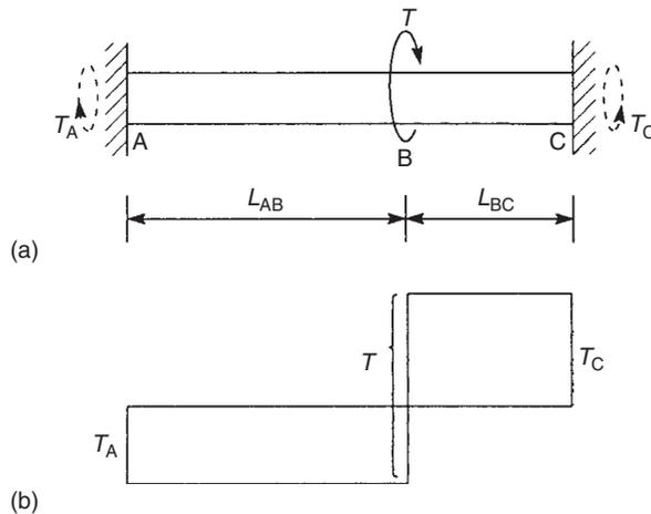
FIGURE 11.6 Torsion of a circular section bar with built-in ends
