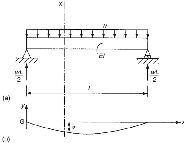
**FIGURE 13.5** Deflection of a simply supported beam carrying a uniformly distributed load (Ex. 13.4)
