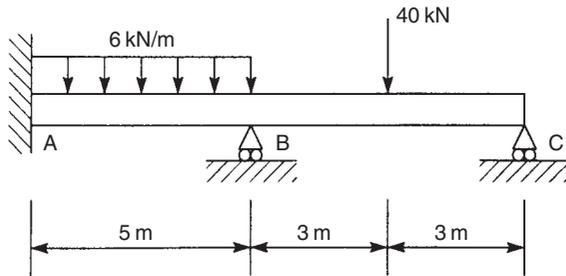
FIGURE 16.42 Beam of Ex. 16.20
