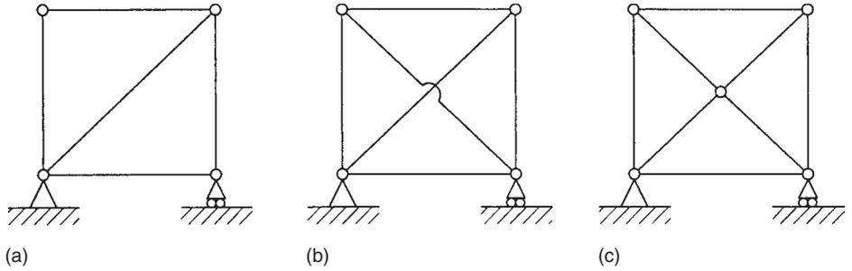
The truss in Fig. 4.7(c) comprises a series of triangular units which suggests that it is statically determinate. However, in this case,  $m = 8$  and  $j = 5$ . Thus
