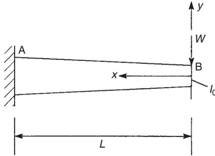
FIGURE 13.16 Deflection of a cantilever of tapering section
