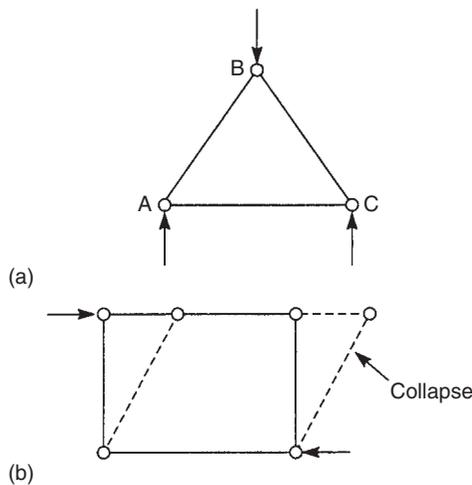
FIGURE 4.3 Basic unit of a truss
