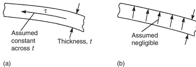
FIGURE 10.10 Assumptions in thin-walled open section beams
