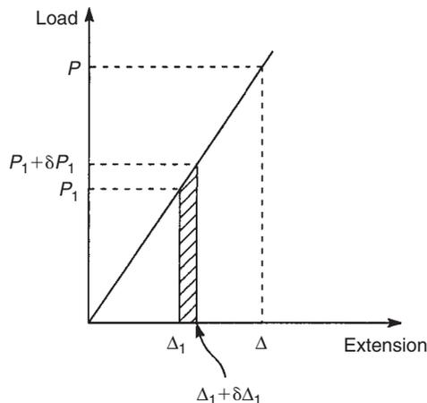
FIGURE 7.15 Work done by a gradually applied load
