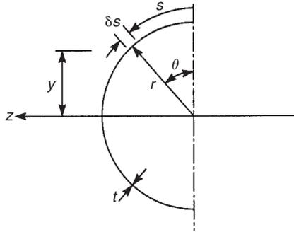
FIGURE 9.30 Second moment of area of a semicircular thin-walled section
