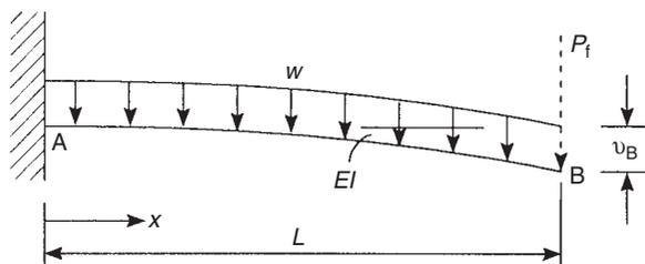
**FIGURE 15.17** Deflection of a cantilever beam using the dummy load method
