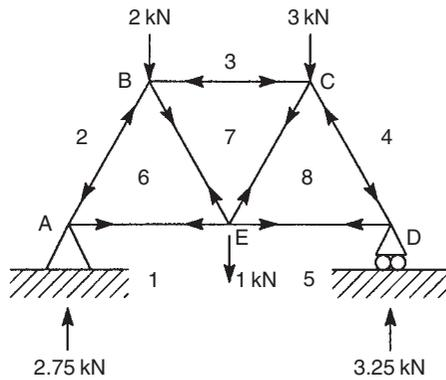
**FIGURE 4.21** Analysis of a truss by a graphical method
