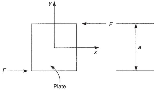
**FIGURE 2.19** Couple produced by out-of-line forces
