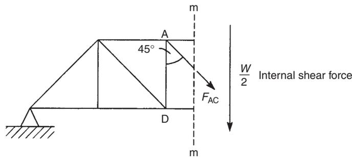
**FIGURE 4.11** Internal shear force in a truss
