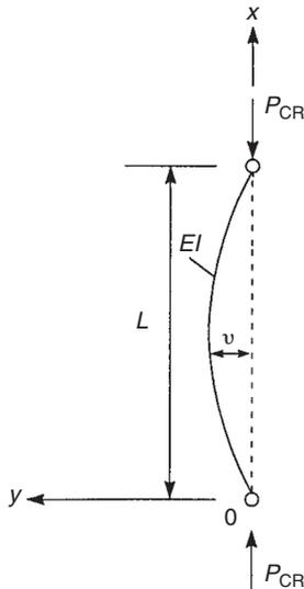
FIGURE 21.3 Determination of buckling load for a pin-ended column
