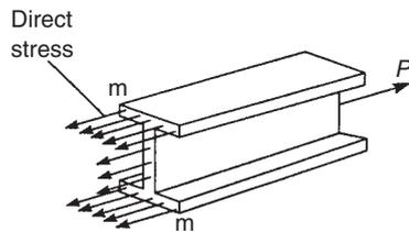
FIGURE 7.2 Internal force distribution in a beam section
