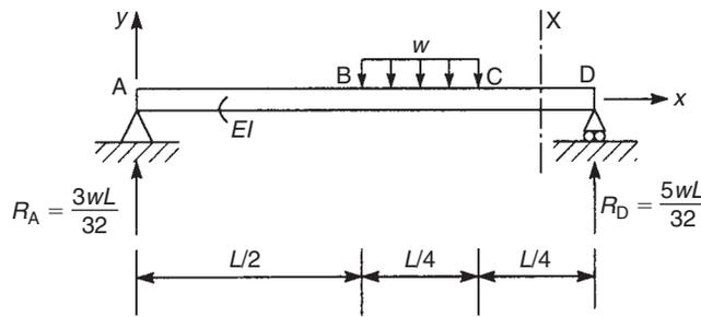
**FIGURE 13.10** Deflection of a beam carrying a part span uniformly distributed load (Ex. 13.9)
