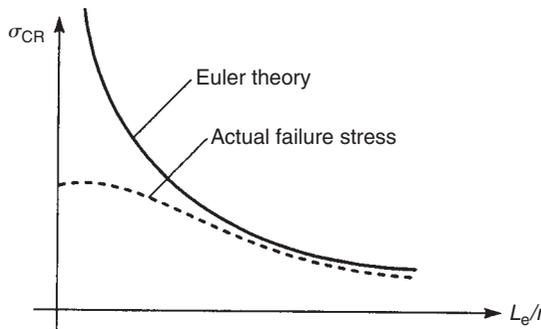
FIGURE 21.9 Variation of critical stress with slenderness ratio
