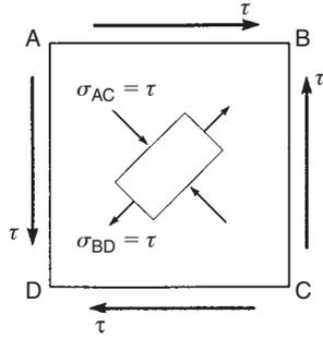
FIGURE 7.12 Stresses on diagonal planes in element
