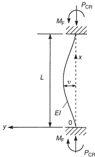
FIGURE 21.5 Buckling of a slender column with fixed ends
