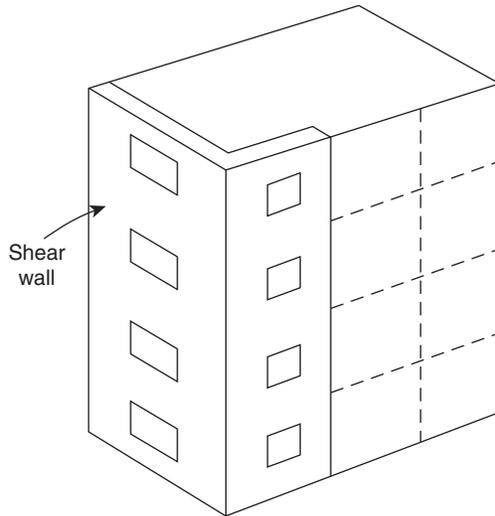
FIGURE 1.9 Shear wall construction
