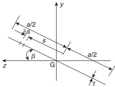
FIGURE 9.29 Second moments of area of an inclined thin-walled section
