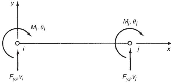
FIGURE 17.6 Forces and moments on a beam element
