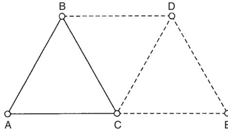
**FIGURE 4.6** Construction of a Warren truss
