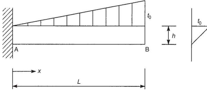
The temperature,  $t$ , at any section  $x$  of the beam is given by
