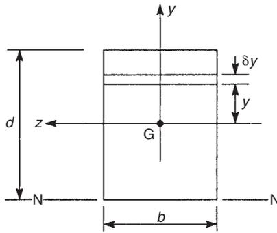
FIGURE 9.21 Second moments of area of a rectangular section
