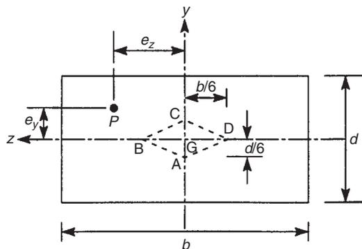
FIGURE 9.11 Core of a rectangular section
