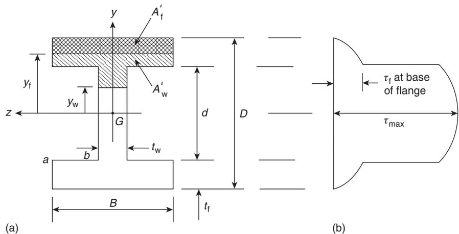
**FIGURE 10.6** Shear stress distribution in an I-section beam
