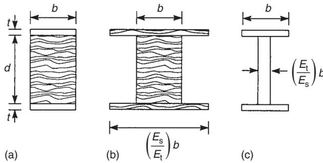
FIGURE 12.4 Reinforced timber beam with steel plates attached to its top and bottom surfaces
