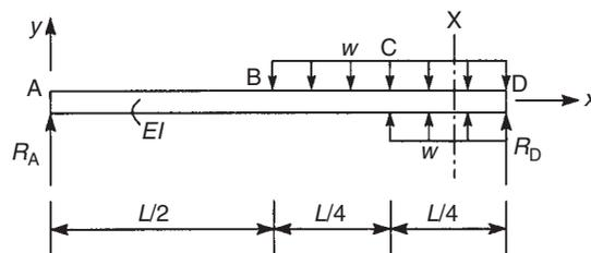
**FIGURE 13.11** Method of solution for a part span uniformly distributed load
