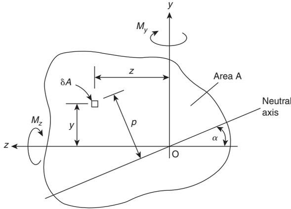
FIGURE 9.18 Bending of an unsymmetrical section beam
