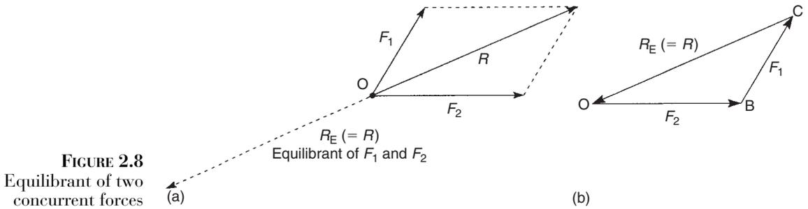
O, as shown in Fig. 2.8(a).  $R_E$  is known at the *equilibrant* of  $F_1$  and  $F_2$  and the particle at O will then be in *equilibrium* and remain stationary. In other words the forces  $F_1$ ,  $F_2$  and  $R_E$  are in equilibrium and, by reference to Fig. 2.3(b), we see that these three forces may be represented by the triangle of vectors OBC as shown in Fig. 2.8(b). This result leads directly to the law of the *triangle of forces* which states that:
