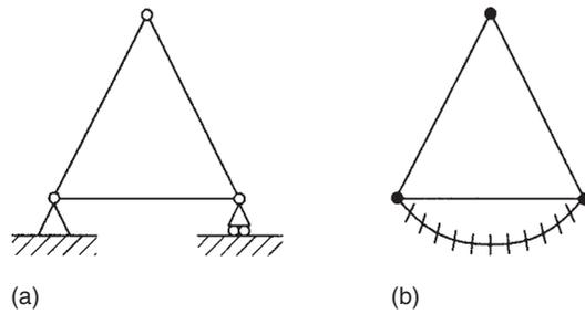
**FIGURE 16.7** A completely stiff structure
