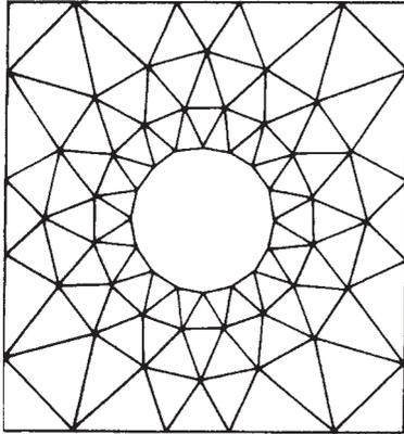
**FIGURE 17.12** Finite element idealization of a flat plate with a central hole
