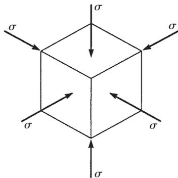
FIGURE 7.7 Cube subjected to hydrostatic pressure
