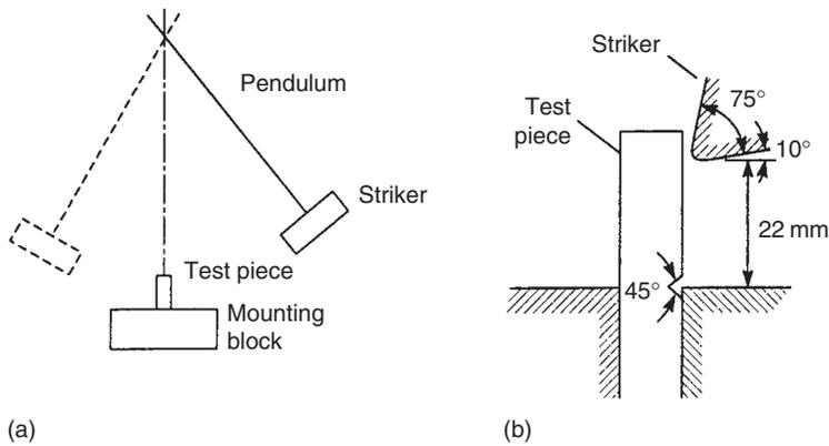
FIGURE 8.6 Izod impact test (a)
