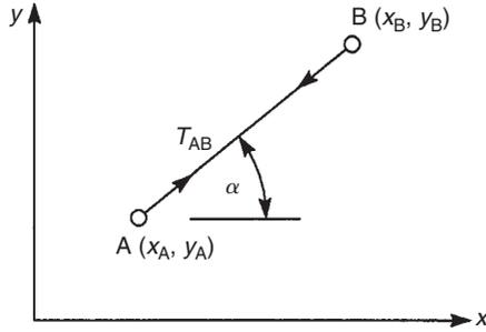
FIGURE 4.19 Method of tension coefficients
