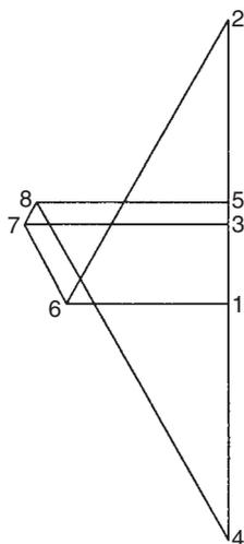
FIGURE 4.22 Force polygon for the truss of Ex. 4.5
