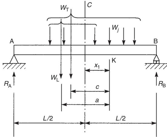
**FIGURE 20.13** Determination of the absolute maximum bending moment in a beam
