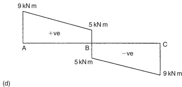
FIGURE 3.23 Torsion diagram for the beam of Ex. 3.13
