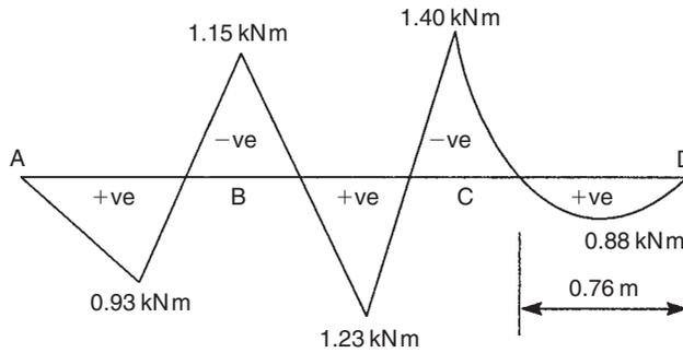
FIGURE 16.35 Bending moment diagram for the beam of Ex. 16.15
