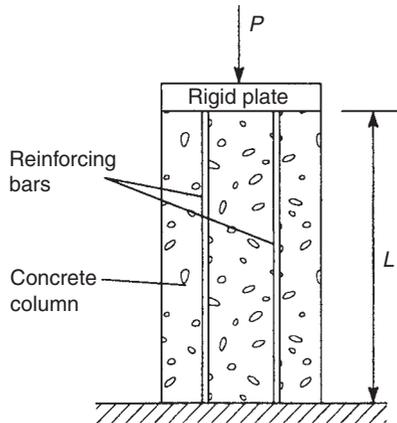
FIGURE 7.17 Composite concrete column
