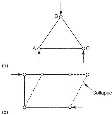
FIGURE 4.3 Basic unit of a truss
