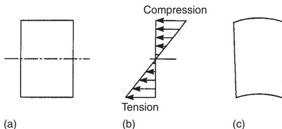
FIGURE 9.14 Anticlastic bending of a beam section
