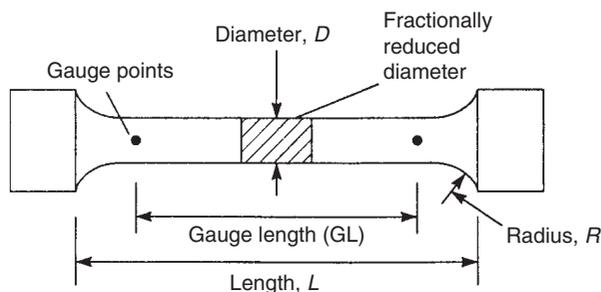
FIGURE 8.1 Standard cylindrical test piece
