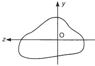
FIGURE 9.20 Theorem of perpendicular axes
