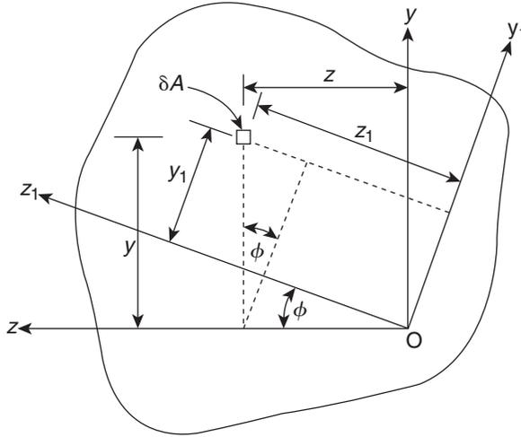
FIGURE 9.31 Principal axes in a beam of arbitrary section
