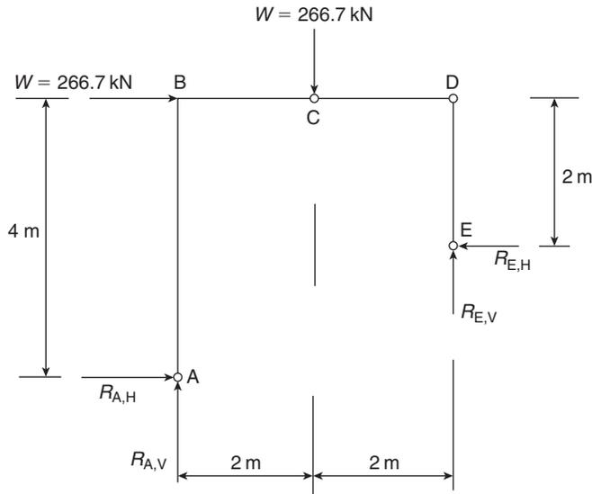
FIGURE 18.18 Support reactions at collapse in the frame of Ex. 18.8
