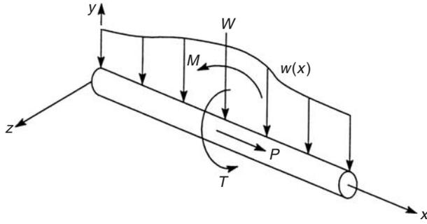
FIGURE 15.7 Virtual work due to externally applied loads
