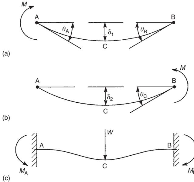
FIGURE 15.25 Model analysis of a fixed beam
