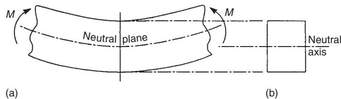
FIGURE 9.4 Bending of a symmetrical section beam
