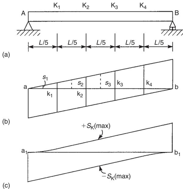
FIGURE 20.10 Diagram of maximum shear force
