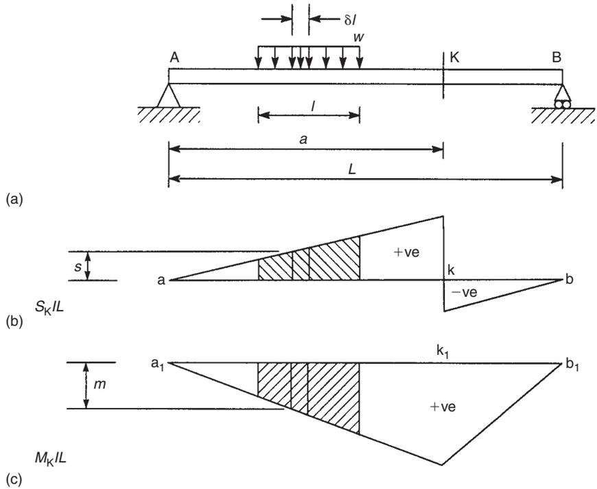
**FIGURE 20.7** Shear force and bending moment due to a moving uniformly distributed load
