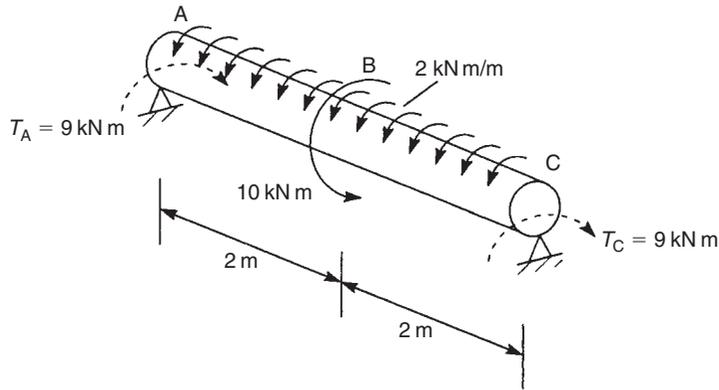
FIGURE 3.22 Beam of Ex. 3.13
