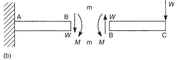
**FIGURE 3.5** Internal force system generated by an external shear load
