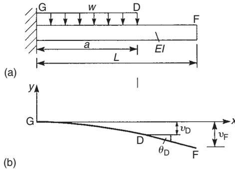
**FIGURE 13.4** Cantilever beam of Ex. 13.3
