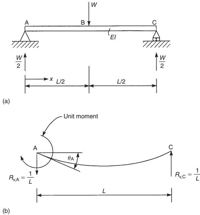
**FIGURE 15.11** Determination of the rotation of a simply supported beam at a support using the unit load method
