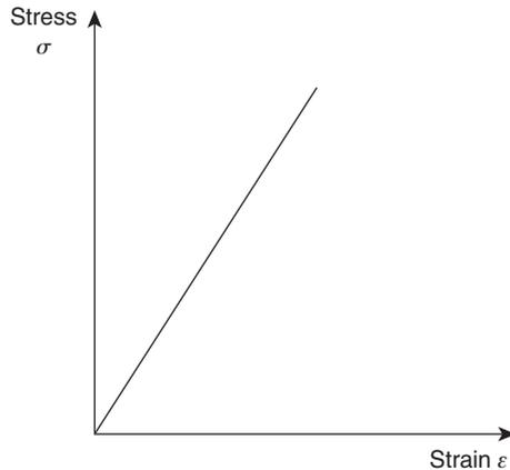
**FIGURE 8.16** Stress–strain curve for a fibre composite
