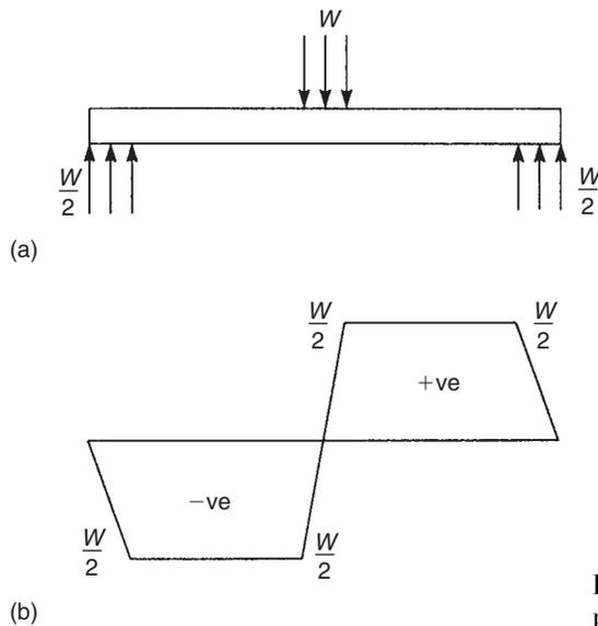
**FIGURE 3.14** Shear force diagram in a practical situation
