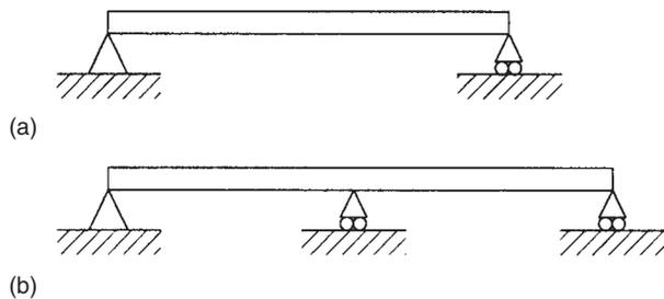
**FIGURE 1.14** (a) Simply supported beam and (b) continuous beam
