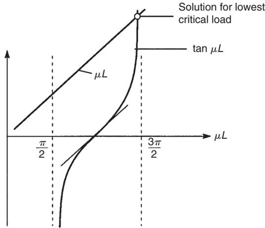
FIGURE 21.8 Solution of a transcendental equation
