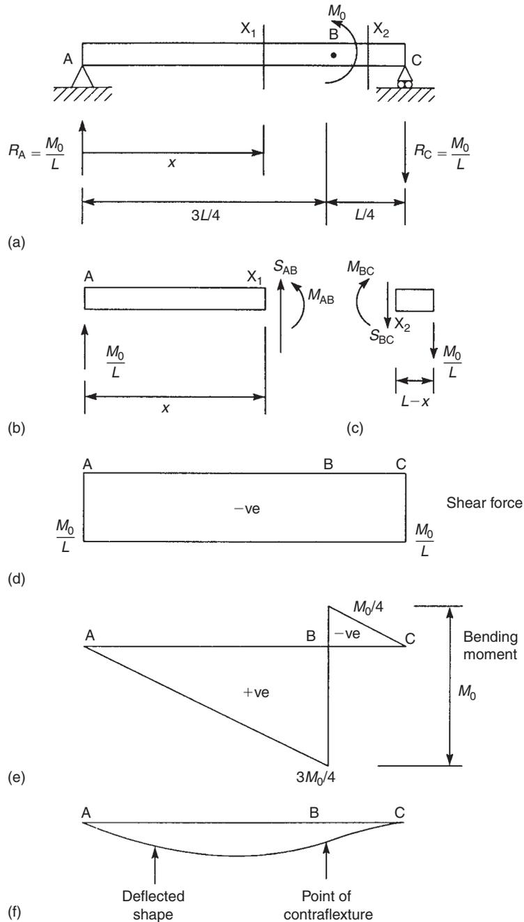
**FIGURE 3.17** Shear force and bending moment diagrams for the beam of Ex. 3.9
