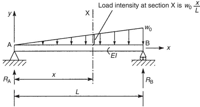
**FIGURE 13.8** Deflection of a simply supported beam carrying a triangularly distributed load
