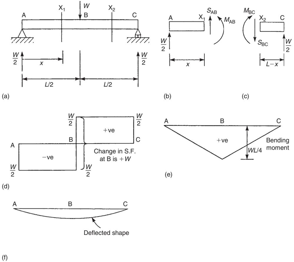
**FIGURE 3.13** Shear force and bending moment diagrams for the beam of Ex. 3.6
