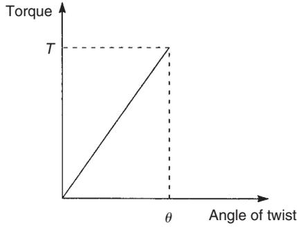
FIGURE 11.8 Torque–angle of twist relationship for a gradually applied torque
