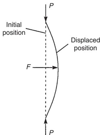
FIGURE 21.2 Definition of buckling load of a column
