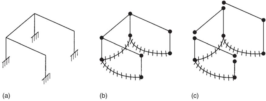
equivalent is shown in Fig. 16.8(b) where we observe by inspection that it consists of three rings, each of which is six times statically indeterminate so that the completely stiff structure is  $3 \times 6 = 18$  times statically indeterminate. Although the number of rings in simple cases such as this is easily found by inspection, more complex cases require a more methodical approach.
