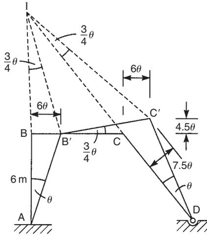
FIGURE 16.50 Arbitrary sway and virtual displacement geometry of frame of Ex. 16.23
