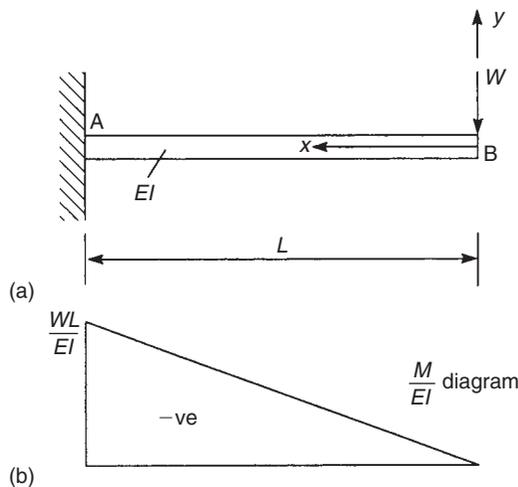
**FIGURE 13.13** Moment-area method for the deflection of a cantilever (Ex. 13.11)
