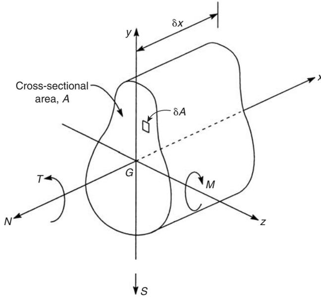
FIGURE 15.5 Virtual work due to internal force system
