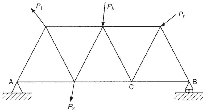
**FIGURE 15.15** Deflection of a truss using complementary energy
