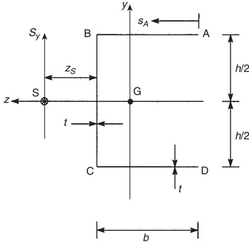
FIGURE 10.17 Channel section beam of Ex. 10.5
