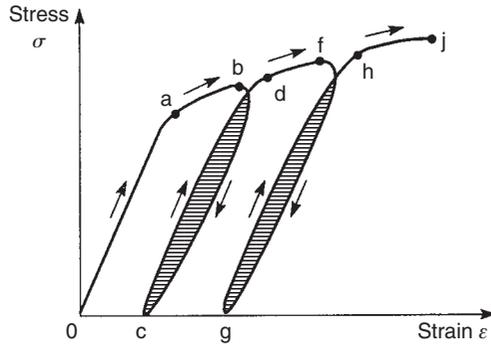
FIGURE 8.17 Strain hardening of a material
