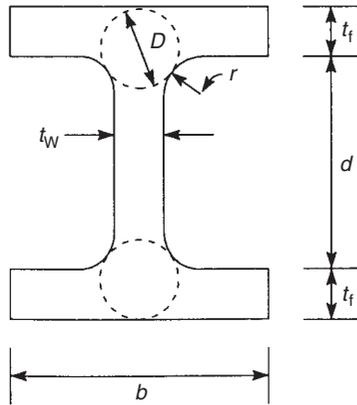
**FIGURE 11.14** Torsion constant for a 'thick' I-section beam
