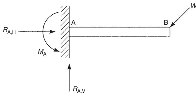
**FIGURE 1.16** Support reactions in a cantilever beam subjected to an inclined load at its free end
