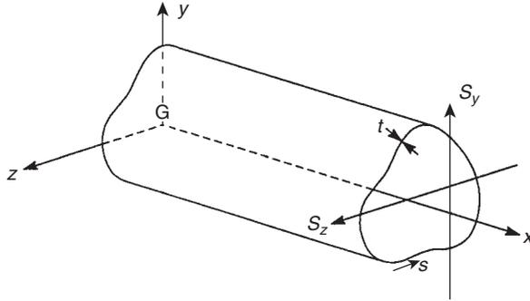
**FIGURE 10.18** Shear of a thin-walled closed section beam
