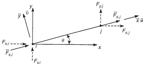
FIGURE 17.3 Local and global axes systems for an axially loaded member
