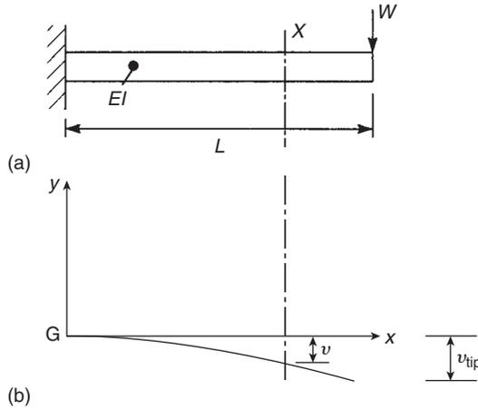
**FIGURE 13.2** Deflection of a cantilever beam carrying a concentrated load at its free end (Ex. 13.1)
