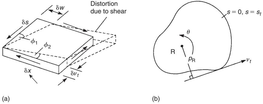
FIGURE 10.20 Rate of twist in a thin-walled closed section beam
