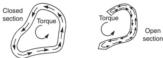
**FIGURE 11.16** Shear stress development in closed and open section beams subjected to torsion
