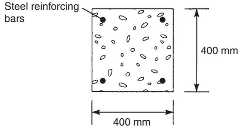
FIGURE 7.18 Reinforced concrete column of Ex. 7.5
