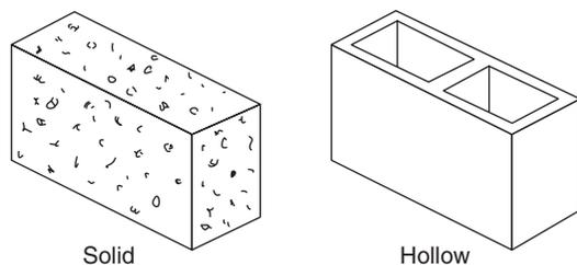
FIGURE 1.24 Concrete blocks
