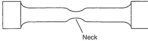
FIGURE 8.9 ‘Necking’ of a test piece in the plastic range
