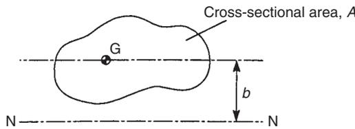
FIGURE 9.19 Parallel axes theorem
