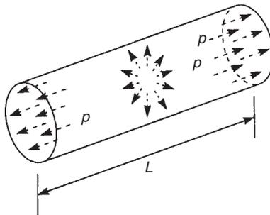
FIGURE 7.22 Thin cylindrical shell under internal pressure
