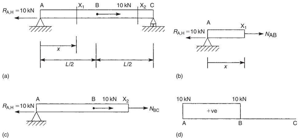
FIGURE 3.9 Normal force diagram for the beam of Ex. 3.2
