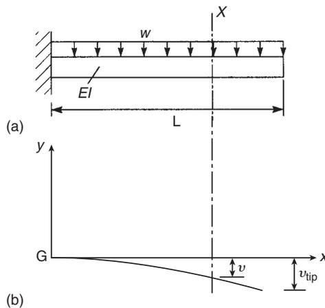
**FIGURE 13.3** Deflection of a cantilever beam carrying a uniformly distributed load
