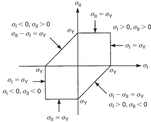
FIGURE 14.20 Yield locus for the Tresca theory of elastic failure
