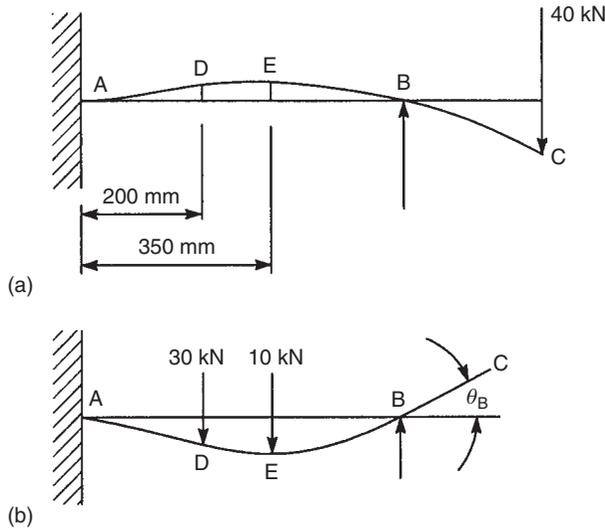
**FIGURE 15.24** Deflection of a propped cantilever using the reciprocal theorem
