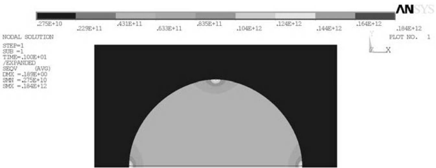
Figure 2.83. Equivalent von Mises stresses in the homogenisation problem \chi^{12}
