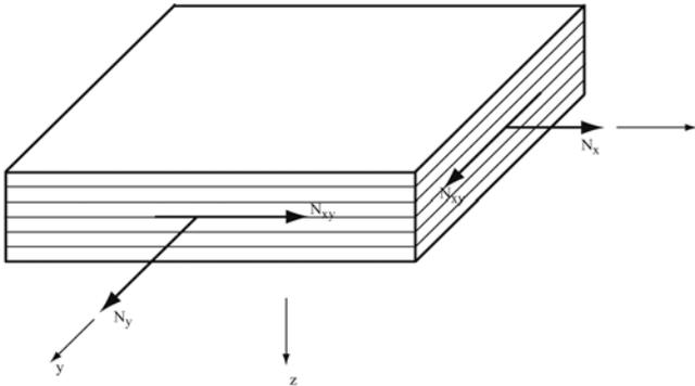
**Fig. 8.1.** Schematic illustration of the force resultants on a composite laminate
