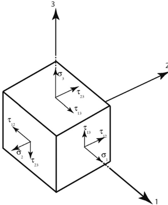
**Fig. 2.2.** An infinitesimal fiber-reinforced element showing the stresses
