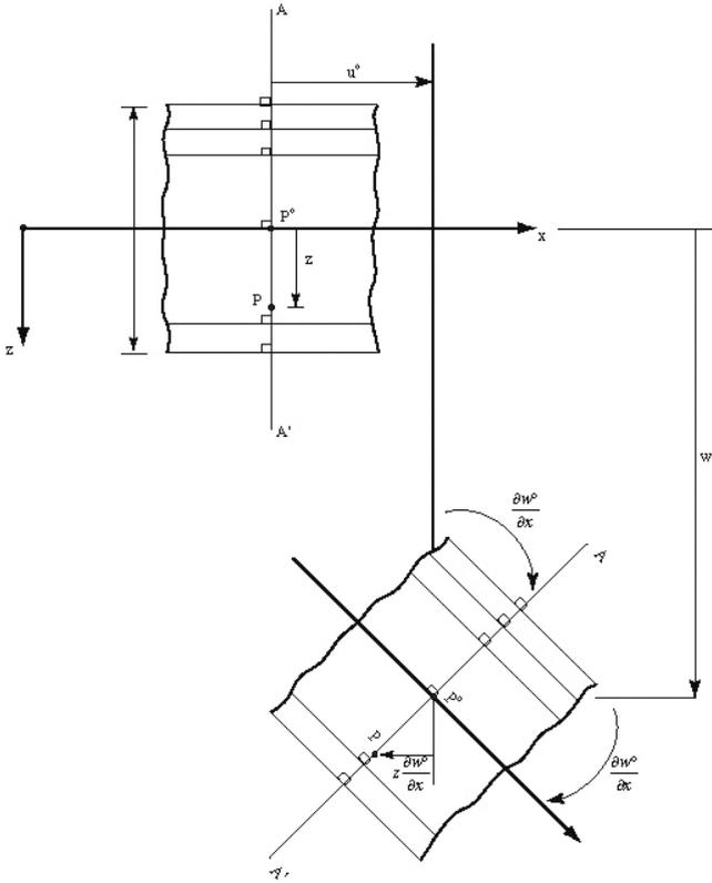
**Fig. 7.3.** Schematic illustration showing the kinematics of deformation of a laminate
