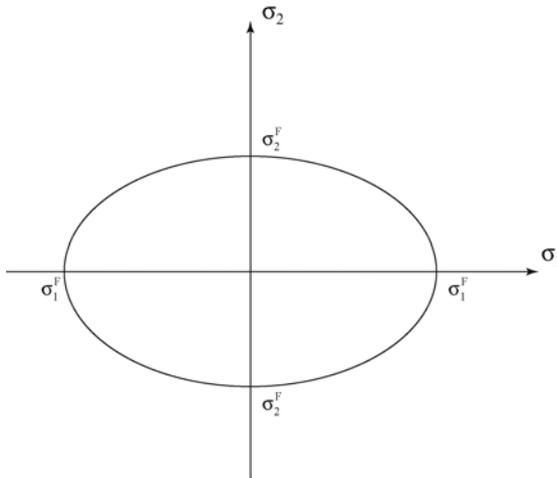
**Fig. 10.7.** Failure envelope for the Tsai-Hill failure theory
