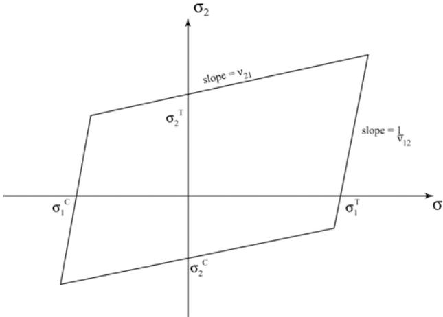
**Fig. 10.5.** Failure envelope for the maximum strain failure theory
