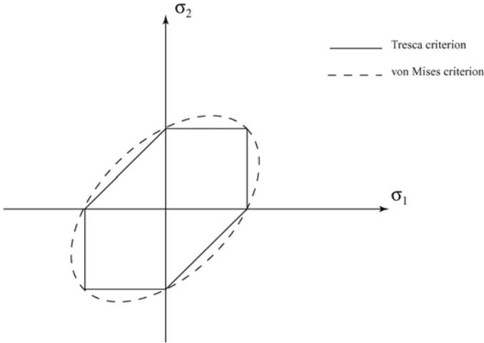
**Fig. 10.10.** Two failure criteria for ductile homogeneous materials
