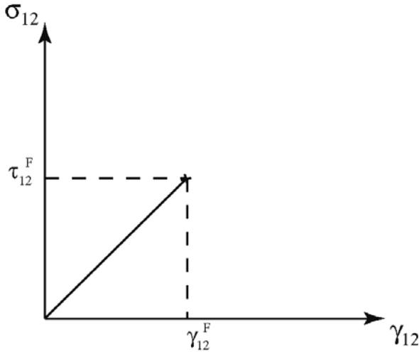
**Fig. 10.3.** Stress-strain curve for the shear loading of a lamina
