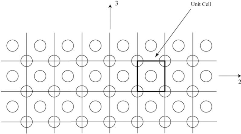
**Fig. 3.2.** A unit cell in a hexagonal-packed array of fiber-reinforced composite material
