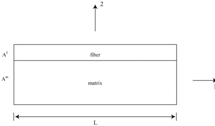
**Fig. 3.3.** A longitudinal cross-section of fiber-reinforced composite material for Example 3.1
