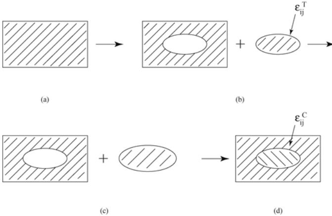
**Fig. 11.1.** Schematic illustration of homogenization according to the Eshelby method
