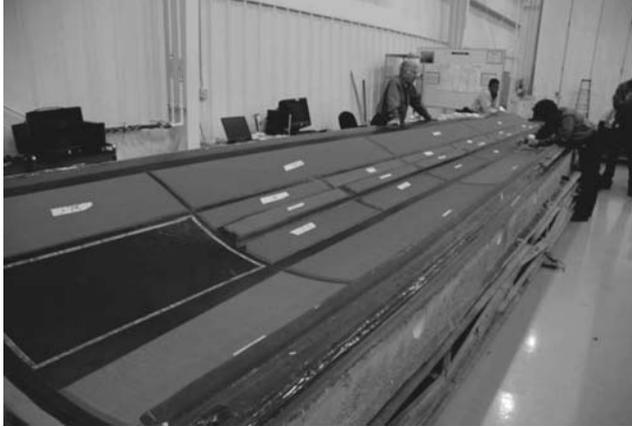
**Figure 2.9** Co-cure of large complex parts (Courtesy Aurora Flight Sciences; see Plate 12 for the colour figure)
