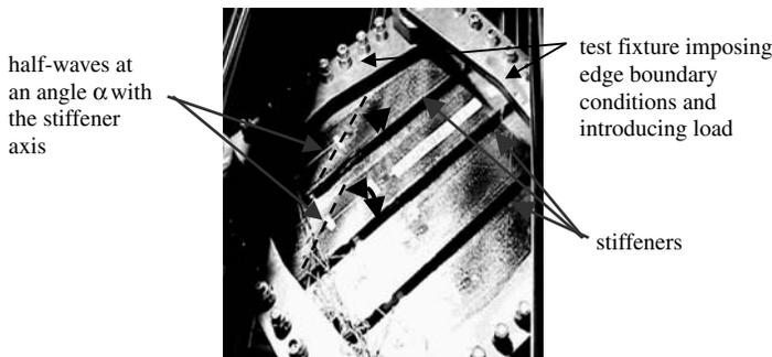
**Figure 7.13** Stiffened composite panel in the post-buckling regime (See Plate 16 for the colour figure)
