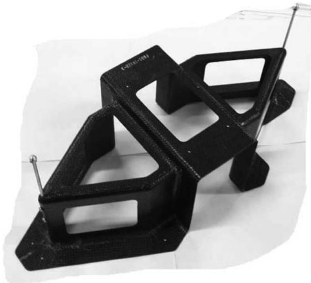
**Figure 2.2** Integration of various parts into a single co-cured part to minimize assembly cost (Courtesy Aurora Flight Sciences)
