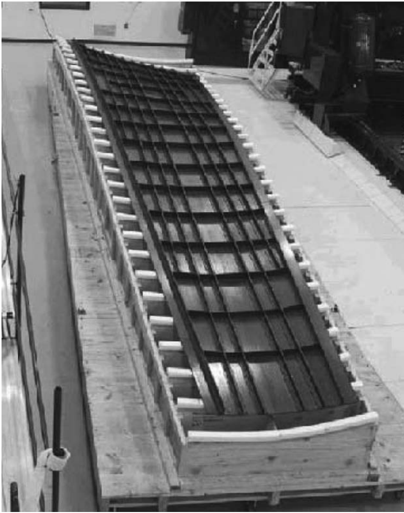
Fig. 5.54 Integral wing cover panel fabricated by the resin film infusion (RFI) process. Source: Ref 16
