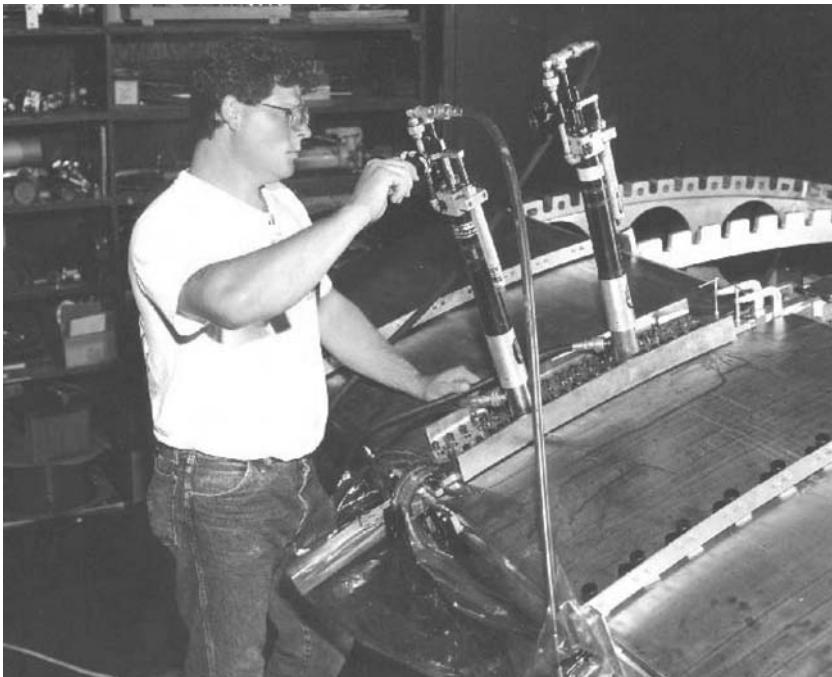
Fig. 20.32 Diamond core drilling of a titanium matrix composite component. Source: The Boeing Company
