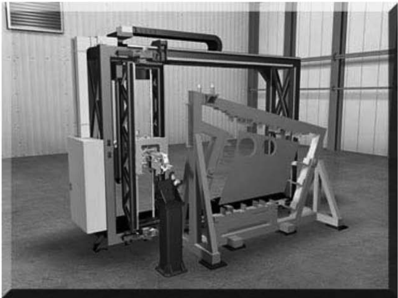
Fig. 11.13 Composite outer wing numerically controlled drill jig (NCDJ) drilling system. Source: The Boeing Company
