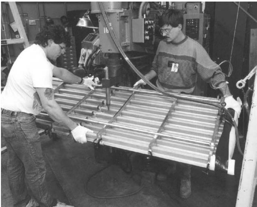
Fig. 20.33 Spot welding titanium matrix composite hat stiffeners. Source: The Boeing Company
