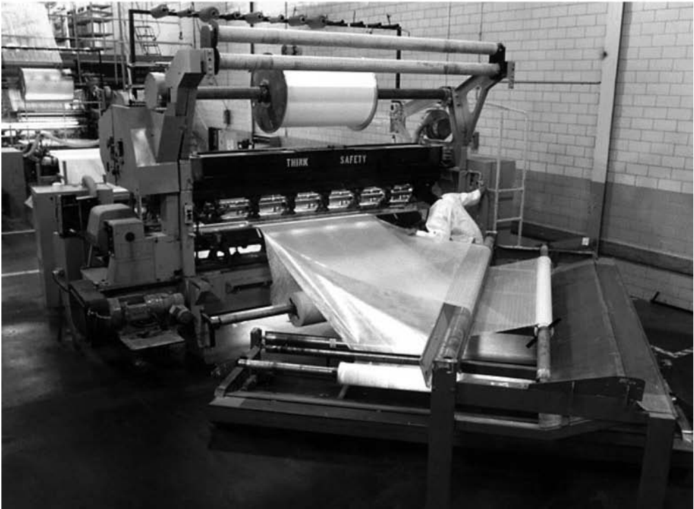
Fig. 2.18 Weaving glass cloth on a textile loom
