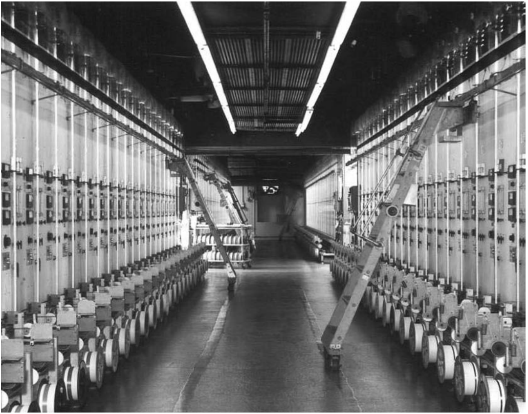
Fig. 20.17 Boron monofilament reactor banks. Source: Specialty Materials Inc.
