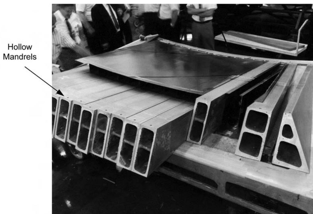
Fig. 9.27 Hollow mandrels to reduce tool mass. Source: The Boeing Company
