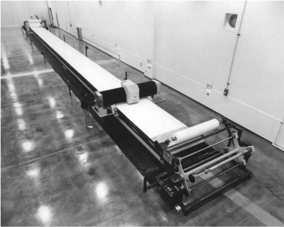
Fig. 5.3 Large ultrasonic ply cutter. Source: The Boeing Company
