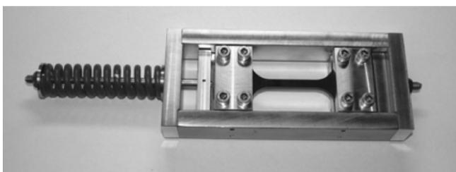
**Fig. 9.30.** Preload aging fixture for neat resin specimens
