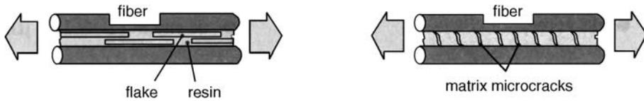
**Figure 3.17** Cross Section with and without Mica
