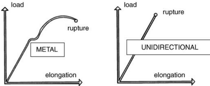
**Figure 3.7 Loading Curves of Metal and Unidirectional Composite**
