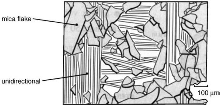
**Figure 3.16 Mica Flakes Arrangement**
