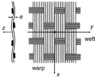
**Figure 3.10** Notation for a Fabric Layer
