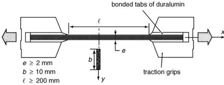
Figure 3.22 Tensile Test
