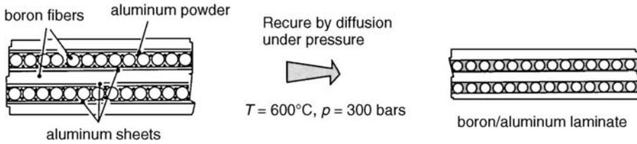
**Figure 3.21 Boron/Aluminum Composite**
