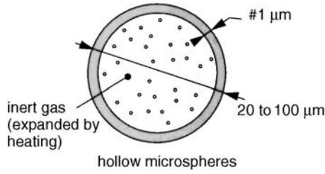
**Figure 3.14 Spherical Fillers**
