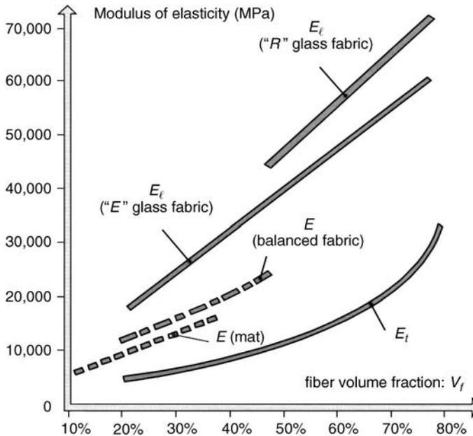
Figure 3.12 Elastic Modulus of Glass/Epoxy Layers
