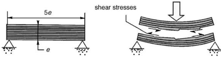
Figure 3.23 Short Beam Shear Test
