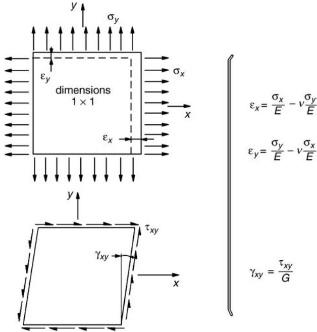
**Figure 3.3 Stress–Strain Behavior in an Isotropic Material**
