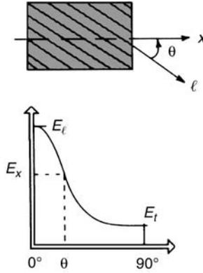
**Figure 3.6 Off-axis Modulus**
