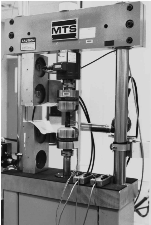
FIGURE 3.25 Tensile coupon mounted in the test frame for finding the tensile strengths of a unidirectional lamina. (Photo courtesy of Dr. R.Y. Kim, University of Dayton Research Institute, Dayton, OH.)
