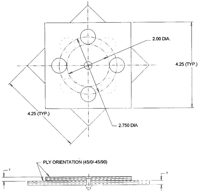
FIGURE 7.5.5.2(d) Assembled test specimen for Procedure A.
