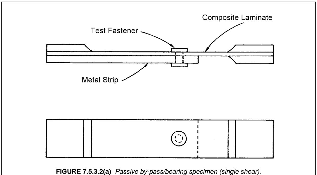
**FIGURE 7.5.3.2(a)** *Passive by-pass/bearing specimen (single shear).*
