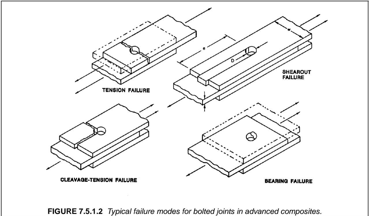
**FIGURE 7.5.1.2** Typical failure modes for bolted joints in advanced composites.
