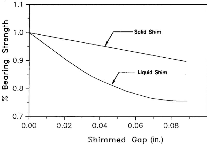
FIGURE 7.5.2.5(b) Bearing strength reduction vs shimmed gap.
