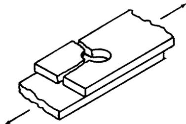
**L-MM: Mixed Mode Failure**
