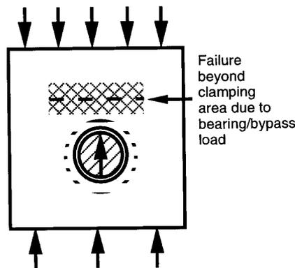
**L-OC: Laminate Off-Set Compression Failure**
