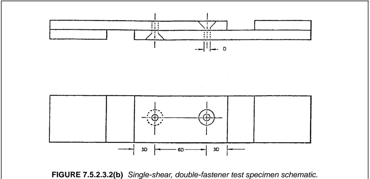
**FIGURE 7.5.2.3.2(b)** *Single-shear, double-fastener test specimen schematic.*
