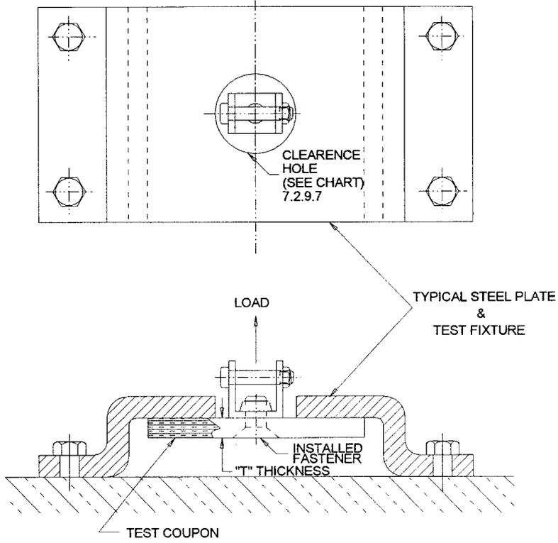
**FIGURE 7.5.5.2(e)** Fastener pull-thru test fixture for Procedure B.
