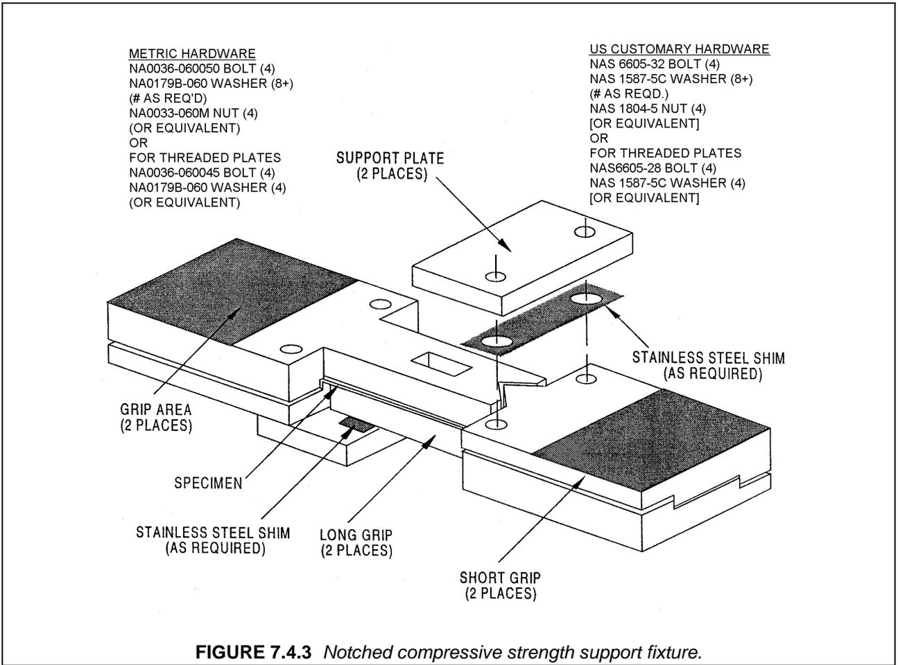
**FIGURE 7.4.3** Notched compressive strength support fixture.
