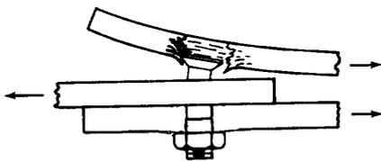
**L-PT: Fastener Pull-Through (or Partial Pull-Through) Failure**
