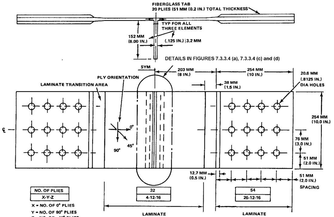
FIGURE 7.6.3.3(c) Specimen configuration.
