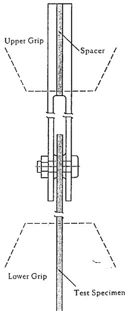
FIGURE 7.5.2.2(b) Fixture assembly for procedure A.
