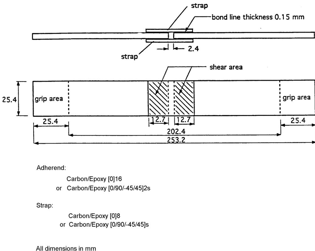
**FIGURE 7.6.3.3(a)** Geometry and materials of the double-lap test specimens.
