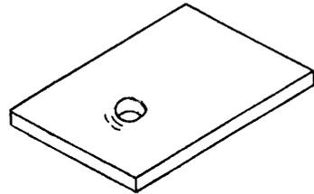
**L-BR: Laminate Bearing Failure**
