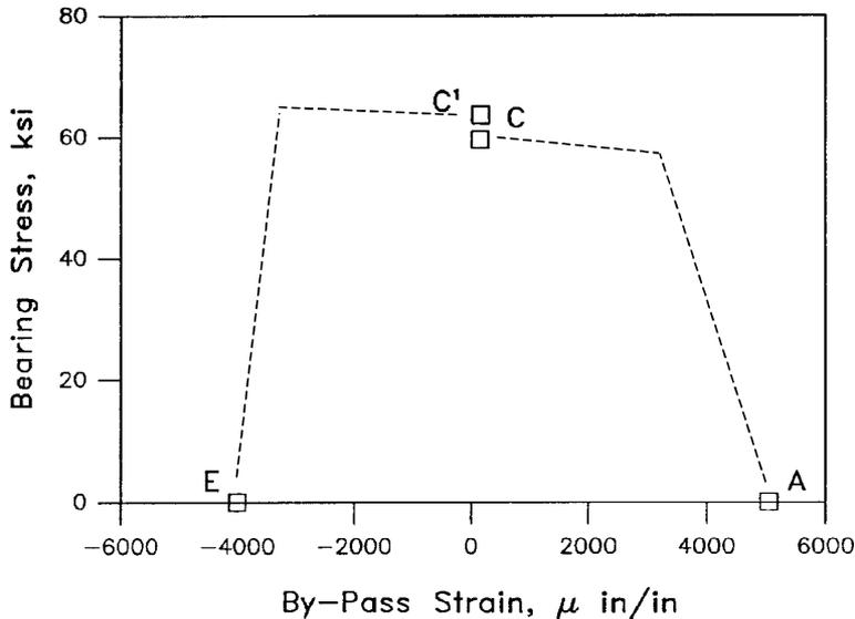
FIGURE 7.5.1.3 Example of bearing/by-pass interaction.
