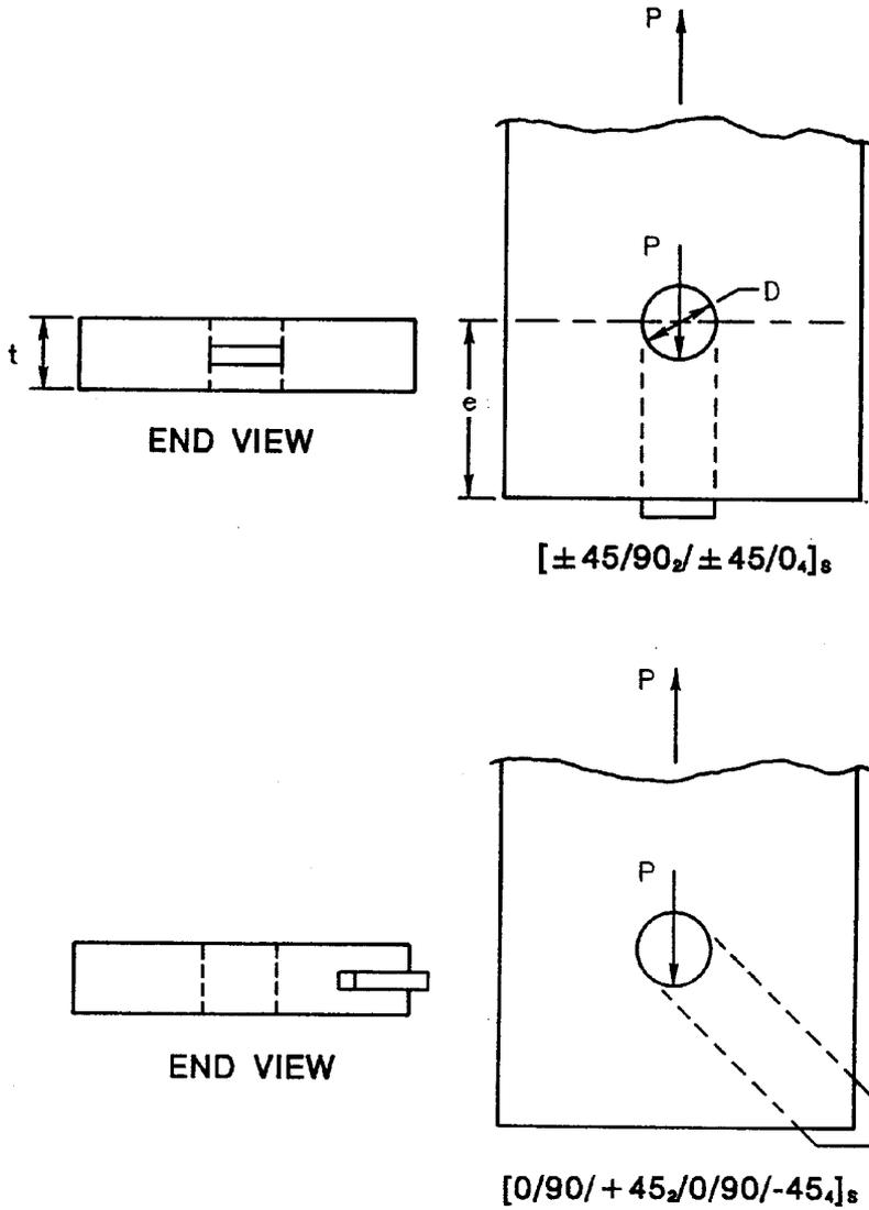
FIGURE 7.5.4(a) *Shear-out failure mode.*
