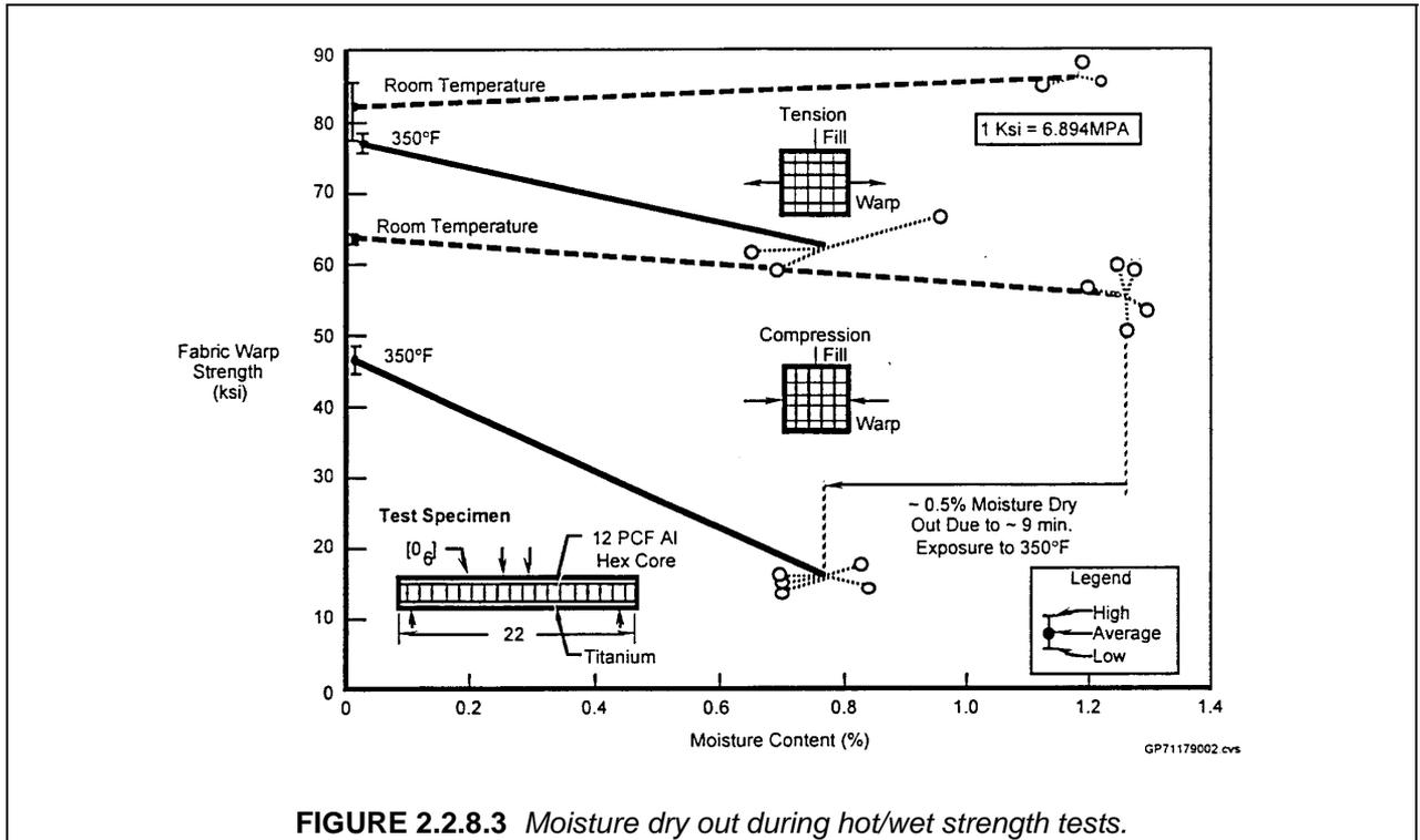
FIGURE 2.2.8.3 Moisture dry out during hot/wet strength tests.
