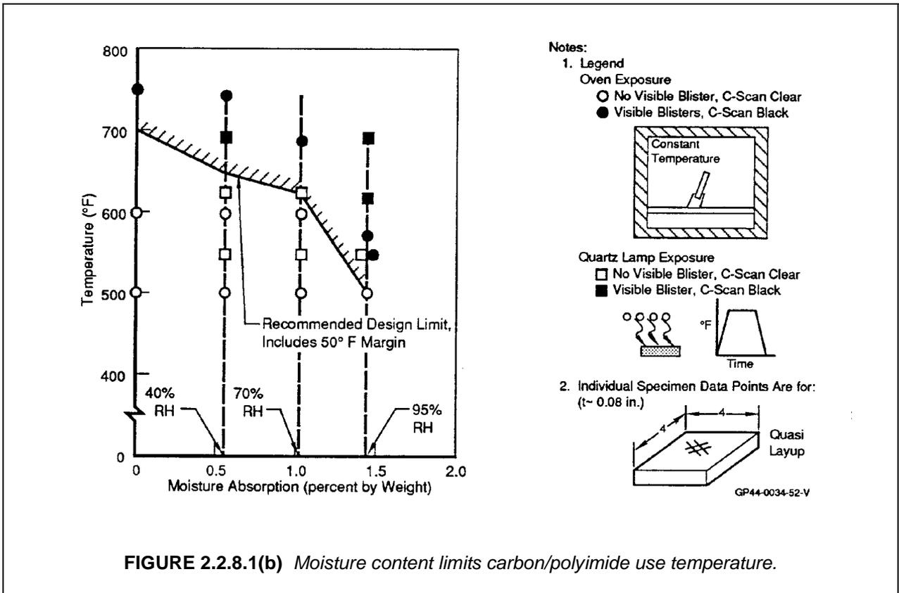
FIGURE 2.2.8.1(b) Moisture content limits carbon/polyimide use temperature.
