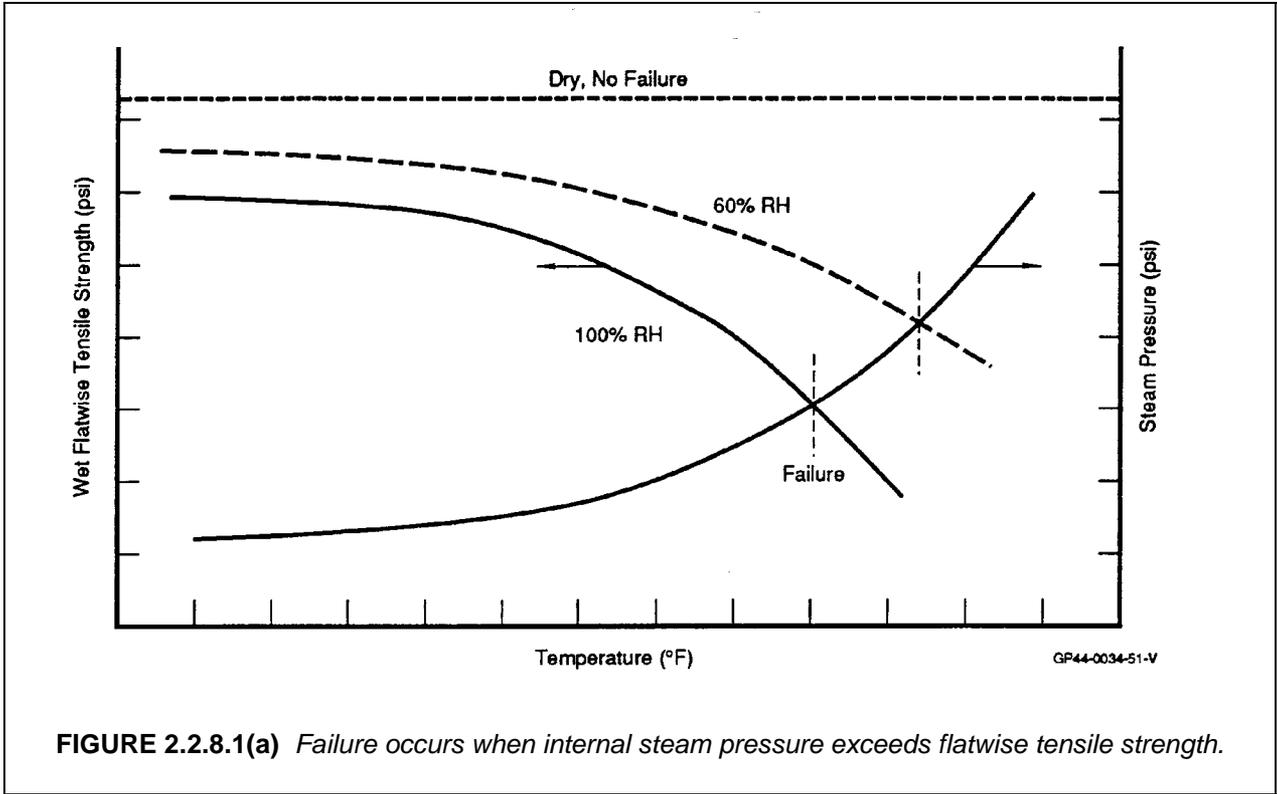
FIGURE 2.2.8.1(a) Failure occurs when internal steam pressure exceeds flatwise tensile strength.
