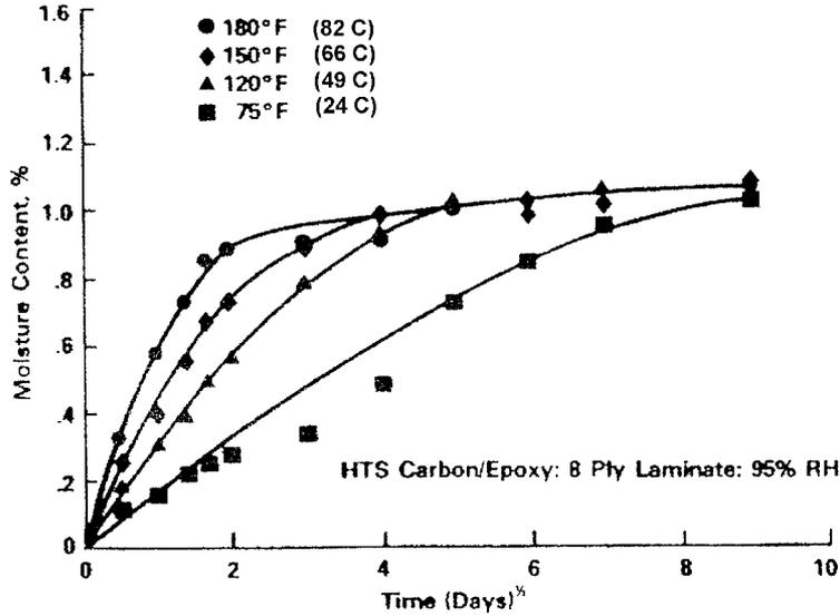
FIGURE 2.2.7(a) Typical moisture absorption response (Reference 2.2.7(d)).
