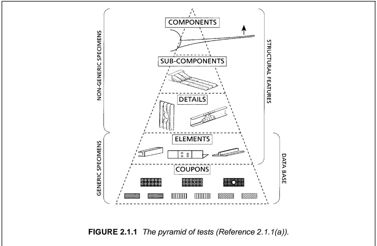
**FIGURE 2.1.1** *The pyramid of tests (Reference 2.1.1(a)).*
