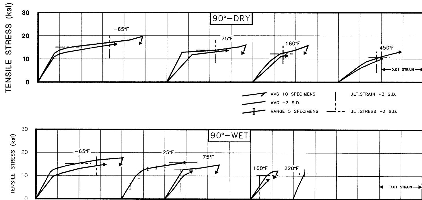
FIGURE A1.3.1(b) Tensile stress-strain for F-161/7743 fiberglass epoxy loaded in the 90° direction.
