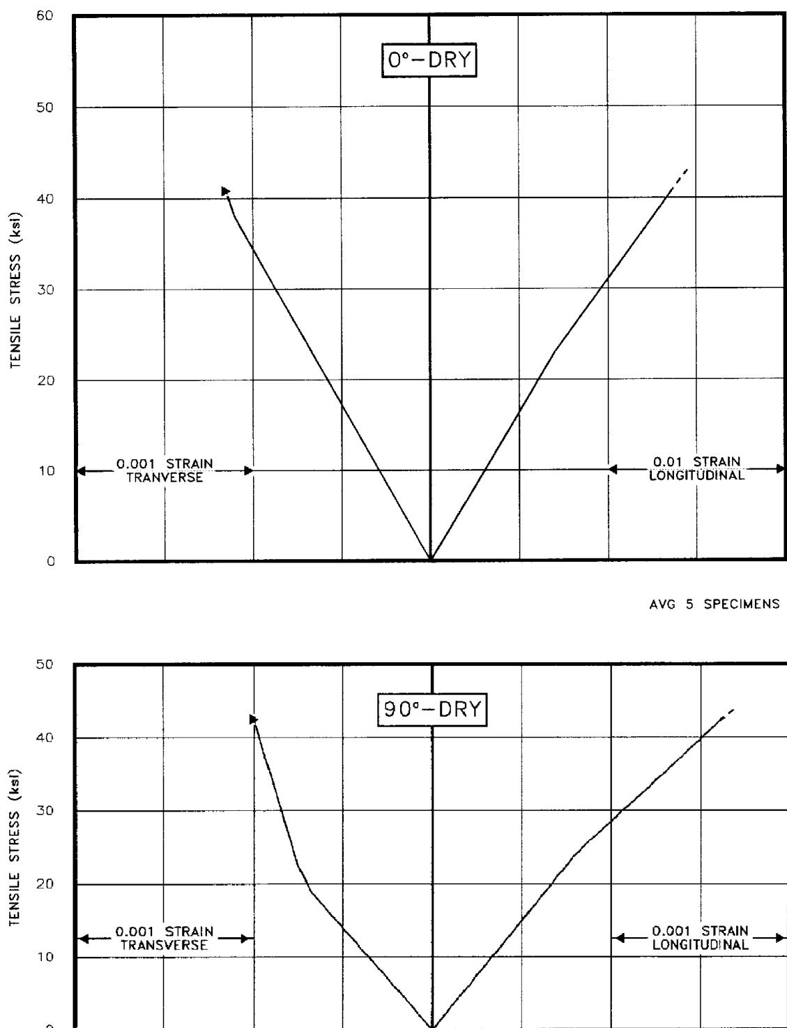
**FIGURE A1.6.4** Poisson effects for F-161/7781 fiberglass epoxy (36% resin).
