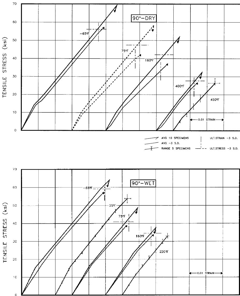
**FIGURE A1.6.1(b)** Tensile stress-strain for F-161/7781 fiberglass epoxy loaded in the 90° direction (36% resin).
