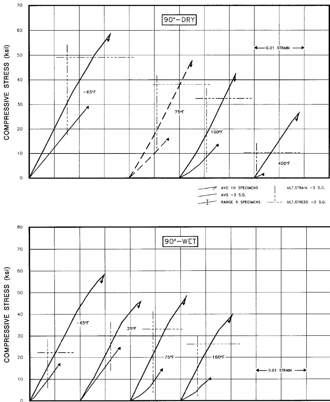
**FIGURE A1.5.2(b)** Compressive stress-strain for F-161/7781 fiberglass epoxy loaded in the 90° direction (31% resin).
