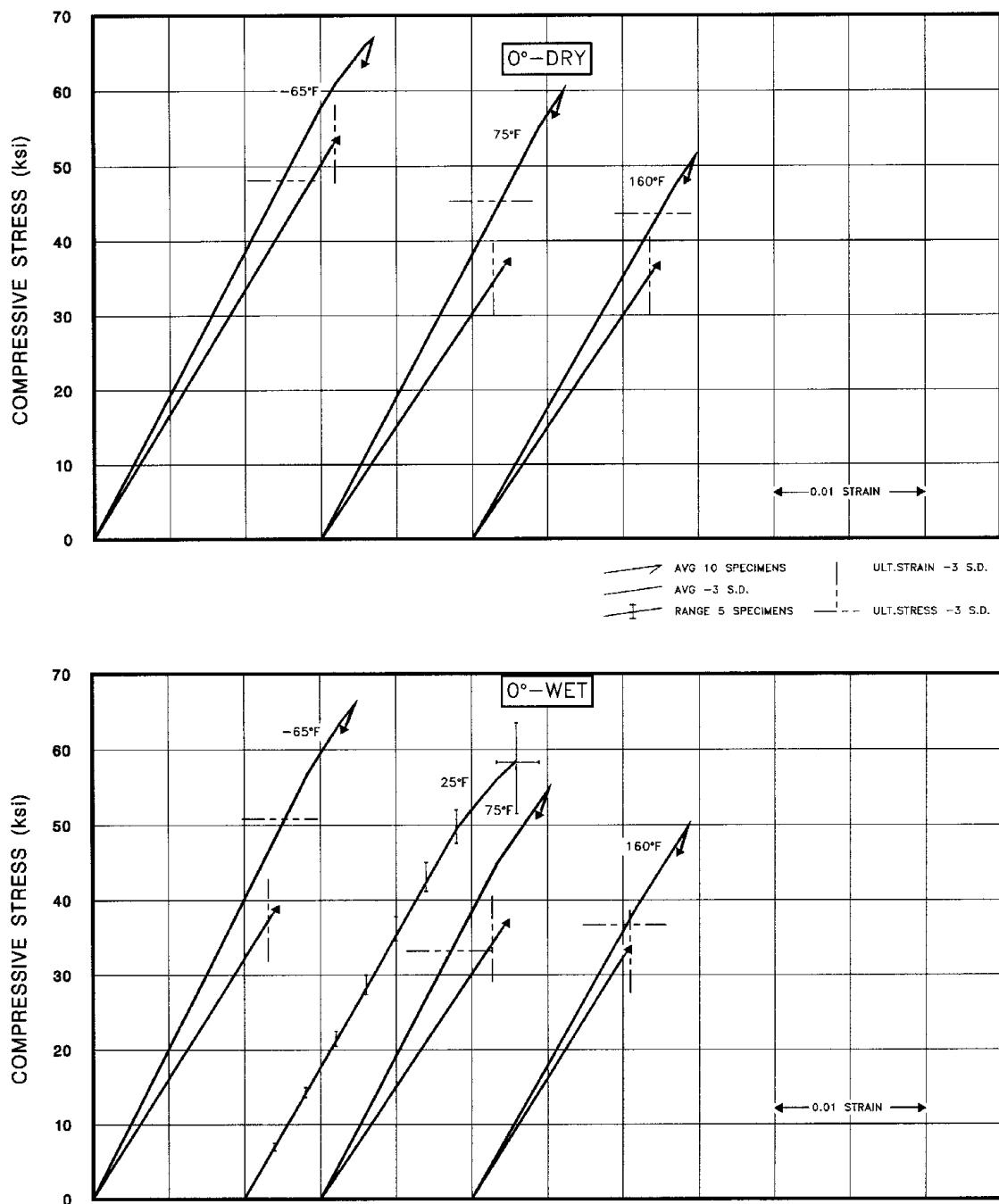
**FIGURE A1.40.2(a)** Compressive stress-strain for N506-7781 fiberglass phenolic loaded in the 0° direction.
