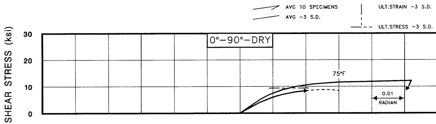
**FIGURE A1.40.3**  $0^\circ$  -  $90^\circ$  rail shear for N506/7781 fiberglass phenolic.
