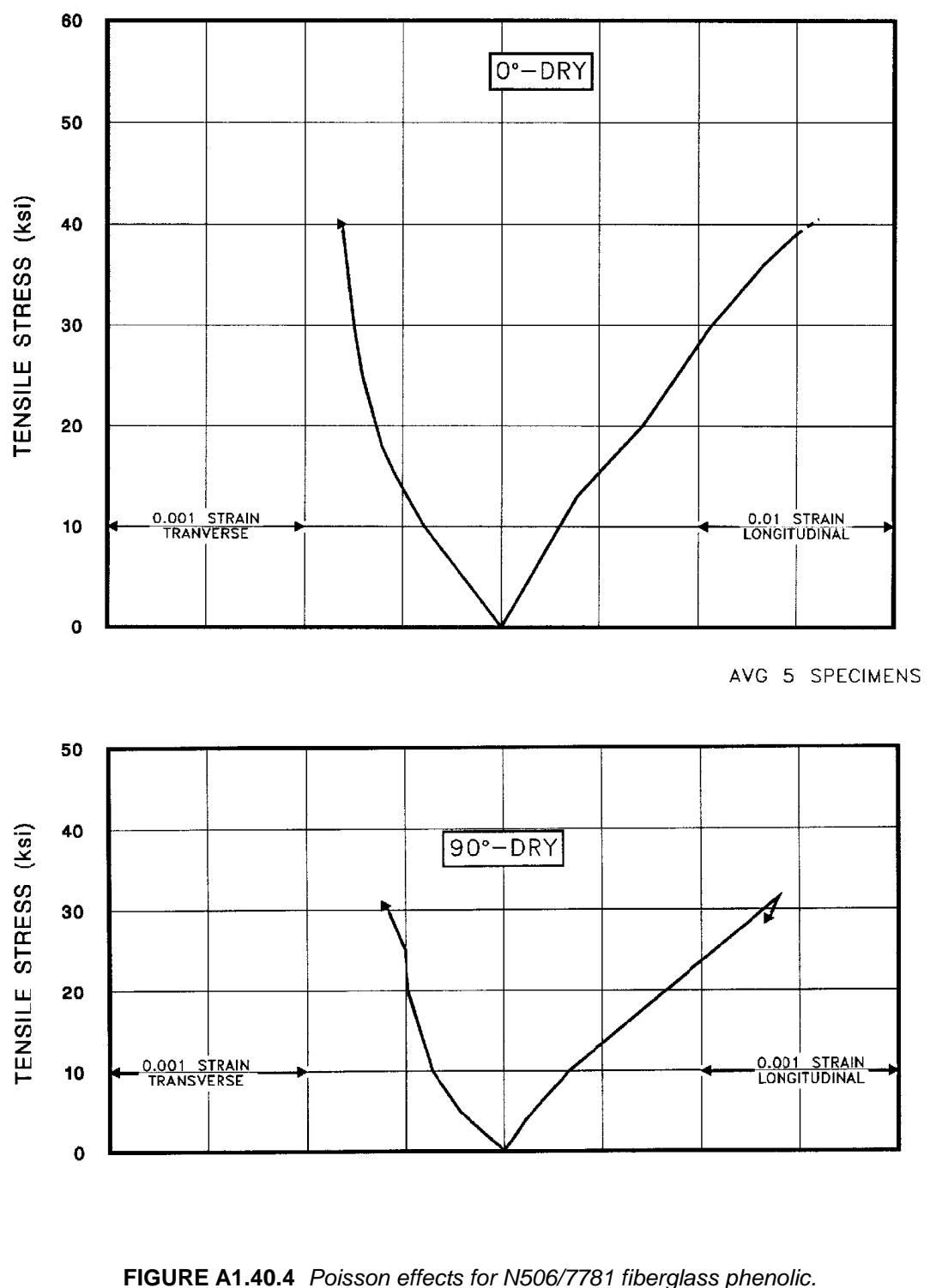
**FIGURE A1.40.4** Poisson effects for N506/7781 fiberglass phenolic.
