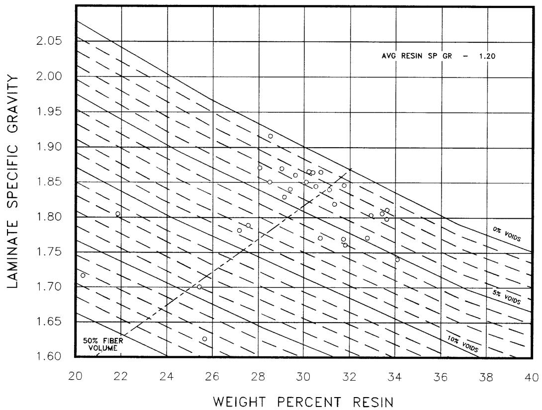
**FIGURE A1.40.5** Voids vs. resin content and specific gravity for N506/7781 fiberglass phenolic.
