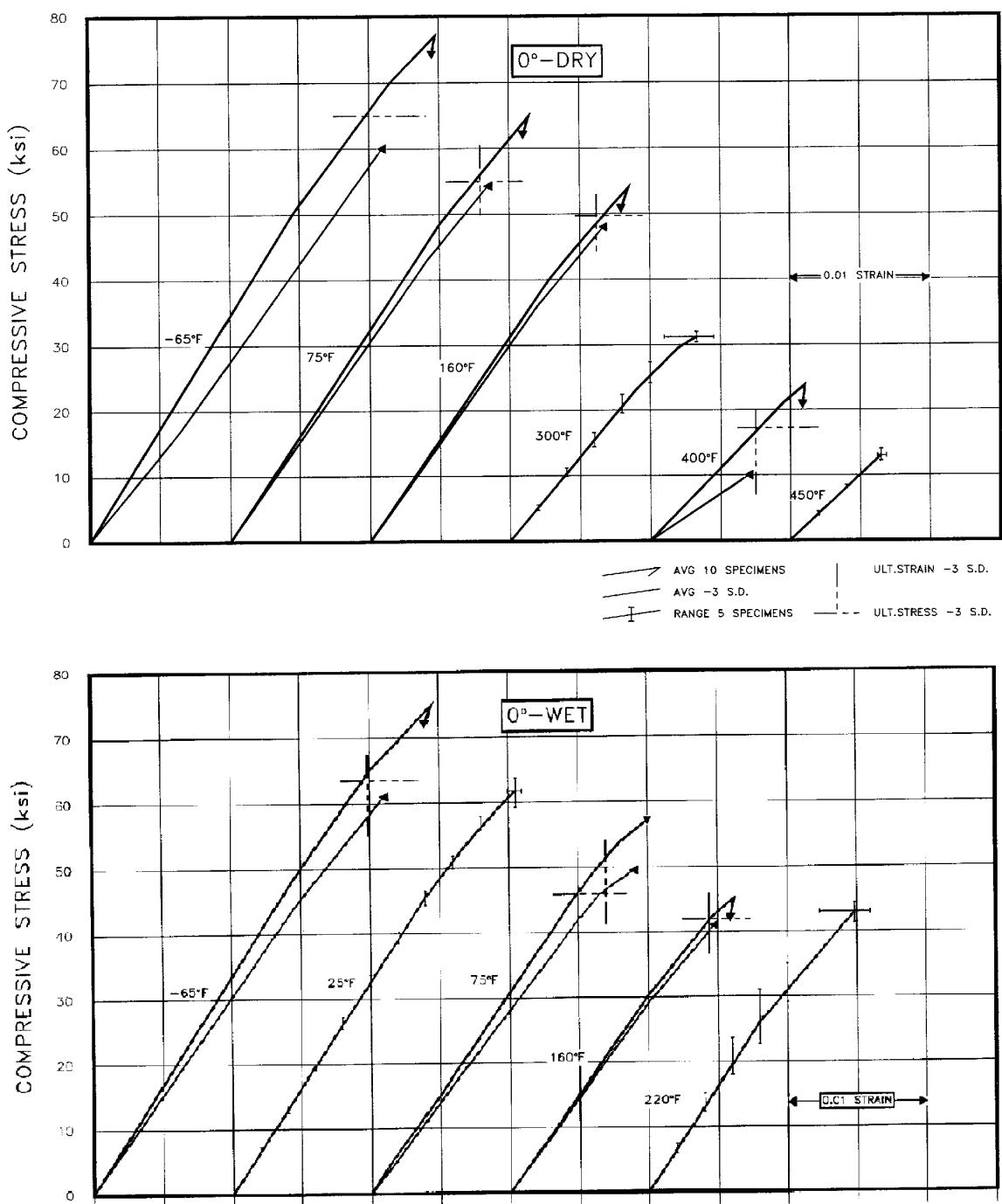
**FIGURE A1.1.2(a)** Compressive stress-strain for E-720E/7781 fiberglass epoxy loaded in the 0° direction.
