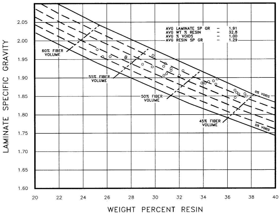
**FIGURE A1.8.5** Voids vs. resin content and specific gravity for N588/7781 fiberglass epoxy.
