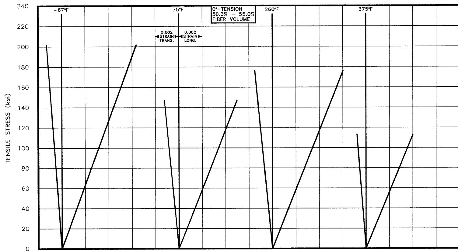
FIGURE A1.110.3 Poisson effects for AVCO 5505 boron/epoxy (100% - 0° direction).
