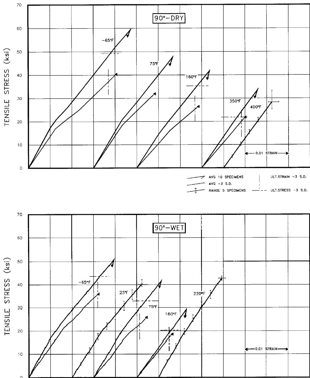
**FIGURE A1.8.1(b)** Tensile stress-strain for N588/7781 fiberglass epoxy loaded in the 90° direction.
