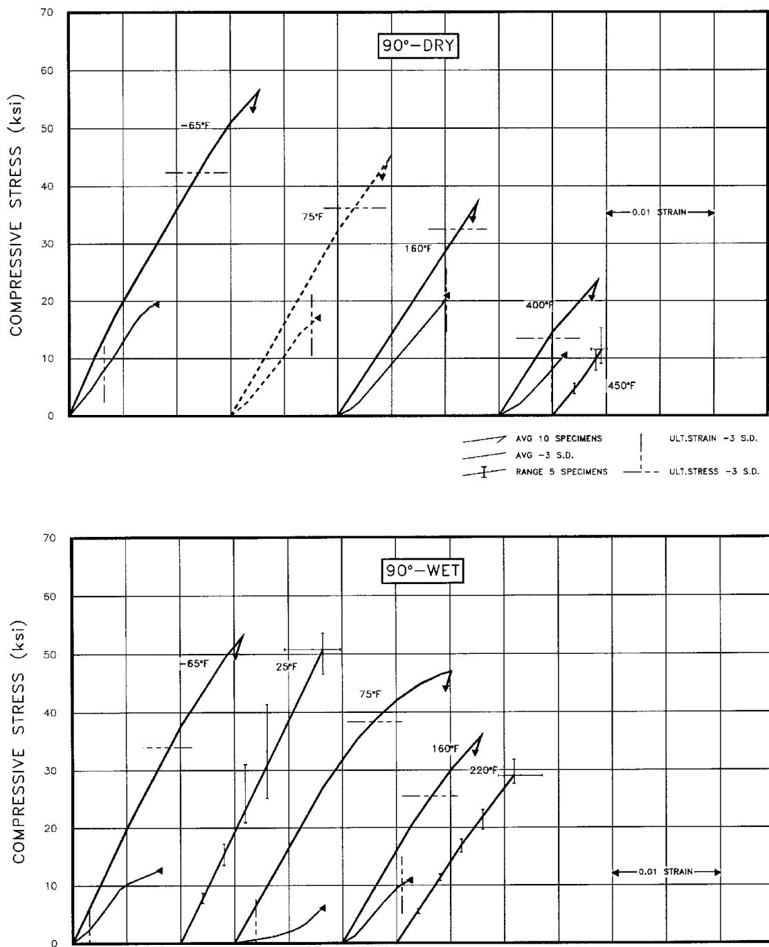
**FIGURE A1.6.2(b)** Compressive stress-strain for F-161/7781 fiberglass epoxy loaded in the 90° direction (36% resin).
