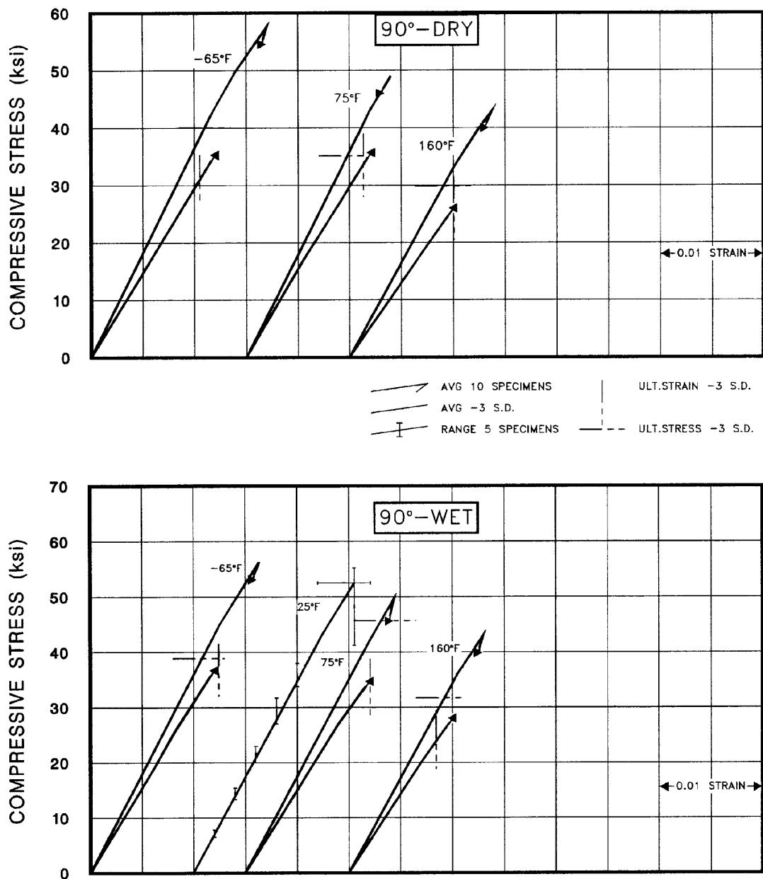
**FIGURE A1.40.2(b)** Compressive stress-strain for N506/7781 fiberglass phenolic loaded in the 90° direction.
