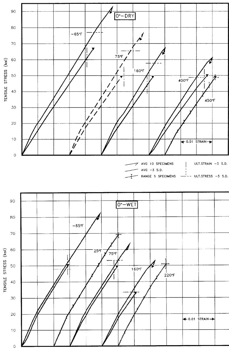
**FIGURE 1.4.1(a)** Tensile stress-strain for F-161/7781 fiberglass epoxy loaded in the 0° direction (26% resin).
