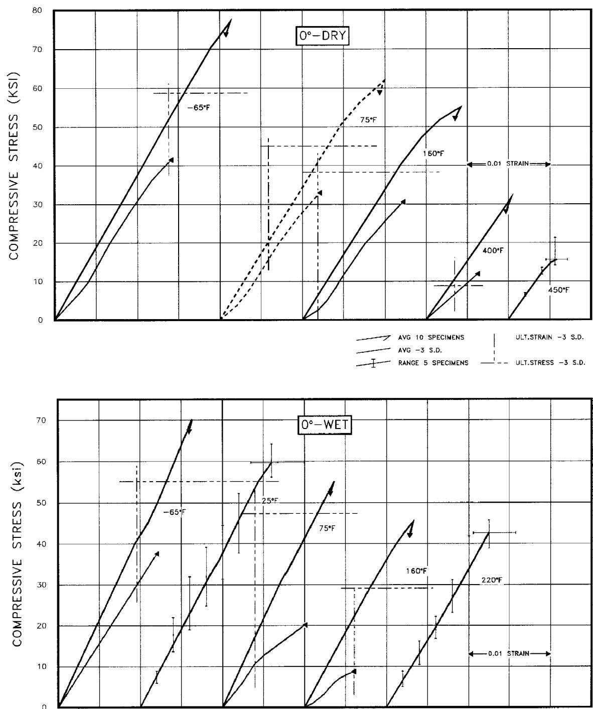
**FIGURE A1.6.2(a)** Compressive stress-strain for F-161/7781 fiberglass epoxy loaded in the 0° direction (36% resin).
