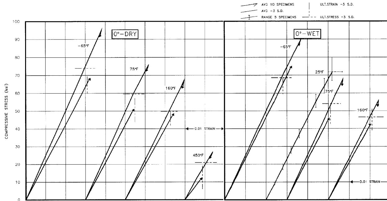
**FIGURE A1.3.2(a)** Compressive stress-strain for F-161/7743 fiberglass epoxy loaded in the 0° direction.
