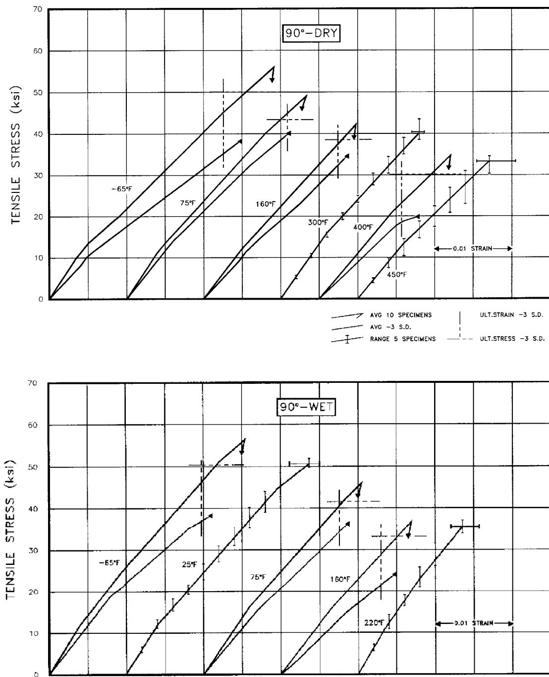
**FIGURE A1.1.1(b)** Tensile stress-strain for E-720E/7781 fiberglass epoxy loaded in the 90° direction.
