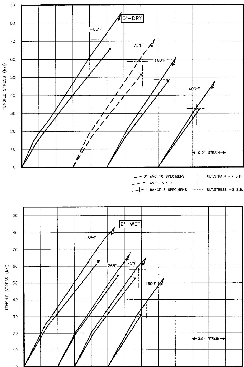
**FIGURE A1.5.1(a)** Tensile stress-strain for F-161/7781 fiberglass epoxy loaded in the 0° direction (31% resin).
