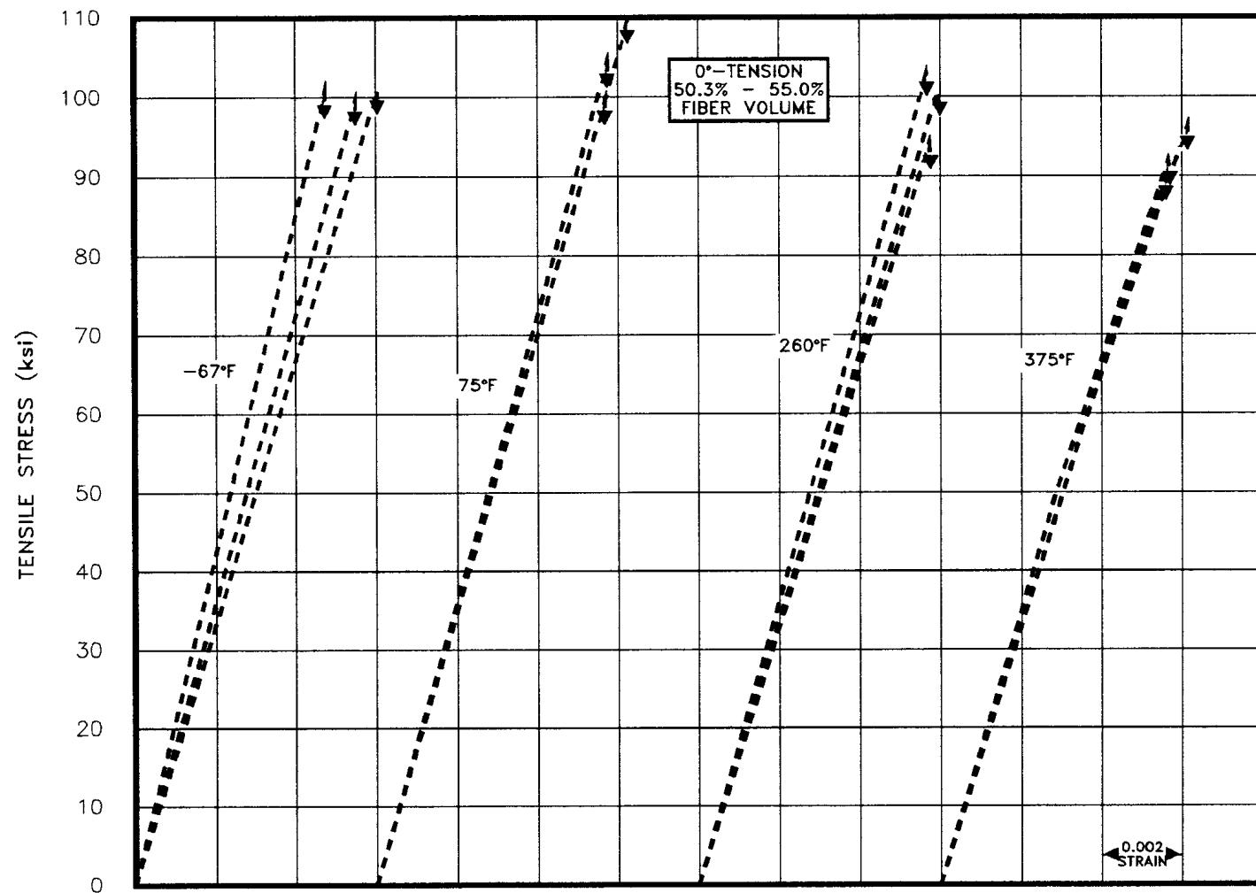
FIGURE A1.111.1(a) Tensile stress-strain for AVCO 5505 boron/epoxy ( $0^\circ$  -  $90^\circ$  crossply) loaded in the  $0^\circ$  direction. Individual tests shown.
