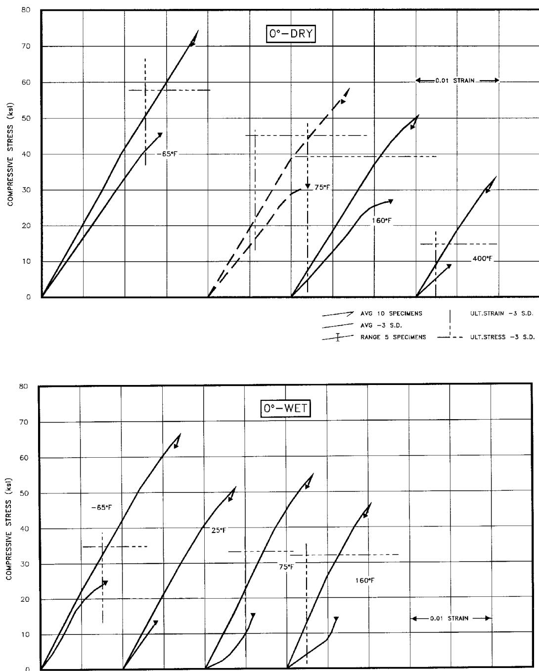
**FIGURE A1.5.2(a)** Compressive stress-strain for F-161/7781 fiberglass epoxy loaded in the 0° direction (31% resin).
