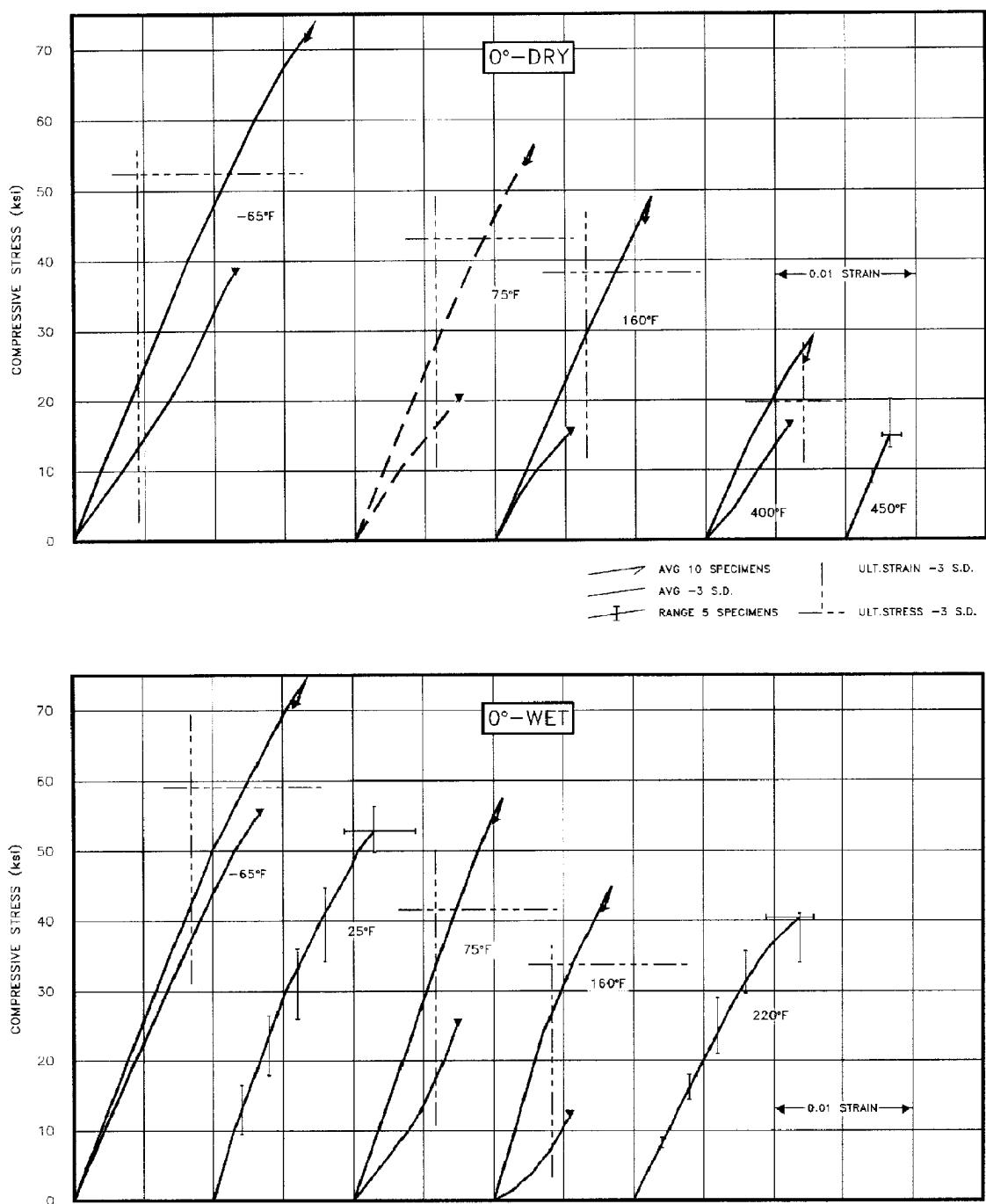
**FIGURE A1.4.2(a)** Compressive stress-strain for F-161/7781 fiberglass epoxy loaded in the 0° direction (26% resin.)
