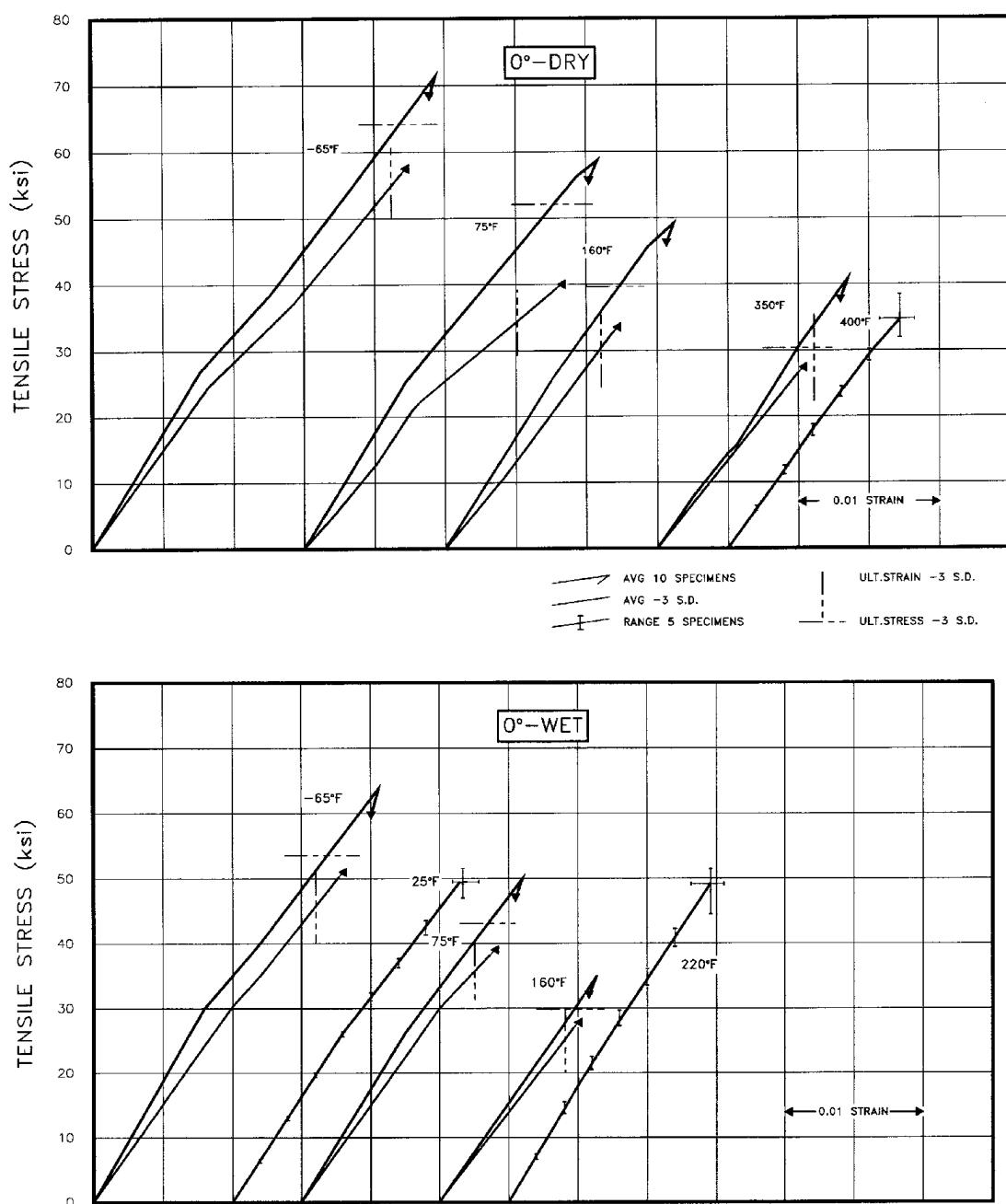
**FIGURE A1.8.1(a)** Tensile stress-strain for N588/7781 fiberglass epoxy loaded in the 0° direction.
