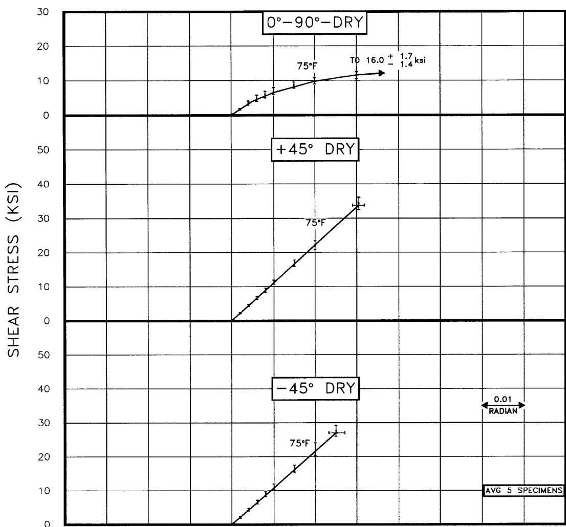
**FIGURE A1.8.3** Rail shear for N588/7781 fiberglass epoxy.
