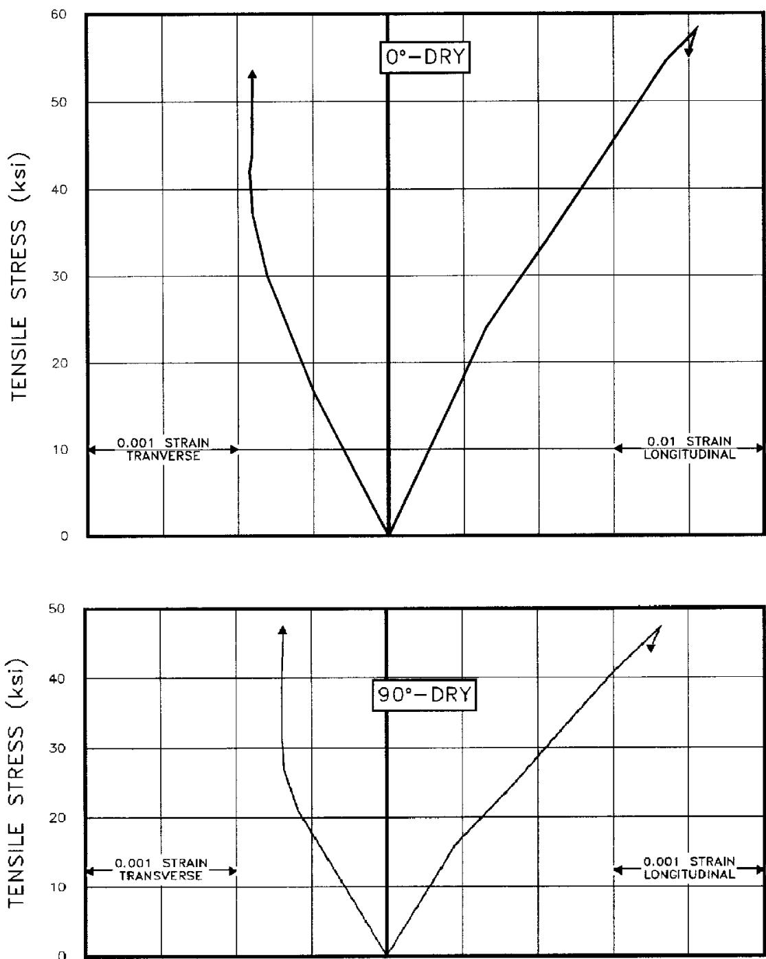
FIGURE A1.8.4 Poisson effects for N588/7781 fiberglass epoxy.
