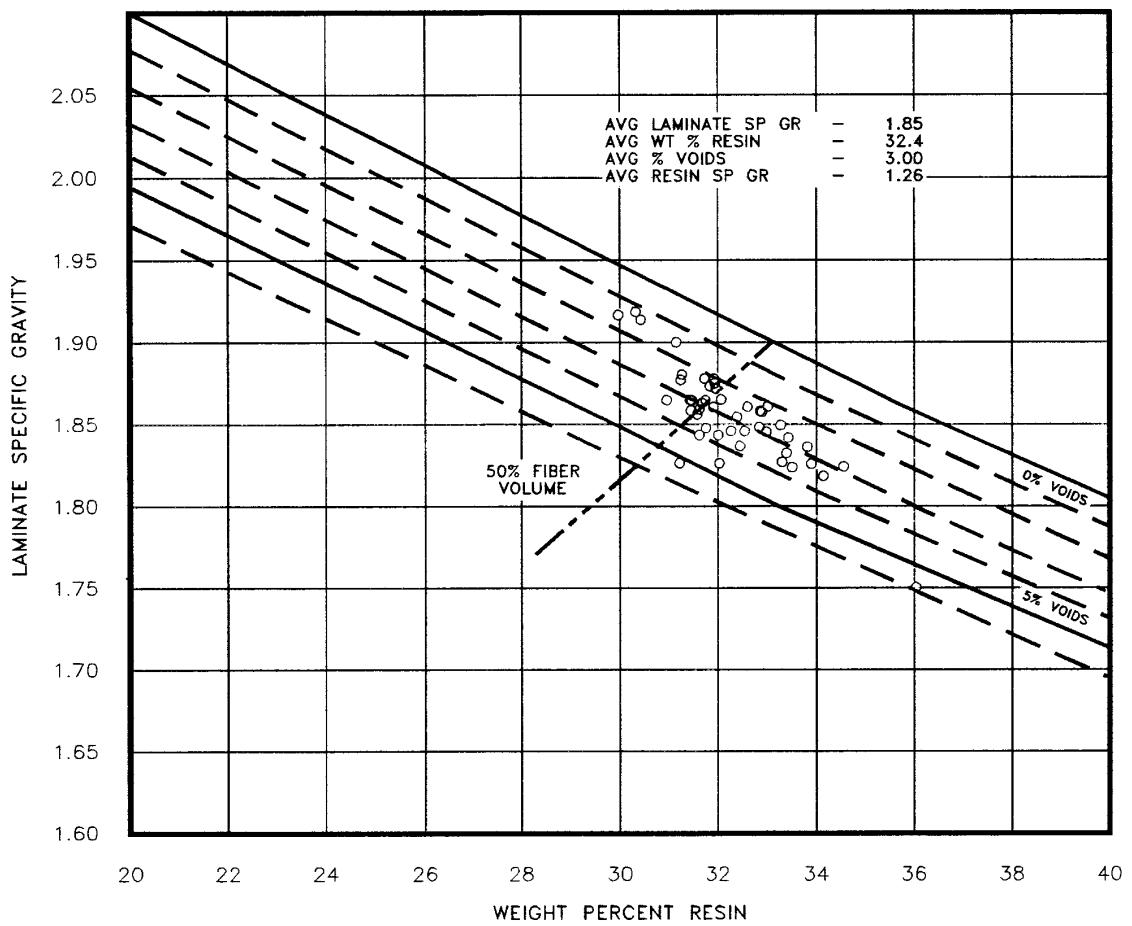
**FIGURE A1.3.5** Voids vs. resin content and specific gravity for F-161/7743 fiberglass epoxy.
