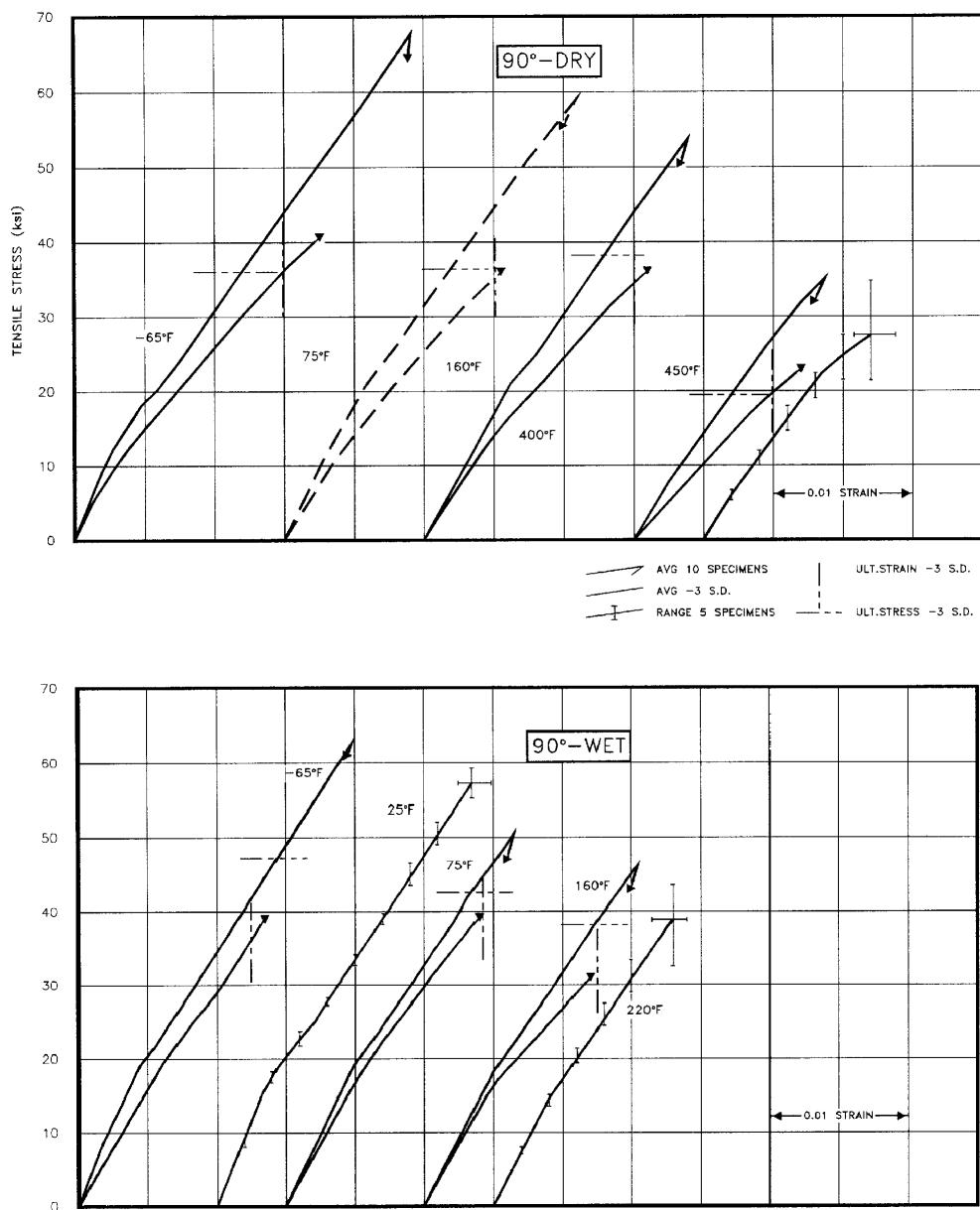
**FIGURE 1.4.1(b)** Tensile stress-strain for F-161/7781 fiberglass epoxy loaded in the 90° direction (26% resin).
