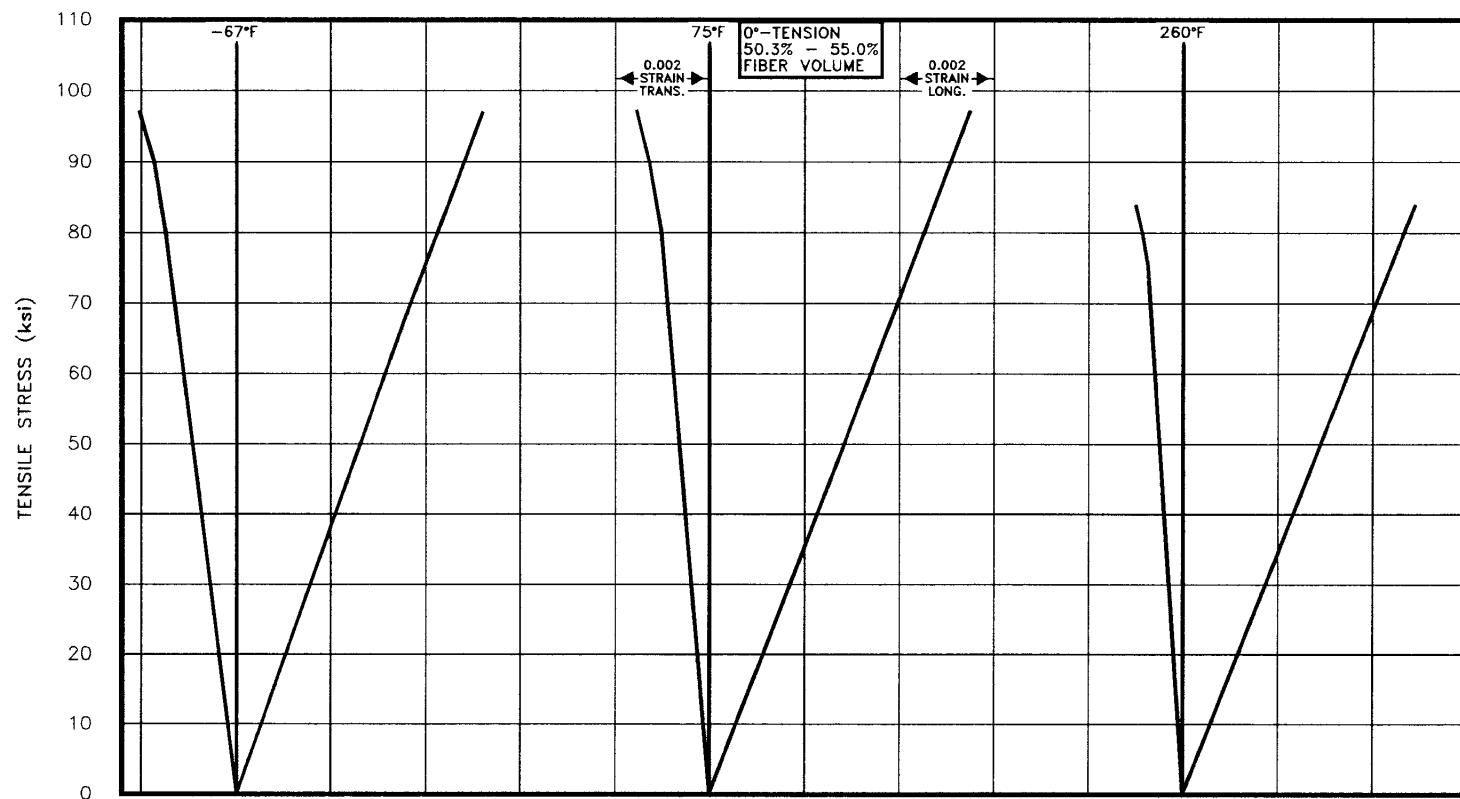
FIGURE A1.111.3 Poisson effects for AVCO 5505 boron/epoxy (0° - 90° crossply).
