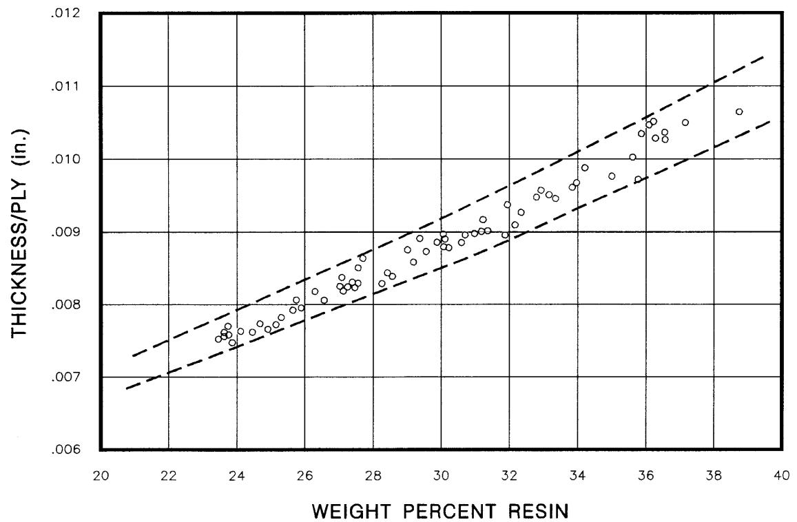
**FIGURE A1.6.6** Thickness vs. resin content for F-161/7781 fiberglass epoxy.
