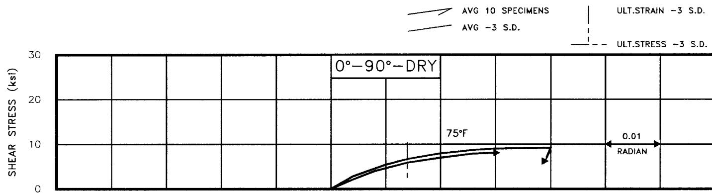
FIGURE A1.3.3  $0^\circ$  -  $90^\circ$  rail shear for F-161/7743 fiberglass epoxy.
