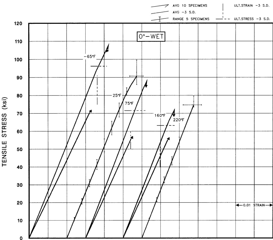
**FIGURE A1.3.1(a)** Tensile stress-strain for F-161/7743 fiberglass epoxy loaded in the  $0^\circ$  direction, continued on next page.
