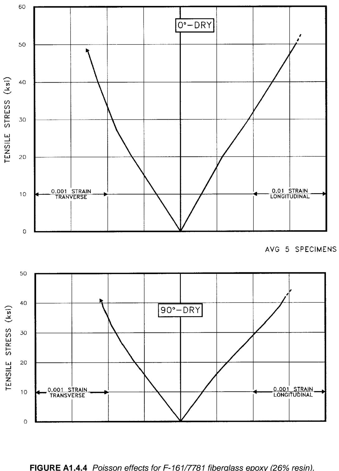
**FIGURE A1.4.4** Poisson effects for F-161/7781 fiberglass epoxy (26% resin).
