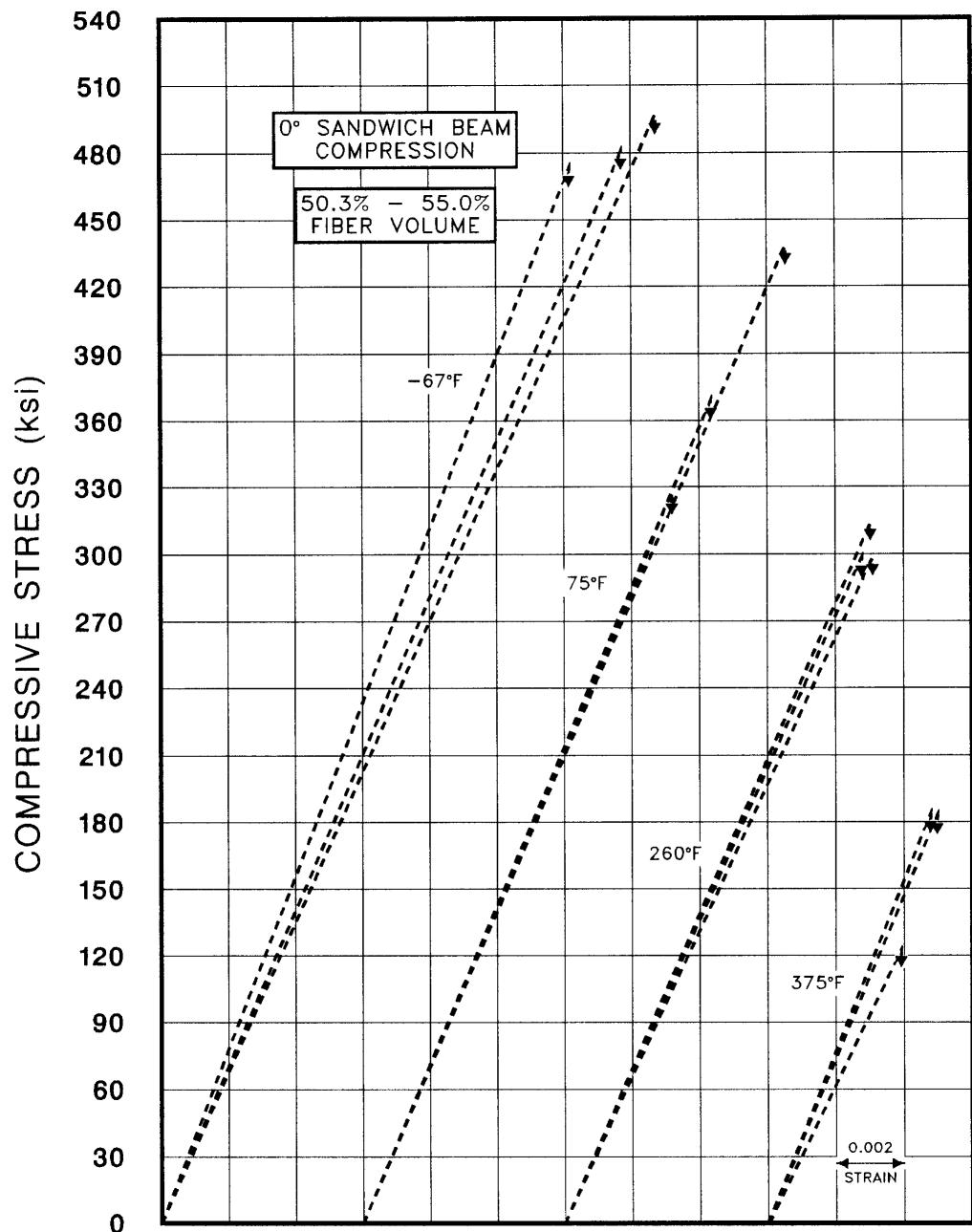
**FIGURE A1.110.2** Compressive stress-strain for AVCO 5505 boron/epoxy (100% - 0° orientation loaded in the 0° direction. Individual tests shown.
