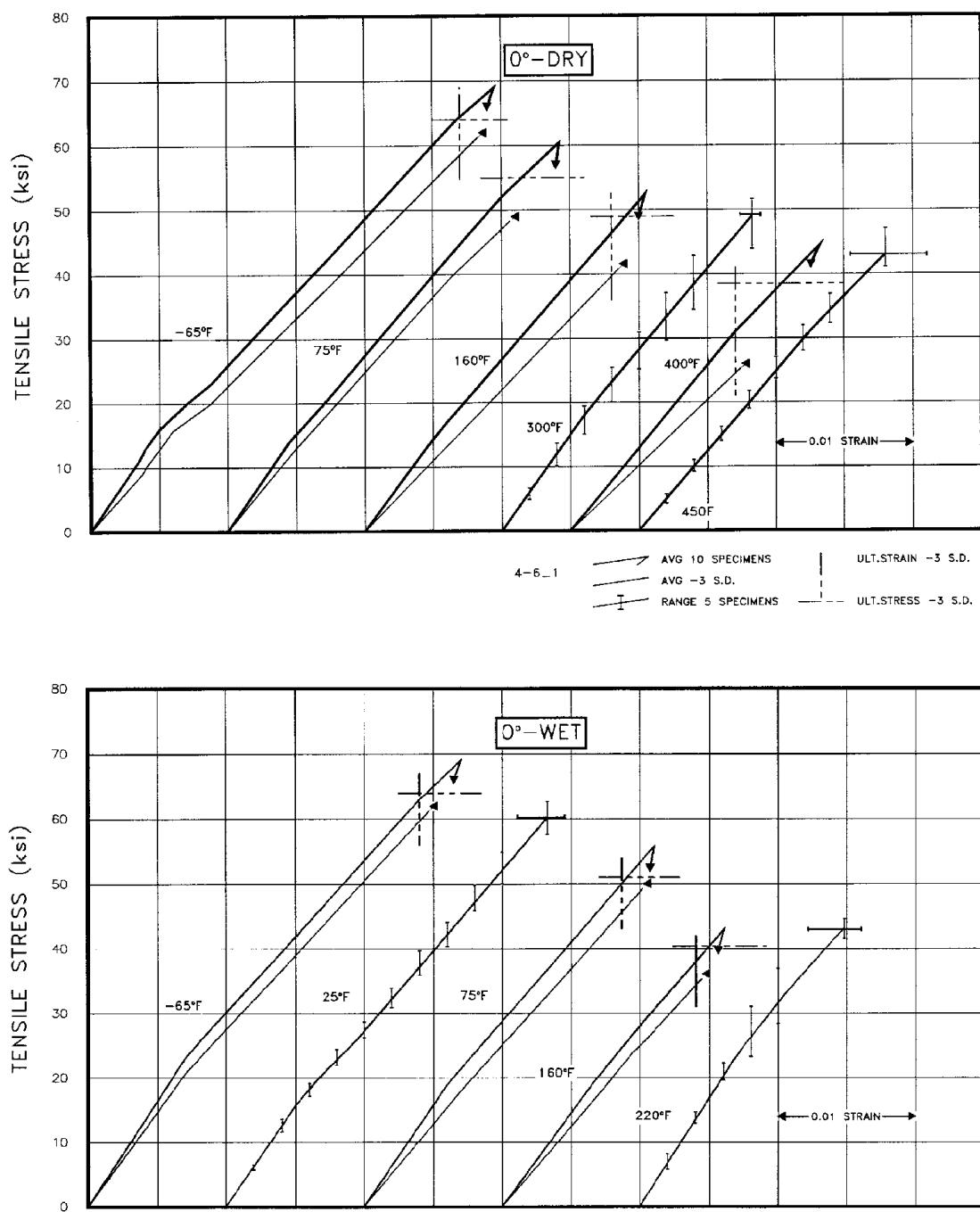
**FIGURE A1.1.1(a)** Tensile stress-strain for E-720E/7781 fiberglass epoxy loaded in the 0° direction.
