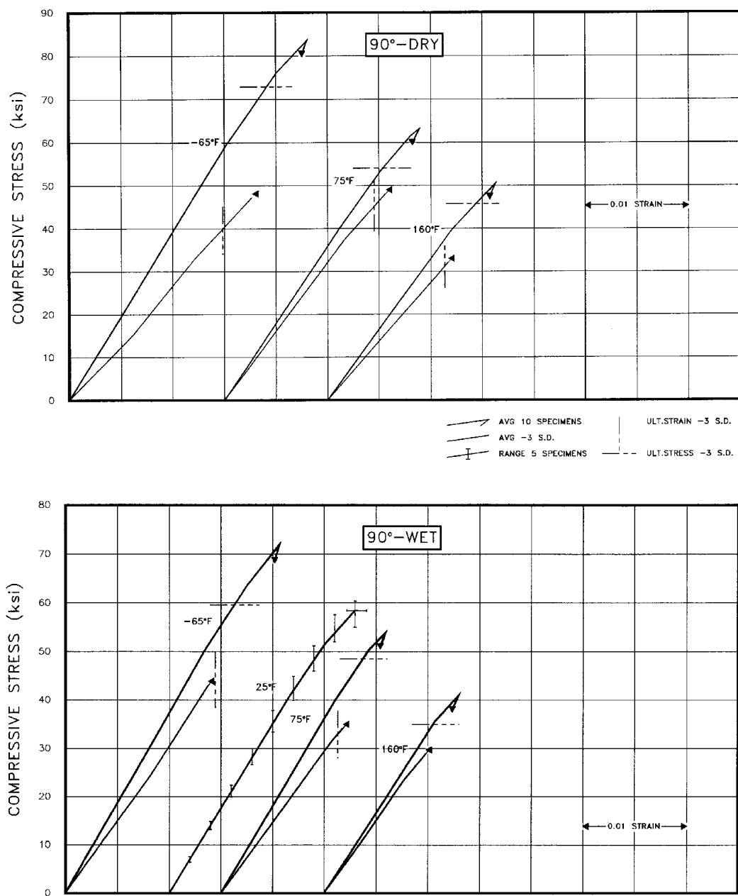
**FIGURE A1.8.2(b)** Compressive stress-strain for N588/7781 fiberglass epoxy loaded in the 90° direction.
