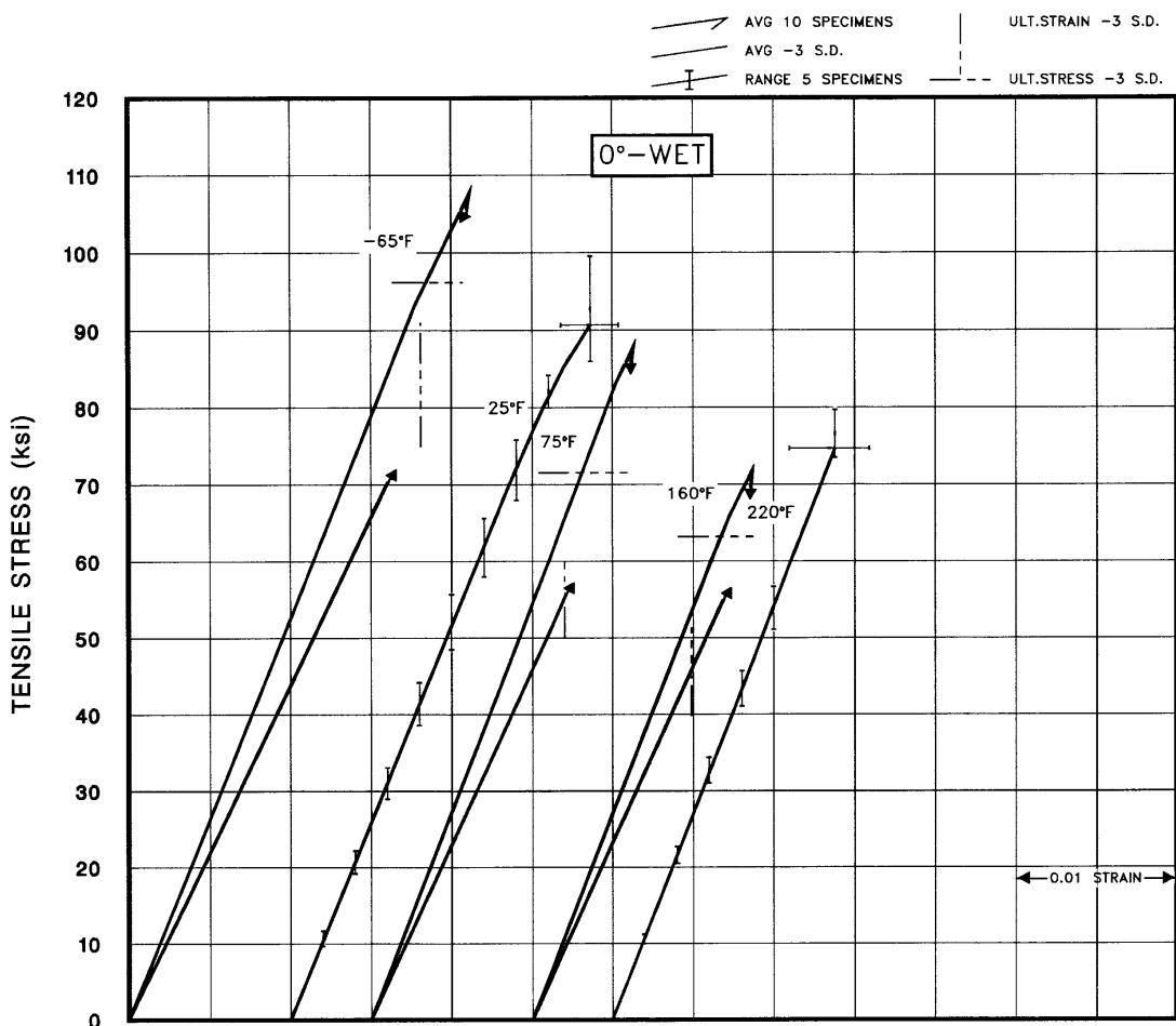
**FIGURE A1.3.1(a)** Tensile stress-strain for F-161/7743 fiberglass epoxy loaded in the  $0^\circ$  direction, concluded.
