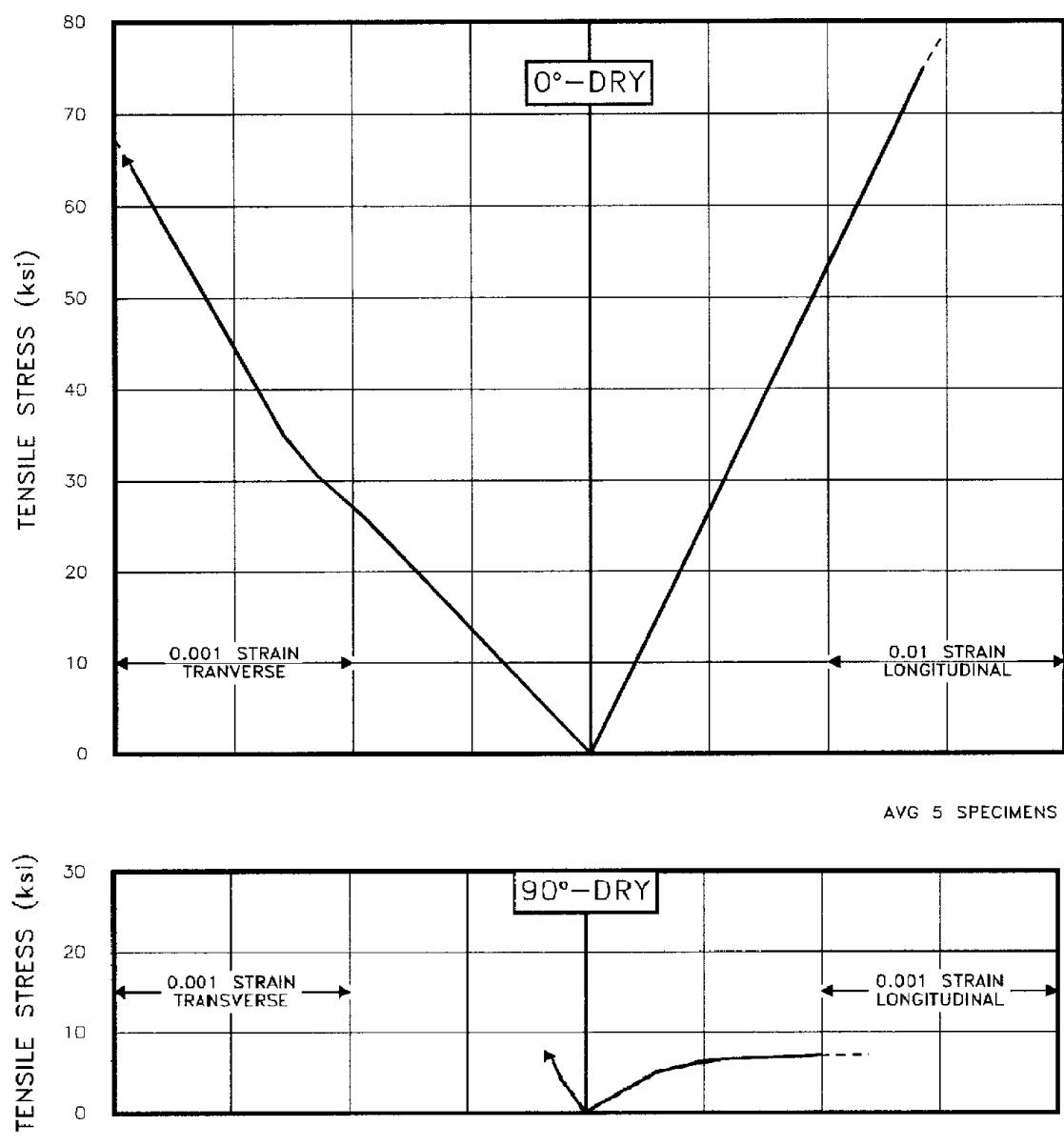
**FIGURE A1.3.4** Poisson effects for F-161/7743 fiberglass epoxy.
