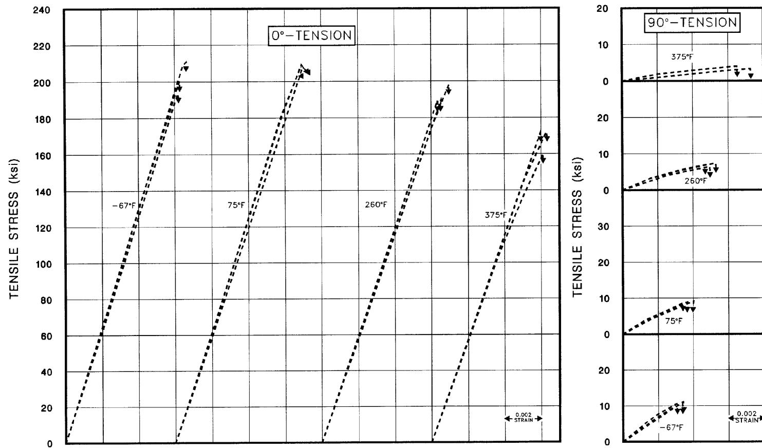
**FIGURE A1.110.1** Tensile stress-strain for AVCO 5505 boron/epoxy (100% - 0° orientation/50.3% to 35% fiber volume) loaded in the 0° and 90° directions. Individual tests shown.
