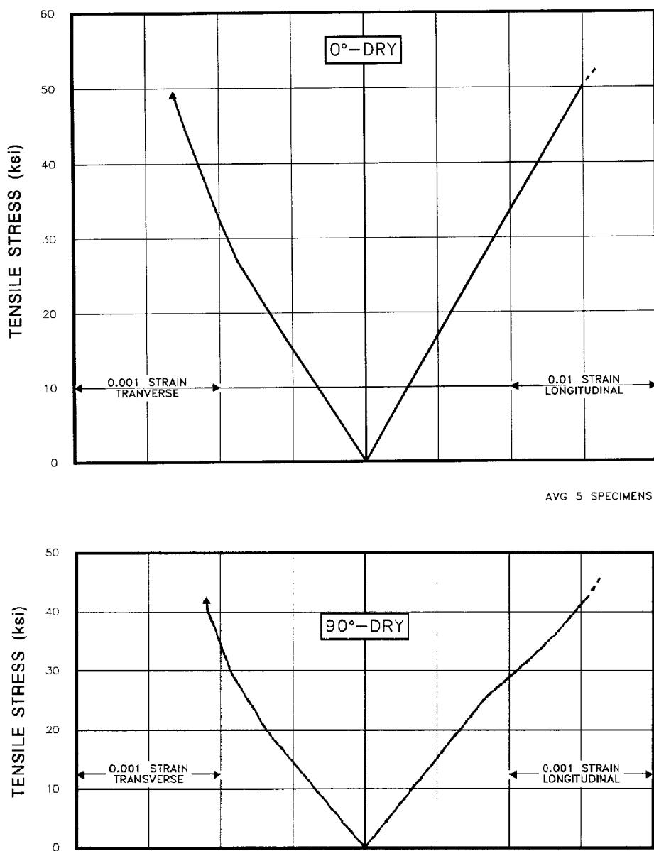
**FIGURE A1.5.4** Poisson effects for F-161/7781 fiberglass epoxy (31% resin).
