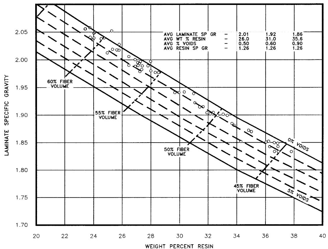
**FIGURE A.1.6.5** Voids vs. resin content and specific gravity for F-161/7781 fiberglass epoxy (26%, 31%, 36% resin).
