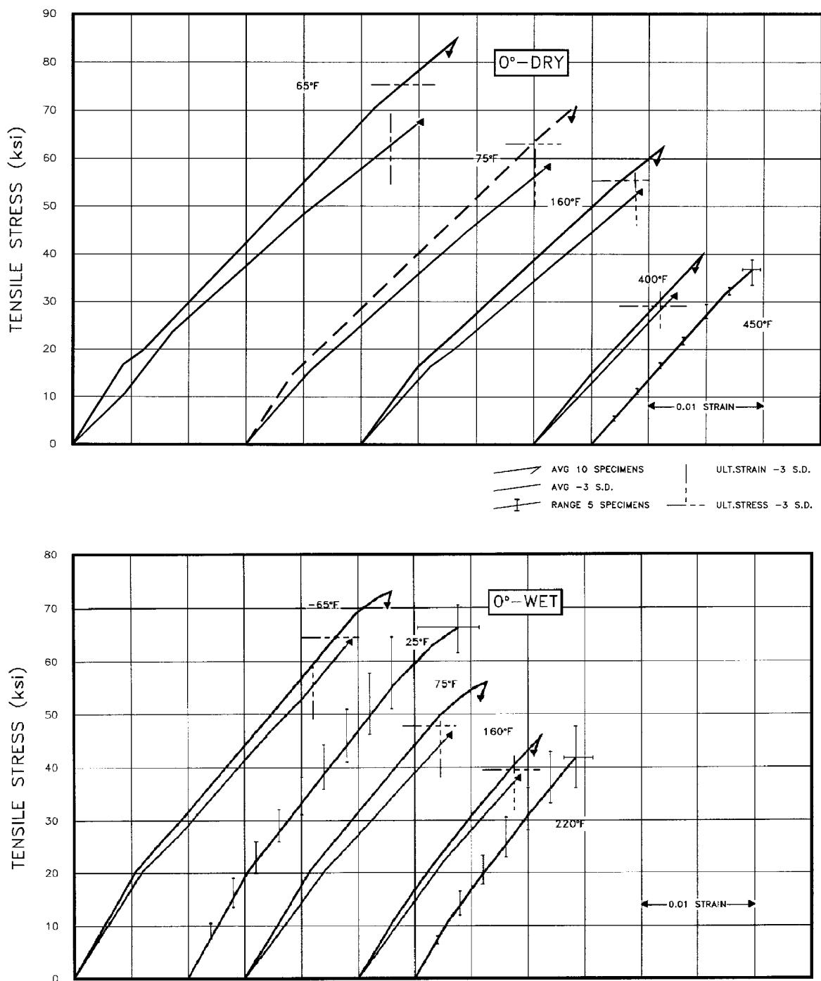
**FIGURE A.1.6.1(a)** Tensile stress-strain for F-161/7781 fiberglass epoxy loaded in the 0° direction (36% resin).
