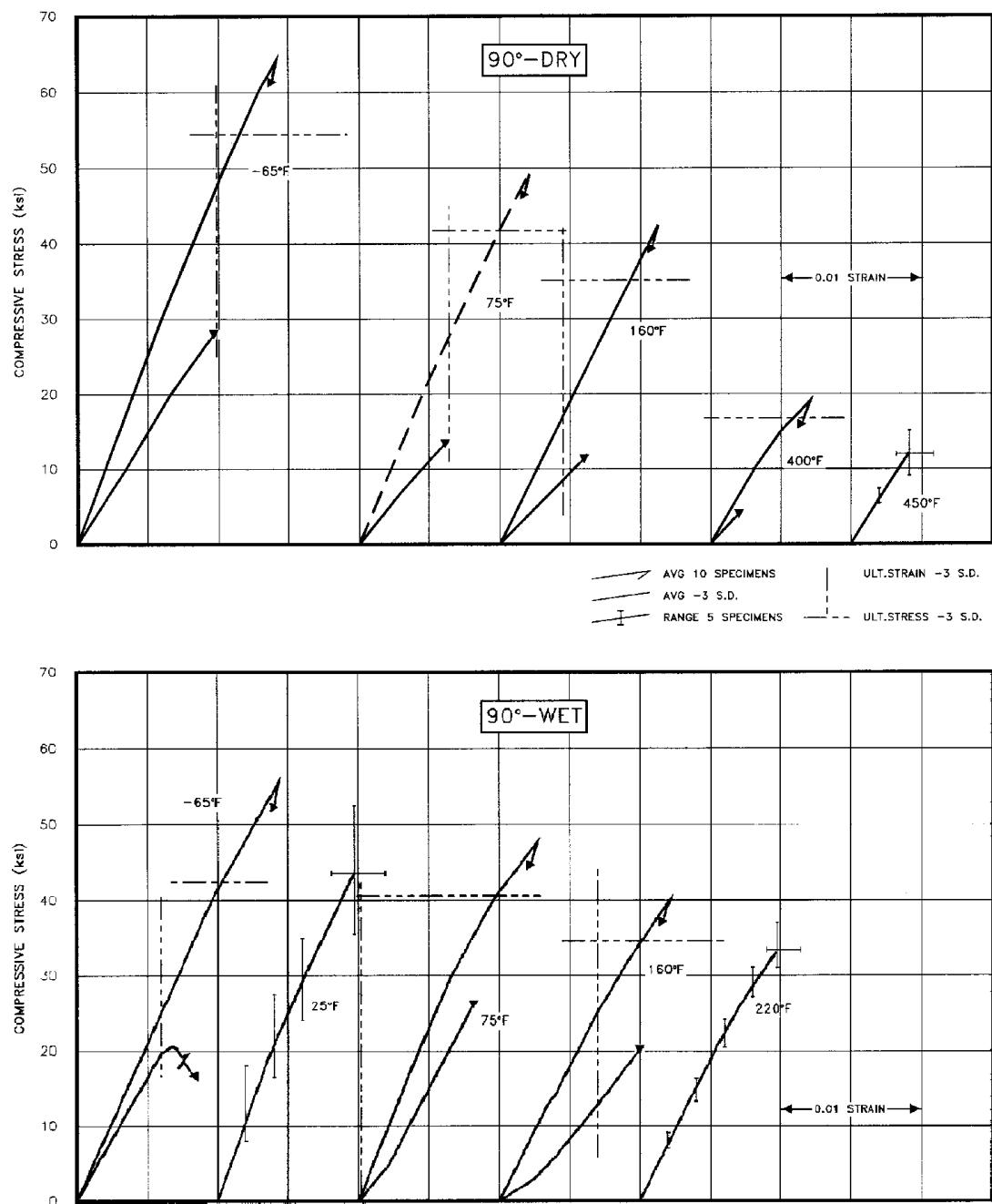
**FIGURE A1.4.2(b)** Compressive stress-strain for F-161/7781 fiberglass epoxy loaded in the 90° direction (26% resin).
