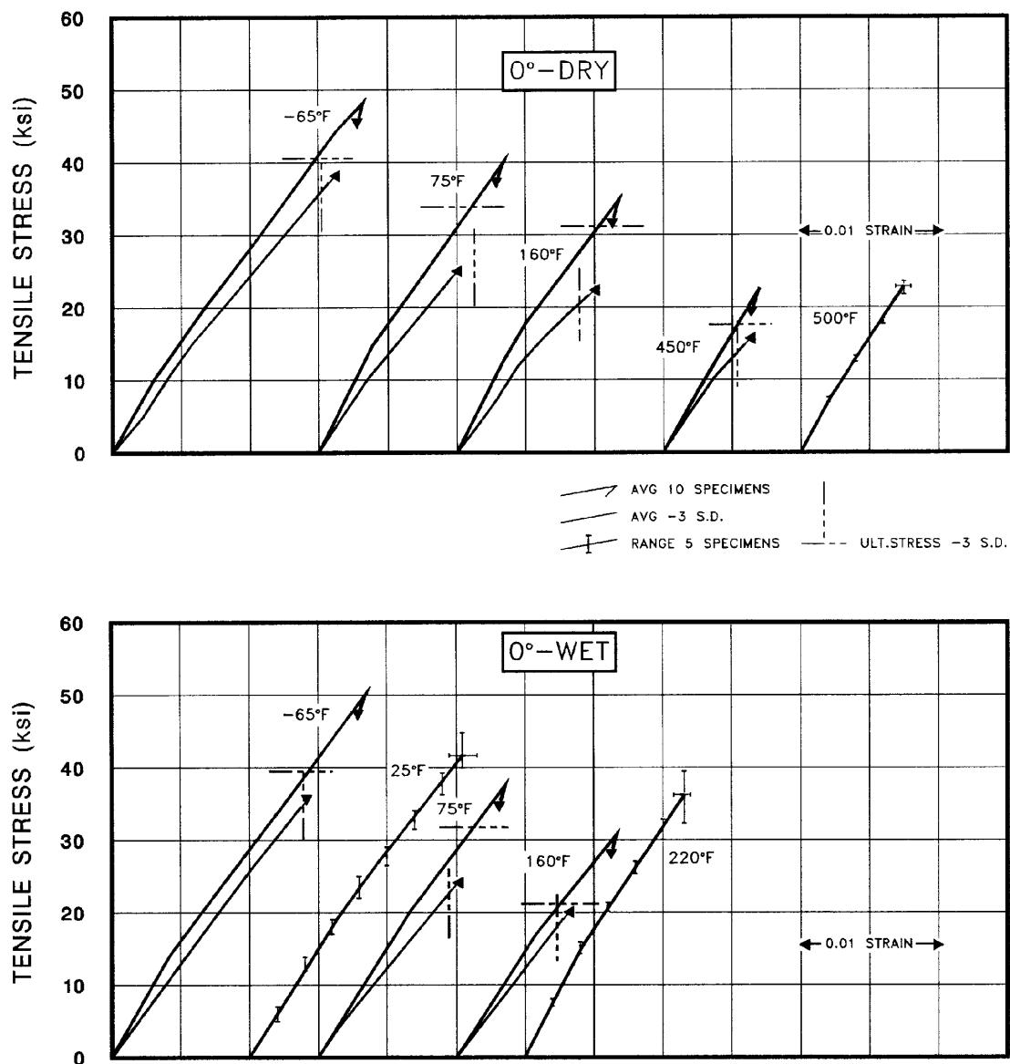
**FIGURE A1.40.1(a)** Tensile stress-strain for N506/7781 fiberglass phenolic loaded in the 0° direction.
