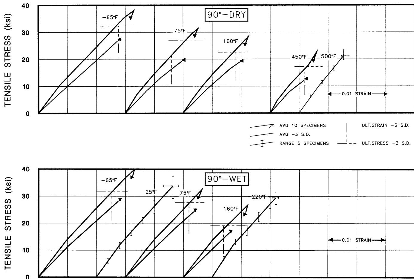
**FIGURE A1.40.1(b)** Tensile stress-strain for N506/7781 fiberglass phenolic loaded in the 90° direction.
