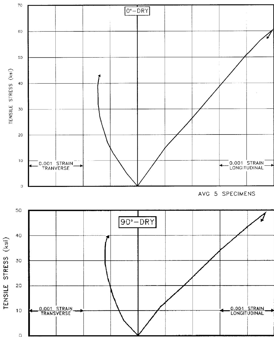
**FIGURE A1.1.4** Poisson effects for E-720E/7781 fiberglass epoxy.
