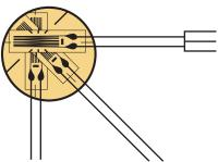
(b) Three-element strain-gage rosettes prewired
