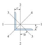
TABLE E-4(b) PROPERTIES OF ANGLE SECTIONS WITH EQUAL LEGS (L SHAPES) – SI UNITS (ABRIDGED LIST)
