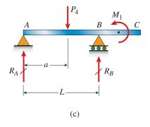
**FIG. 4-2c** Beam with an overhang. (Repeated)
