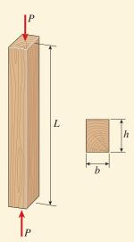
**FIG. 11-40** Example 11-8. Wood post in compression
