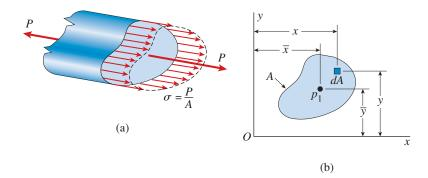
**FIG. 1-4** Uniform stress distribution in a prismatic bar: (a) axial forces P, and (b) cross section of the bar
