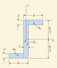
FIG. 12-23 Example 12-6. Product of inertia of a Zection
