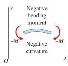
**FIG. 5-10** Relationships between signs of bending moments and signs of curvatures
