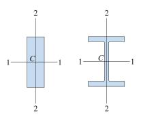
FIG. 11-9 Cross sections of columns showing principal centroidal axes with  $I_1 > I_2$
