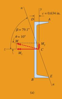
FIG. 6-24 (a) Solution to Example 6-6
