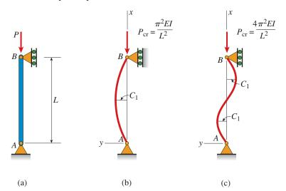
**FIG. 11-8** Buckled shapes for an ideal column with pinned ends: (a) initially straight column, (b) buckled shape for n = 1, and (c) buckled shape for n = 2
