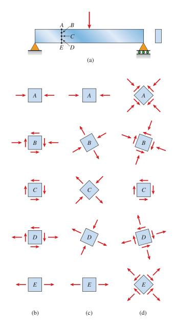
FIG. 8-13 Stresses in a beam of rectangular cross section: (a) simple beam with points A, B, C, D, and E on the side of the beam; (b) normal and shear stresses acting on stress elements at points A, B, C, D, and E; (c) principal stresses; and (d) maximum shear stresses
