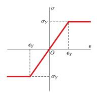
**FIG. 6-38** Idealized stress-strain diagram for an elastoplastic material
