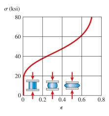
**FIG. 1-17** Stress-strain diagram for copper in compression
