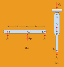
**FIG. 2-12** Example 2-3. Change in length of a nonuniform bar (bar *ABC*)
