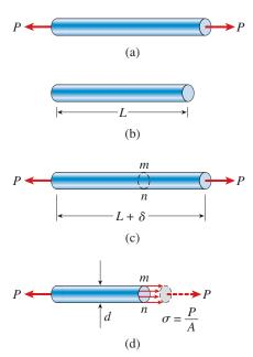
FIG. 1-2 Prismatic bar in tension:
