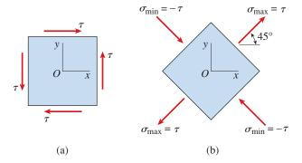
**FIG. 3-23** Stress elements oriented at  $\theta = 0$  and  $\theta = 45$  for pure shear
