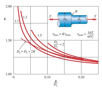
FIG. 3-48 Stress-concentration factor K for a stepped shaft in torsion. (The dashed line is for a full quarter-circular fillet.)
