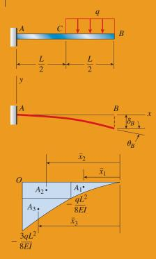
**FIG. 9-25** Example 9-11. Cantilever beam supporting a uniform load on the right-hand half of the beam
