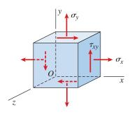
**FIG. 7-24** Element of material in plane stress ( $\sigma_z = 0$ )
