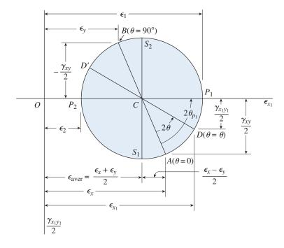
Since each gage measures the normal strain in only one direction, and since the directions of the principal stresses are usually unknown, it is necessary to use three gages in combination, with each gage measuring the strain in a different direction. From three such measurements, it is possible to calculate the strains in any direction, as illustrated in Example 7-8.
