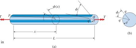
**FIG. 3-3** Deformations of a circular bar in pure torsion
