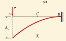
**FIG. 9-29** Example 9-14. Cantilever beam with two different moments of inertia
