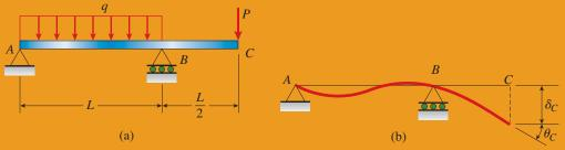
**FIG. 9-42** Example 9-18. Beam with an overhang
