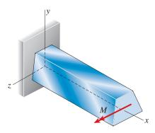
FIG. 6-39 Beam of elastoplastic material subjected to a positive bending moment *M*
