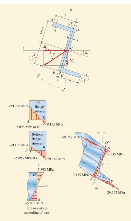
**FIG. 6-25** (a) Z-section subjected to bending moment M at angle  $\theta$  to Z axis (b) Normal stress distribution in Z-section
