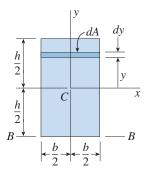
FIG. 12-10 Moments of inertia of a rectangle
