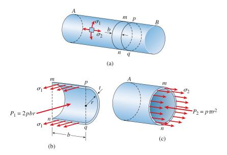
**FIG. 8-7** Stresses in a circular cylindrical pressure vessel
