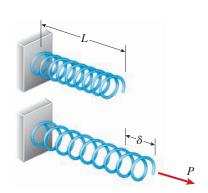
**FIG. 2-2** Elongation of an axially loaded spring
