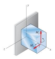
**FIG. 6-13** Sign conventions for bending moments  $M_v$  and  $M_z$
