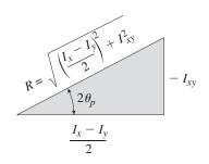
**FIG. 12-27** Geometric representation of Eq. (12-30)
