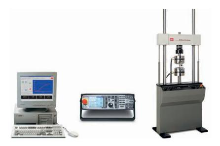
FIG. 1-7 Tensile-test machine with automatic data-processing system. (Courtesy of MTS Systems Corporation)
