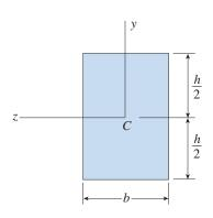
FIG. 6-42 Rectangular cross section
