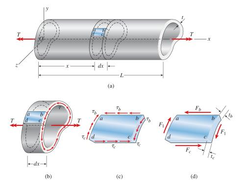
FIG. 3-40 Thin-walled tube of arbitrary cross-sectional shape
