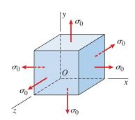
FIG. 7-29 Element in spherical stress
