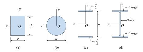
FIG. 5-18 Cross-sectional shapes of beams
