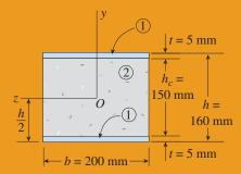
FIG. 6-8 Example 6-2. Cross section of sandwich beam having aluminum-alloy faces and a plastic core
