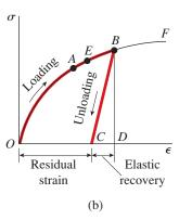
FIG. 1-18 Stress-strain diagrams illustrating (a) elastic behavior, and (b) partially elastic behavior
