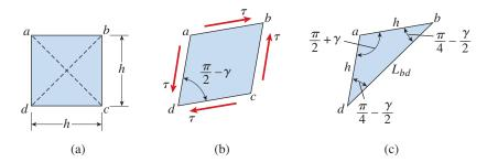
FIG. 3-28 Geometry of deformed element in pure shear
