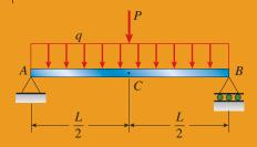
**FIG. 9-40** Example 9-17. Simple beam with two loads
