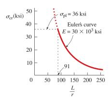
**FIG. 11-10** Graph of Euler's curve (from Eq. 11-16) for structural steel with  $E = 30 \times 10^3$  ksi and  $\sigma_{\rm pl} = 36$  ksi
