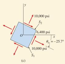
**FIG. 7-21** Example 7-5 (continued). (a) Stresses acting on an element oriented at  $\theta = 40^{\circ}$ , (b) principal stresses, and (c) maximum shear stresses
