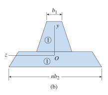
FIG. 6-9 Composite beam of two materials: (a) actual cross section, and (b) transformed section consisting only of material 1
