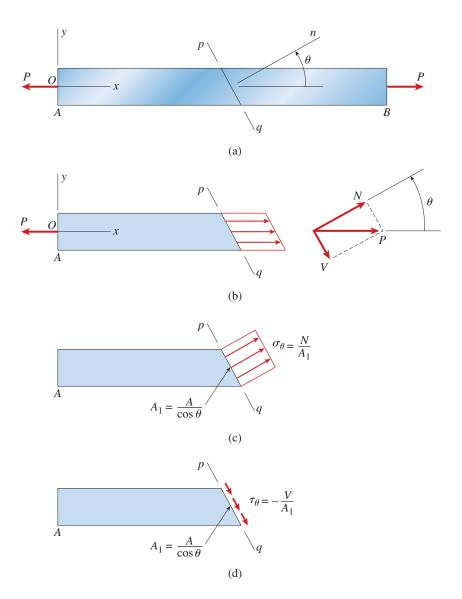
**FIG. 2-33** Prismatic bar in tension showing the stresses acting on an inclined section pq
