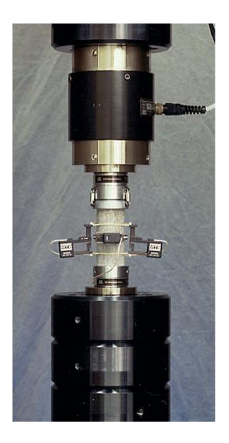
FIG. 1-9 Rock sample being tested in compression to obtain compressive strength, elastic modulus and Poisson's ratio (Courtesy of MTS Systems Corporation)
