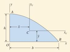
**FIG. 12-15** Example 12-4. Parallel-axis theorem
