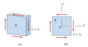
FIG. 8-23 Stress element at point B
