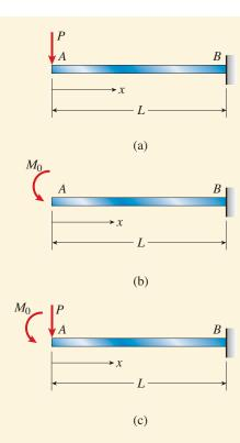
**FIG. 9-34** Example 9-16. Strain energy of a beam
