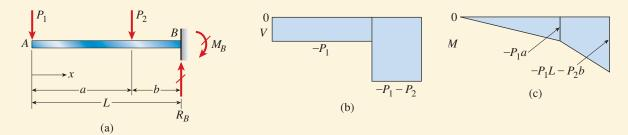
**FIG. 4-19** Example 4-5. Cantilever beam with two concentrated loads
