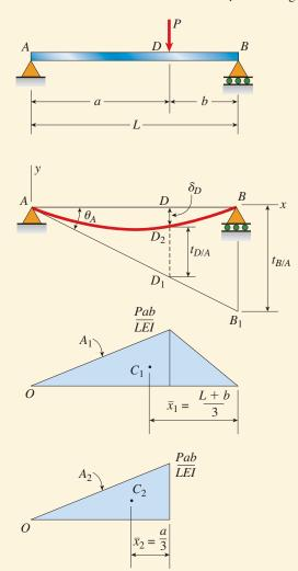
**FIG. 9-26** Example 9-12. Simple beam with a concentrated load
