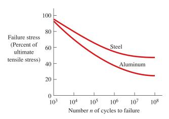
FIG. 2-59 Typical endurance curves for steel and aluminum in alternating (reversed) loading
