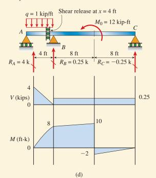
**FIG. 4-21** Example 4-7. Modified beam with overhang—add shear release.
