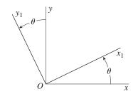
**FIG. 7-32** Axes  $x_1$  and  $y_1$  rotated through an angle  $\theta$  from the xy axes
