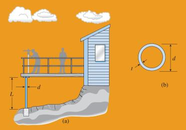
FIG. 11-20 Example 11-2. Aluminum pipe column
