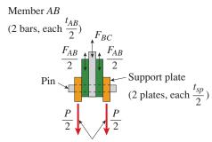
Load *P* at joint *B* is applied to the two support plates
