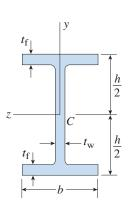
**FIG. 6-44** Cross section of a wide-flange beam
