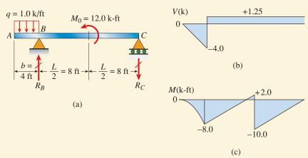
**FIG. 4-21** Example 4-7. Beam with an overhang
