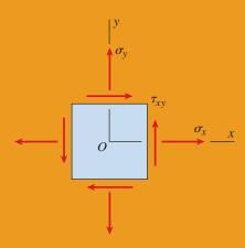
FIG. 8-30 Notation for an element in plane stress
