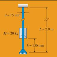
**FIG. 2-54** Example 2-16. Impact load on a vertical bar
