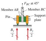
(b) Section *a–a* at joint *B* (Elevation view)
