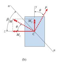
**FIG. 6-15** Doubly symmetric beam with an inclined load P acting at an angle  $\theta$  to the positive y axis
