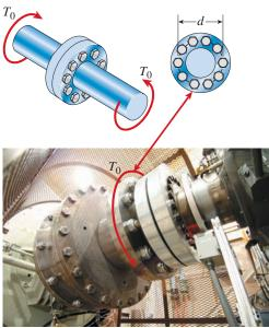
Drive shaft coupling on a ship propulsion motor
