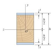
FIG. 6-4 Doubly symmetric cross section
