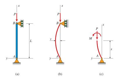
**FIG. 11-5** Column with pinned ends: (a) ideal column, (b) buckled shape, and (c) axial force *P* and bending moment *M* acting at a cross section
