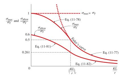
**FIG. 11-34** Design formulas for structural-steel columns
