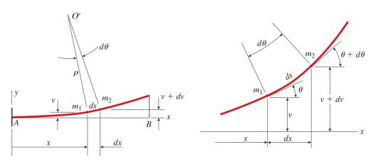
FIG. 9-2 Deflection curve of a beam
