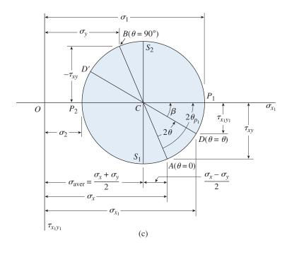
$\sigma_{x_1} = \sigma_y$  and  $\tau_{x_1y_1} = -\tau_{xy}$ . Note that point *B* on the circle corresponds to  $\theta = 90^\circ$ . In addition, the *y* face of the element (Fig. 7-16a) is labeled "*B*" to show its correspondence with point *B* on the circle.
