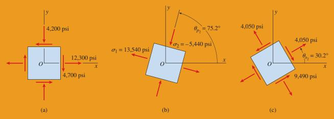
FIG. 7-14 Example 7-3. (a) Element in plane stress, (b) principal stresses, and (c) maximum shear stresses
