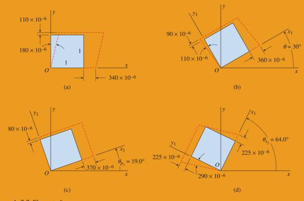
FIG. 7-37 Example 7-7. Element of material in plane strain: (a) element oriented to the x and y axes, (b) element oriented at an angle  $\theta = 30^{\circ}$ , (c) principal strains, and (d) maximum shear strains. (*Note:* The edges of the elements have unit lengths.)
