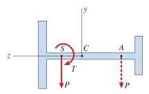
**FIG. 6-27** Singly symmetric beam with load *P* applied at point *A*
