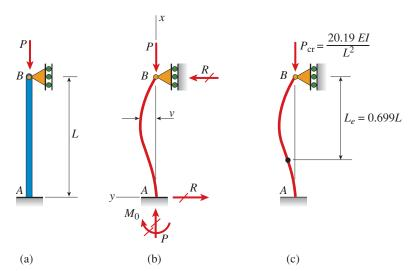
FIG. 11-18 Column fixed at the base and pinned at the top
