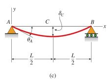
**FIG. 9-17** Simple beam with a triangular load
