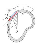
FIG. 3-41 Cross section of thin-walled tube
