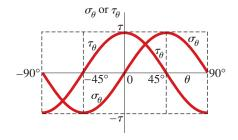
**FIG. 3-22** Graph of normal stresses  $\sigma_{\theta}$  and shear stresses  $\tau_{\theta}$  versus angle  $\theta$  of the inclined plane
