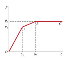
**FIG. 2-74** Load-displacement diagram for the statically indeterminate structure shown in Fig. 2-73
