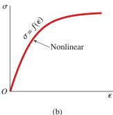
FIG. 2-66 Types of idealized material behavior: (a) elastic-nonlinear stress-strain curve, (b) general nonlinear stress-strain curve, (c) elastoplastic stress-strain curve, and (d) bilinear stress-strain curve
