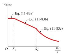
FIG. 11-35 Design formulas for aluminum columns
