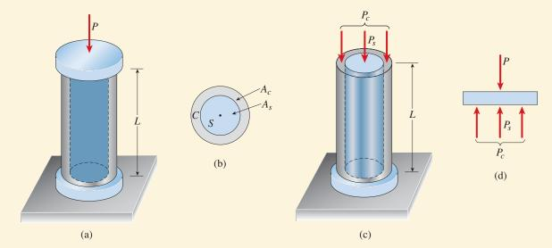
**FIG. 2-17** Example 2-5. Analysis of a statically indeterminate structure
