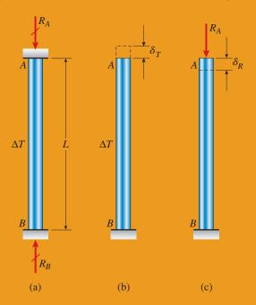
FIG. 2-23 Example 2-7. Statically indeterminate bar with uniform temperature increase  $\Delta T$
