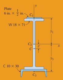
**FIG. 12-8** Example 12-2. Centroid of a composite area
