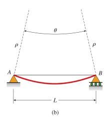
**FIG. 9-30** Beam in pure bending by couples of moment M
