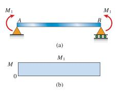
**FIG. 5-2** Simple beam in pure bending  $(M = M_1)$
