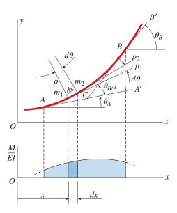
**FIG. 9-22** Derivation of the first moment-area theorem
