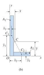
**FIG. 12-6** Centroid of a composite area consisting of two parts
