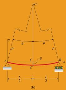
FIG. 5-8 Example 5-1. Beam in pure bending: (a) beam with loads, and (b) deflection curve
