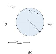
**FIG. 7-15** Two forms of Mohr's circle: (a)  $\tau_{x_1y_1}$  is positive downward and the angle  $2\theta$  is positive counterclockwise, and (b)  $\tau_{x_1y_1}$  is positive upward and the angle  $2\theta$  is positive clockwise. (*Note:* The first form is used in this book.)
