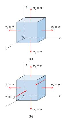
FIG. 8-4 Stresses in a spherical pressure vessel at (a) the outer surface and (b) the inner surface
