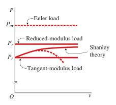
FIG. 11-33 Load-deflection diagram for elastic and inelastic buckling
