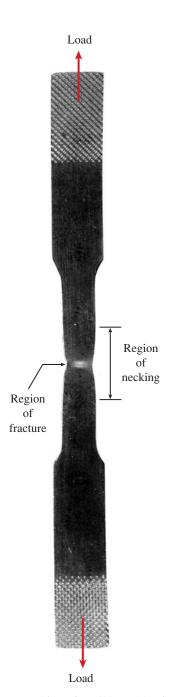
**FIG. 1-11** Necking of a mild-steel bar in tension
