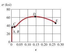
FIG. 1-12 Stress-strain diagram for a typical structural steel in tension (drawn to scale)
