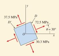
**FIG. 7-19** Example 7-4 (continued). Stresses acting on an element oriented at an angle  $\theta = 30^{\circ}$
