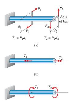
**FIG. 3-2** Circular bar subjected to torsion by torques  $T_1$  and  $T_2$
