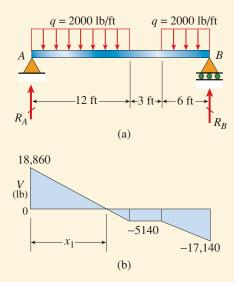
**FIG. 5-21** Example 5-7. Design of a simple beam with partial uniform loads
