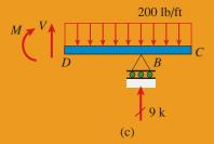
FIG. 4-13 Example 4-3. Shear force and bending moment in a beam with an overhang
