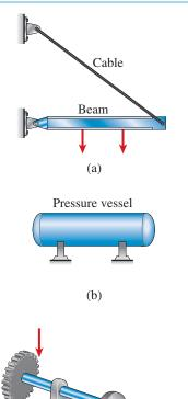
FIG. 8-20 Examples of structures subjected to combined loadings:
