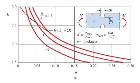
**FIG. 5-50** Stress-concentration factor K for a notched beam of rectangular cross section in pure bending (h = height of beam; b = thickness of beam, perpendicular to the plane of the figure). The dashed line is for semicircular notches ( $h = h_1 + 2R$ )
