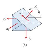
FIG. 7-27 Element in triaxial stress
