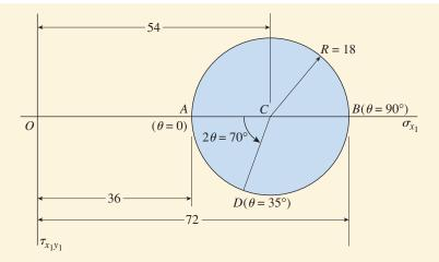
FIG. 8-11 Mohr's circle for the biaxial stress element of Fig. 8-10b. (*Note:* All stresses on the circle have units of MPa.)
