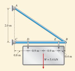
**FIG. 1-33** Example 1-8. Two-bar truss *ABC* supporting a sign of weight *W*
