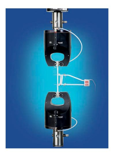
**FIG. 1-8** Typical tensile-test specimen with extensometer attached; the specimen has just fractured in tension. (Courtesy of MTS Systems Corporation)
