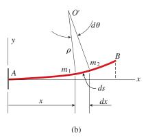
FIG. 5-5 Curvature of a bent beam:
