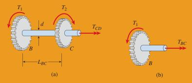
**FIG. 3-18** Free-body diagrams for Example 3-4
