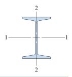
TABLE E-2(a) PROPERTIES OF I-BEAM SECTIONS (S SHAPES) – USCS UNITS (ABRIDGED LIST)
