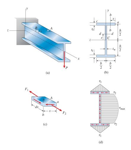
**FIG. 6-32** Shear stresses in a wide-flange beam
