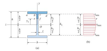
FIG. 5-38 Shear stresses in the web of a wide-flange beam. (a) Cross section of beam, and (b) distribution of vertical shear stresses in the web
