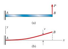
FIG. 5-1 Bending of a cantilever beam:
