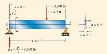
**FIG. 8-17** Example 8-3. Beam of rectangular cross section
