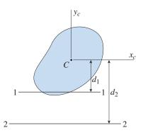
FIG. 12-14 Plane area with two parallel noncentroidal axes (axes 1-1 and 2-2)
