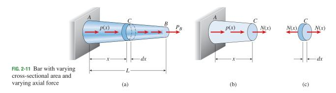
The elongation  $d\delta$  of the differential element (Fig. 2-11c) may be obtained from the equation  $\delta = PL/EA$  by substituting N(x) for P, dx for L, and A(x) for A, as follows:
