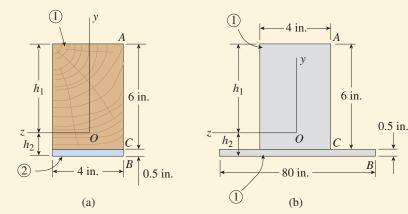
**FIG. 6-10** Example 6-3. Composite beam of Example 6-1 analyzed by the transformed-section method:
