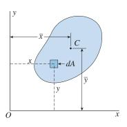
**FIG. 12-1** Plane area of arbitrary shape with centroid *C*
