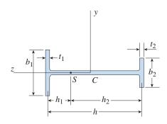
**6.9-4** The cross section of an unbalanced wide-flange beam is shown in the figure. Derive the following formula for the distance e from the centerline of the web to the shear center S:
