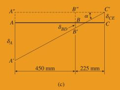
**FIG. 2-8** Example 2-2. Horizontal beam *ABC* supported by two vertical bars
