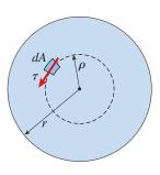
FIG. 3-9 Determination of the resultant of the shear stresses acting on a cross section
