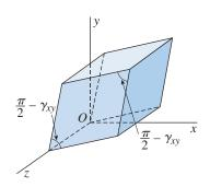
FIG. 7-26 Shear strain  $\gamma_{xy}$
