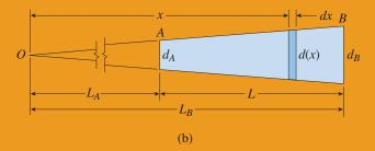
FIG. 2-13 Example 2-4. Change in length of a tapered bar of solid circular cross section
