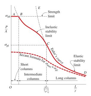
FIG. 11-29 Diagram of average compressive stress P/A versus slenderness ratio L/r
