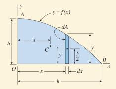
**FIG. 12-5** Example 12-1. Centroid of a parabolic semisegment
