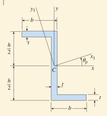
FIG. 12-28 Example 12-7. Principal axes and principal moments of inertia for a ∡ection
