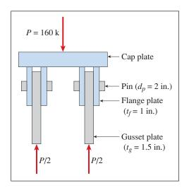
(c) Section through bottom of brace
