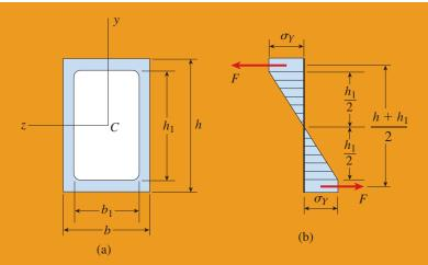
FIG. 6-48 Solution to Example 6-10
