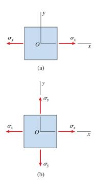
FIG. 7-11 Elements in uniaxial and biaxial stress
