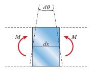
**FIG. 9-32** Side view of an element of a beam subjected to bending moments *M*
