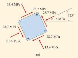
**FIG. 2-39** Example 2-10. Stresses on an inclined section
