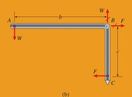
FIG. 2-7 Example 2-1. (a) Rigid L-shaped frame *ABC* attached to outer frame *BCD* by a pivot at *B*, and (b) free-body diagram of frame *ABC*
