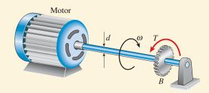
**FIG. 3-30** Example 3-7. Steel shaft in torsion
