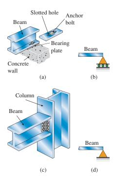
FIG. 4-3 Beam supported on a wall:
