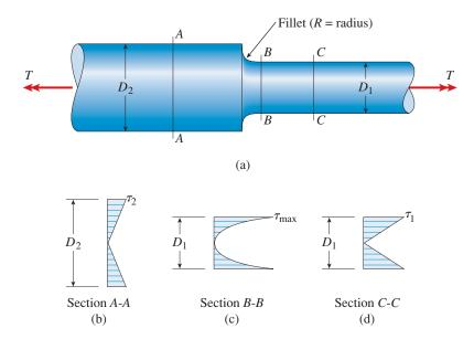
FIG. 3-47 Stepped shaft in torsion
