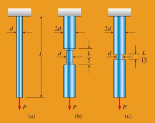
**FIG. 2-48** Example 2-12. Calculation of strain energy
