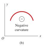
FIG. 9-3 Sign convention for curvature
