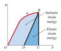
FIG. 2-43 Elastic and inelastic strain energy
