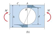
**FIG. 5-49** Stress distributions in a beam in pure bending with a circular hole at the neutral axis. (The beam has a rectangular cross section with height *h* and thickness *b*.)
