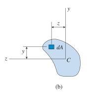
**FIG. 6-19** Unsymmetric beam subjected to a bending moment M
