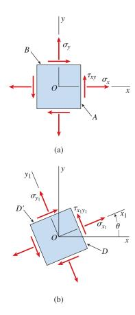
**FIG. 7-16** Construction of Mohr's circle for plane stress
