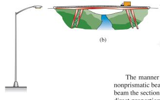
FIG. 5-23 Examples of nonprismatic beams: (a) street lamp, (b) bridge with tapered girders and piers, (c) wheel strut of a small airplane, and (d) wrench handle
