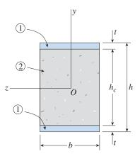
FIG. 6-5 Cross section of a sandwich beam having two axes of symmetry (doubly symmetric cross section)
