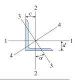
TABLE E-5(a) PROPERTIES OF ANGLE SECTIONS WITH UNEQUAL LEGS (L SHAPES) – USCS UNITS (ABRIDGED LIST)
