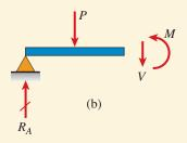
**FIG. 4-11** Example 4-1. Shear forces and bending moment in a simple beam
