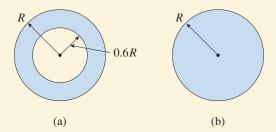
**FIG. 3-13** Example 3-3. Comparison of hollow and solid shafts
