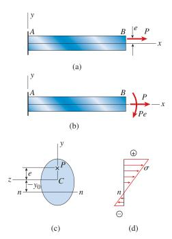
**FIG. 5-46** (a) Cantilever beam with an eccentric axial load P, (b) equivalent loads p and pe, (c) cross section of beam, and (d) distribution of normal stresses over the cross section
