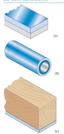
**FIG. 6-1** Examples of composite beams: (a) bimetallic beam, (b) plastic-coated steel pipe, and (c) wood beam reinforced with a steel plate
