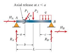
FIG. 4-5 Simple beam with axial release
