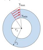
FIG. 3-5 Shear strains in a circular tube
