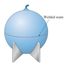
FIG. 8-1 Spherical pressure vessel
