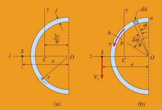
FIG. 6-37 Example 6-8. Shear center of a thin-walled semicircular section
