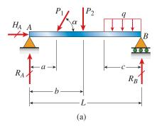
FIG. 4-2a Simple beam. (Repeated)
