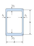
FIG. 3-43 Thin-walled rectangular tube
