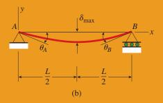
**FIG. 9-8** Example 9-1. Deflections of a simple beam with a uniform load
