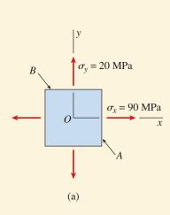
FIG. 7-18 Example 7-4. (a) Element in plane stress, and (b) the corresponding Mohr's circle. (*Note:* All stresses on the circle have units of MPa.)
