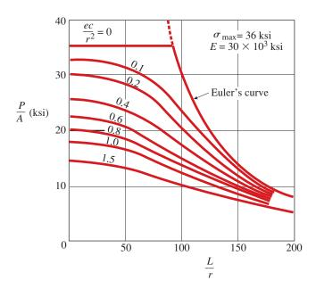
FIG. 11-27 Graph of the secant formula (Eq. 11-59) for  $\sigma_{\text{max}} = 36$  ksi and  $E = 30 \times 10^3$  ksi
