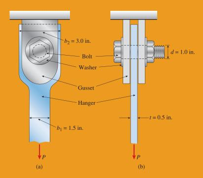
**FIG. 1-32** Example 1-7. Vertical hanger subjected to a tensile load *P*: (a) front view of bolted connection, and (b) side view of connection
