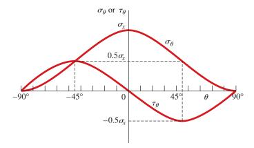
**FIG. 2-35** Graph of normal stress  $\sigma_{\theta}$  and shear stress  $\tau_{\theta}$  versus angle  $\theta$  of the inclined section (see Fig. 2-34 and Eqs. 2-29a and b)
