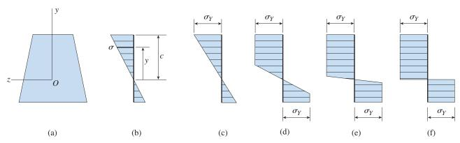
**FIG. 6-40** Stress distributions in a beam of elastoplastic material
