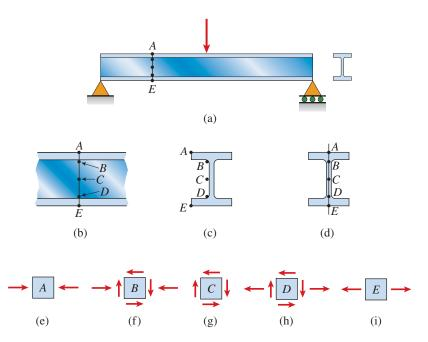
FIG. 8-16 Stresses in a wide-flange beam
