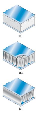
**FIG. 6-2** Sandwich beams with: (a) plastic core, (b) honeycomb core, and (c) corrugated core
