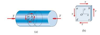
FIG. 3-20 Stresses acting on a stress element cut from a bar in torsion (pure shear)
