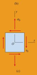
FIG. 8-24 Example 8-4. Rotor shaft of a helicopter (combined torsion and axial force)
