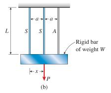
**\*2.4-13** A horizontal rigid bar of weight W = 7200 lb is supported by three slender circular rods that are equally spaced (see figure). The two outer rods are made of aluminum ( $E_1 = 10 \times 10^6$  psi) with diameter  $d_1 = 0.4$  in. and length  $L_1 = 40$  in. The inner rod is magnesium ( $E_2 = 6.5 \times 10^6$  psi) with diameter  $d_2$  and length  $L_2$ . The allowable stresses in the aluminum and magnesium are 24,000 psi and 13,000 psi, respectively.
