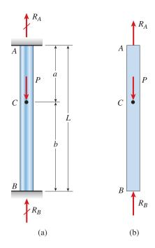
**FIG. 2-16** Analysis of a statically indeterminate bar
