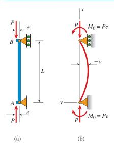
FIG. 11-21 Column with eccentric axial loads
