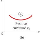
**FIG. 6-20** Sign conventions for curvatures  $\kappa_y$  and  $\kappa_z$  in the xy and xz planes, respectively
