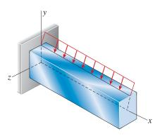
**FIG. 6-12** Doubly symmetric beam with an inclined load
