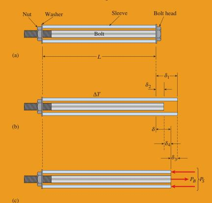
FIG. 2-24 Example 2-8. Sleeve and bolt assembly with uniform temperature increase  $\Delta T$
