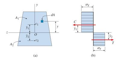
FIG. 6-41 Location of the neutral axis and determination of the plastic moment  $M_P$  under fully plastic conditions
