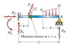
FIG. 4-6 Propped cantilever beam with moment release
