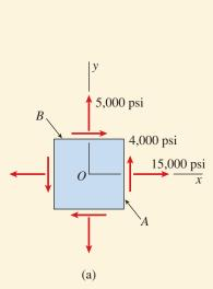
**FIG. 7-20** Example 7-5. (a) Element in plane stress, and (b) the corresponding Mohr's circle. (*Note:* All stresses on the circle have units of psi.)
