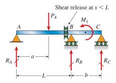
FIG. 4-7 Modified beam with overhang—add shear release
