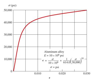
FIG. 2-68 Stress-strain curve for an aluminum alloy using the Ramberg-Osgood equation (Eq. 2-72)
