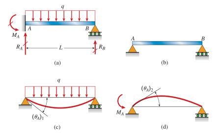
FIG. 10-13 Analysis of a propped cantilever beam by the method of superposition with the moment reaction  $M_A$  selected as the redundant
