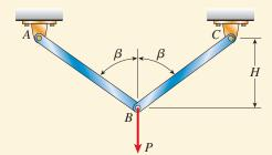
**FIG. 2-50** Example 2-14. Displacement of a truss supporting a single load *P*
