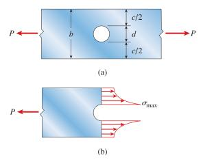
FIG. 2-62 Stress distribution in a flat bar with a circular hole
