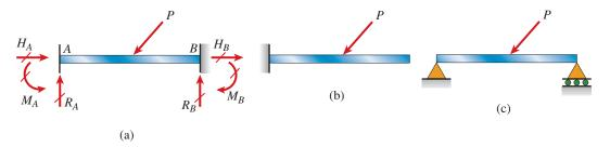
FIG. 10-3 Fixed-end beam: (a) beam with load and reactions; (b) released structure when the three reactions at end *B* are selected as the redundants; and (c) released structure when the two moment reactions and the horizontal reaction at end *B* are selected as the redundants
