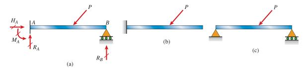
FIG. 10-1 Propped cantilever beam:
