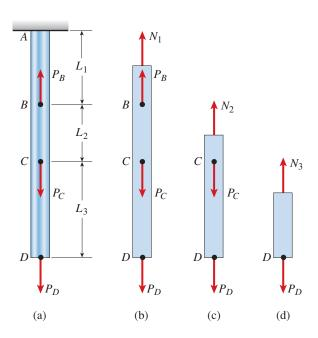
**FIG. 2-9** (a) Bar with external loads acting at intermediate points; (b), (c), and (d) free-body diagrams showing the internal axial forces  $N_1$ ,  $N_2$ , and  $N_3$
