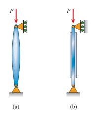
FIG. 11-12 Nonprismatic columns
