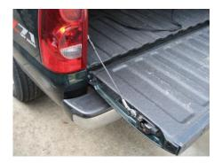
**1.2-10** Solve the preceding problem if the mass of the tail gate is  $M_T = 27$  kg and that of the crate is  $M_C = 68$  kg. Use dimensions H = 305 mm, L = 406 mm,  $d_C = 460$  mm, and  $d_T = 350$  mm. The cable cross-sectional area is  $A_c = 11.0$  mm<sup>2</sup>.
