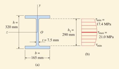
**FIG. 5-39** Example 5-14. Shear stresses in the web of a wide-flange beam
