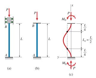
**FIG. 11-17** Buckling of a column with both ends fixed against rotation
