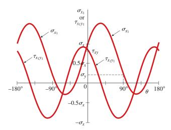
**FIG. 7-3** Graph of normal stress  $\sigma_{x_1}$  and shear stress  $\tau_{x_1y_1}$  versus the angle  $\theta$  (for  $\sigma_y = 0.2\sigma_x$  and  $\tau_{xy} = 0.8\sigma_x$ )
