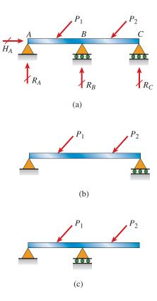
FIG. 10-5 Example of a continuous beam: (a) beam with loads and reactions; (b) released structure when the reaction at support B is selected as the redundant; and (c) released structure when the reaction at end C is selected as the redundant
