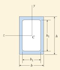
FIG. 6-47 Example 6-10. Cross section of a hollow box beam (elastoplastic material)
