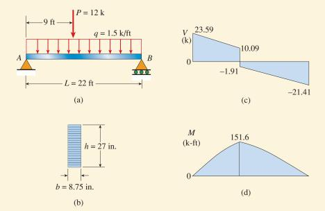
FIG. 5-14 Example 5-3. Stresses in a simple beam
