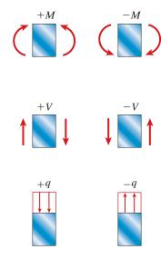
**FIG. 9-4** Sign conventions for bending moment M, shear force V, and intensity q of distributed load
