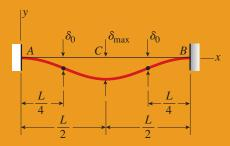
FIG. 10-11 Deflection curve for the fixedend beam of Fig. 10-9
