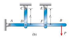
**FIG. 2-26** Statically indeterminate structure with a small misfit
