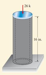
**FIG. 1-5** Example 1-1. Hollow aluminum post in compression
