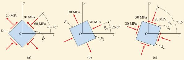
**FIG. 7-23** Example 7-6 (continued). (a) Stresses acting on an element oriented at  $\theta = 45^{\circ}$ , (b) principal stresses, and (c) maximum shear stresses
