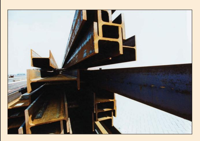
Steel members come in a wide variety of shapes; the properties of the cross section are needed for analysis and design.
