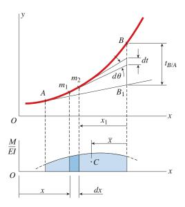
FIG. 9-23 Derivation of the second moment-area theorem
