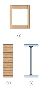
FIG. 5-41 Cross sections of typical built-up beams: (a) wood box beam, (b) glulam beam, and (c) plate girder
