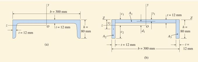
FIG. 5-16 Cross section of beam discussed in Example 5-4. (a) Actual shape, and (b) idealized shape for use in analysis (the thickness of the beam is exaggerated for clarity)
