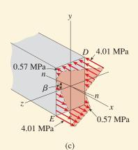
FIG. 6-17 Solution to Example 6-4.
