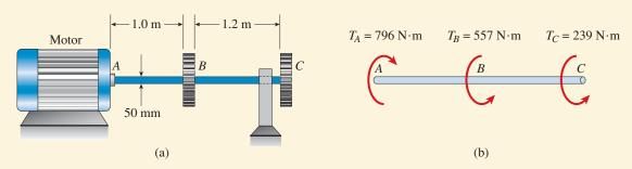
FIG. 3-31 Example 3-8. Steel shaft in torsion
