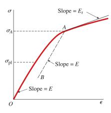
FIG. 11-31 Compression stress-strain diagram for the material of the column shown in Fig. 11-30
