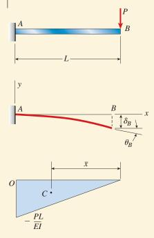
**FIG. 9-24** Example 9-10. Cantilever beam with a concentrated load
