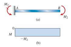
**FIG. 5-3** Cantilever beam in pure bending  $(M = -M_2)$
