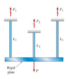
**FIG. 2-73** Elastoplastic analysis of a statically indeterminate structure
