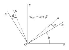
**FIG. 7-34** Shear strain  $\gamma_{x_1y_1}$  associated with the  $x_1y_1$  axes
