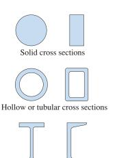
**FIG. 2-4** Typical cross sections of structural members
