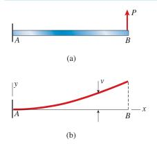
**FIG. 9-1** Deflection curve of a cantilever beam
