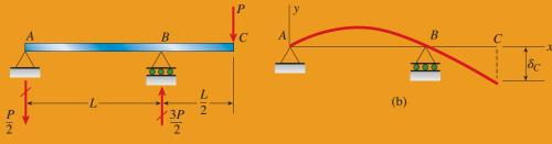
**FIG. 9-15** Example 9-5. Deflections of a beam with an overhang
