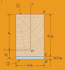
**FIG. 6-7** Example 6-1. Cross section of a composite beam of wood and steel
