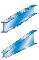
**FIG. 9-27** Beams with varying moments of inertia (see also Fig. 5-23)
