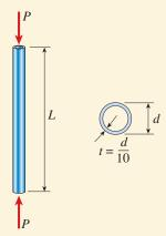
**FIG. 11-39** Example 11-7. Aluminum tube in compression
