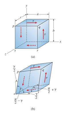
FIG. 1-28 Element of material subjected to shear stresses and strains
