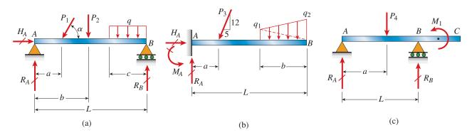
FIG. 4-2 Types of beams: (a) simple beam, (b) cantilever beam, and (c) beam with an overhang
