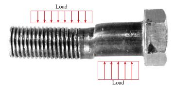
FIG. 1-26 Failure of a bolt in single shear
