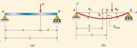
**FIG. 9-12** Example 9-3. Deflections of a simple beam with a concentrated load
