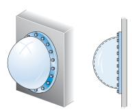
**8.2-4** A rubber ball (see figure) is inflated to a pressure of 60 kPa. At that pressure the diameter of the ball is 230 mm and the wall thickness is 1.2 mm. The rubber has modulus of elasticity E = 3.5 MPa and Poisson's ratio  $\nu = 0.45$ .
