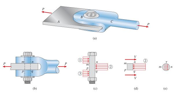
FIG. 1-24 Bolted connection in which the bolt is loaded in double shear
