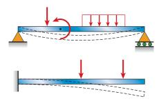
FIG. 4-1 Examples of beams subjected to lateral loads
