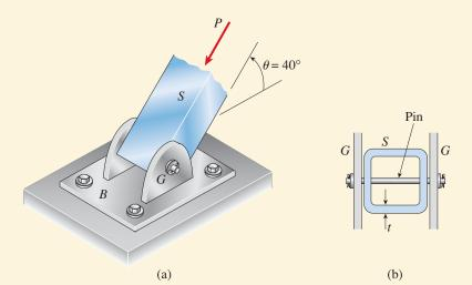
**FIG. 1-30** Example 1-5. (a) Pin connection between strut *S* and base plate *B* (b) Cross section through the strut *S*
