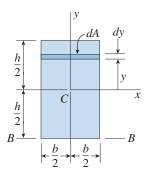
**FIG. 12-10** Moments of inertia of a rectangle (Repeated)
