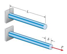
FIG. 2-5 Elongation of a prismatic bar in tension
