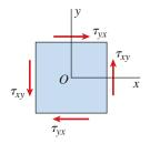
FIG. 7-5 Element in pure shear
