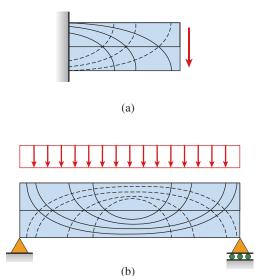
FIG. 8-14 Principal-stress trajectories for beams of rectangular cross section: (a) cantilever beam, and (b) simple beam. (Solid lines represent tensile principal stresses and dashed lines represent compressive principal stresses.)
