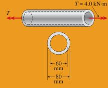
FIG. 3-26 Example 3-6. Circular tube in torsion
