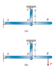
FIG. 2-25 Statically determinate structure with a small misfit
