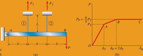
FIG. 2-75 Example 2-19. Elastoplastic analysis of a statically indeterminate structure
