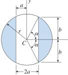
Circle with core removed (Origin of axes at center of circle)
