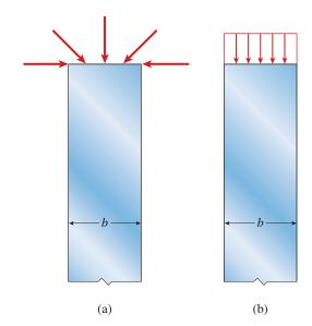
**FIG. 2-61** Illustration of Saint-Venant's principle: (a) system of concentrated loads acting over a small region of a bar, and (b) statically equivalent system
