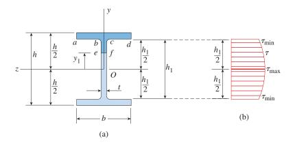
FIG. 5-38 (Repeated) Shear stresses in the web of a wide-flange beam.
