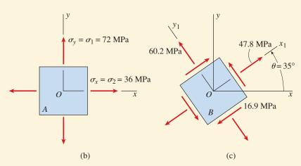
FIG. 8-10 Solution to Example 8-2
