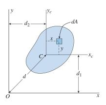
FIG. 12-13 Derivation of parallel-axis theorem (Repeated)
