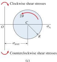
FIG. 7-17 Alternative sign convention for shear stresses: (a) clockwise shear stress, (b) counterclockwise shear stress, and (c) axes for Mohr's circle. (Note that clockwise shear stresses are plotted upward and counterclockwise shear stresses are plotted downward.)
