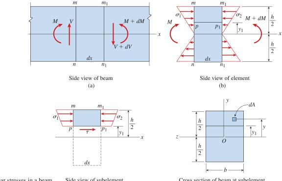
**FIG. 5-28** Shear stresses in a beam of rectangular cross section
