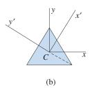
**FIG. 12-26** Examples of areas for which every centroidal axis is a principal axis and the centroid *C* is a principal point
