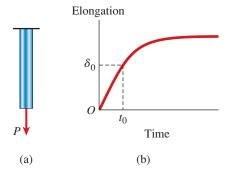
FIG. 1-20 Creep in a bar under constant load
