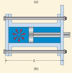
FIG. 2-52 Example 2-15. Proposed modifications to the bolts: (a) Bolts with reduced shank diameter, and (b) bolts with increased length
