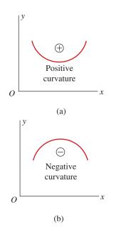
FIG. 5-6 Sign convention for curvature
