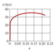
FIG. 1-13 Typical stress-strain diagram for an aluminum alloy
