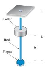
**2.8-2** Solve the preceding problem if the collar has mass M = 80 kg, the height h = 0.5 m, the length L = 3.0 m, the cross-sectional area A = 350 mm<sup>2</sup>, and the modulus of elasticity E = 170 GPa.
