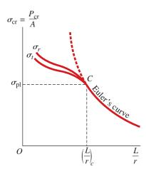
**FIG. 11-32** Diagram of critical stress versus slenderness ratio
