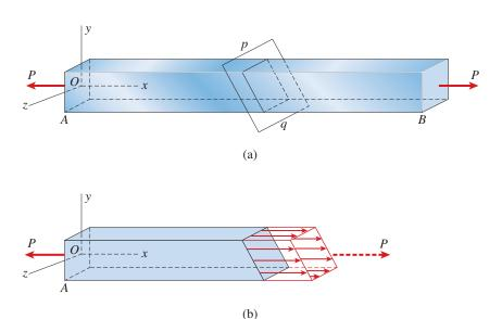
**FIG. 2-32** Prismatic bar in tension showing the stresses acting on an inclined section pq: (a) bar with axial forces P, (b) three-dimensional view of the cut bar showing the stresses, and (c) two-dimensional view
