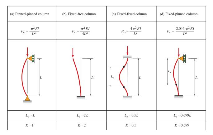
FIG. 11-19 Critical loads, effective lengths, and effective-length factors for ideal columns
