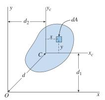
Equations (12-11a) and (12-11b) represent the **parallel-axis theorem for** moments of inertia:
