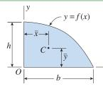
**Semisegment of** *n***th degree** (Origin of axes at corner)
