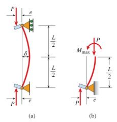
FIG. 11-26 Column with eccentric axial loads
