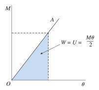
FIG. 9-31 Diagram showing linear relationship between bending moments M and the angle  $\theta$
