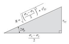
**FIG. 7-10** Geometric representation of Eq. (7-11)
