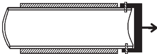
FIGURE 5.10 A mandrel to manufacture composite pipes.
