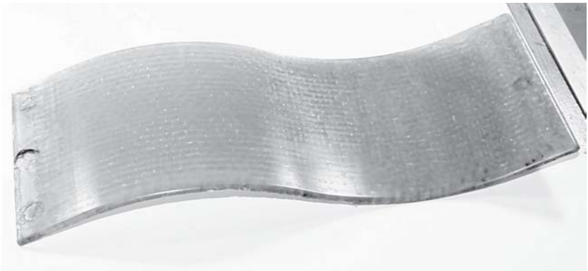
FIGURE 1.4(a) A curved piece made by Liquid Composite Molding (LCM) method.
