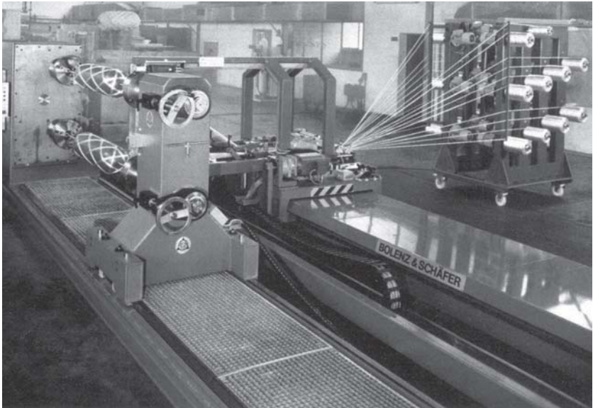
FIGURE 1.2(c) A two-spindle winder with a carriage-mounted resin bath and a free-standing creel in the background (courtesy of Composites Technology magazine, August 2005).
