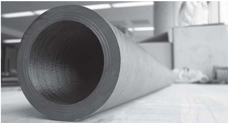
FIGURE 1.6(a) A thermoplastic composite tube made by the fiber placement process.
