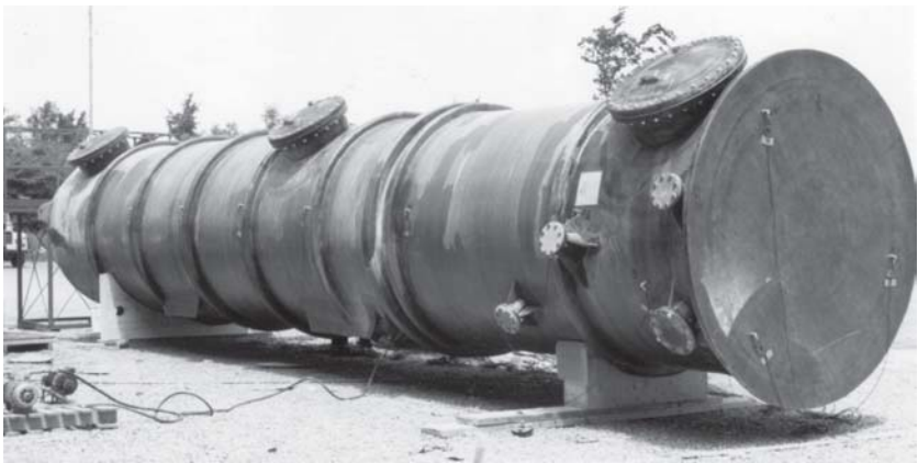
FIGURE 1.2(a) Composite pressure vessel made by combination of hand-lay-up and filament winding.
