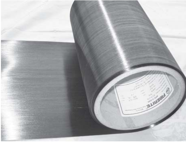
FIGURE 8.4 Photo of a roll of unidirectional tape made of carbon/PEKK.
