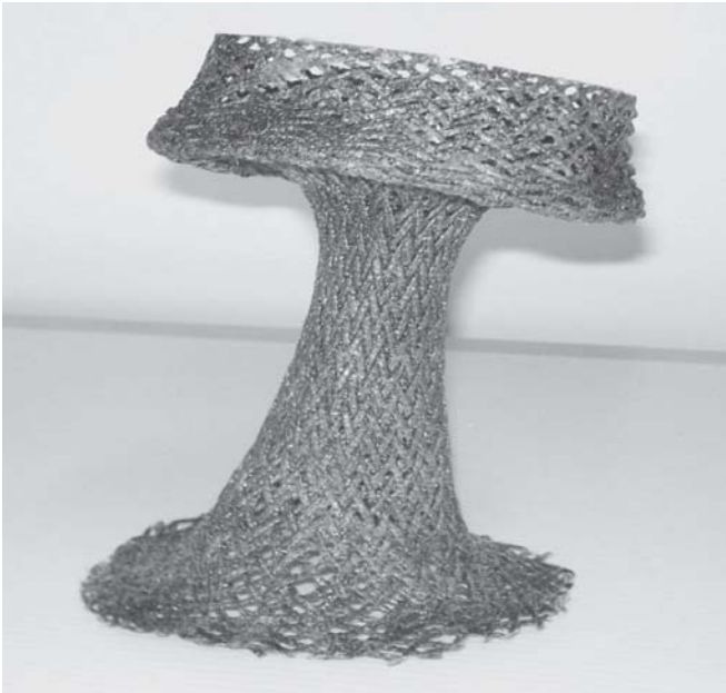
FIGURE 7.10 Preform made by braiding.
