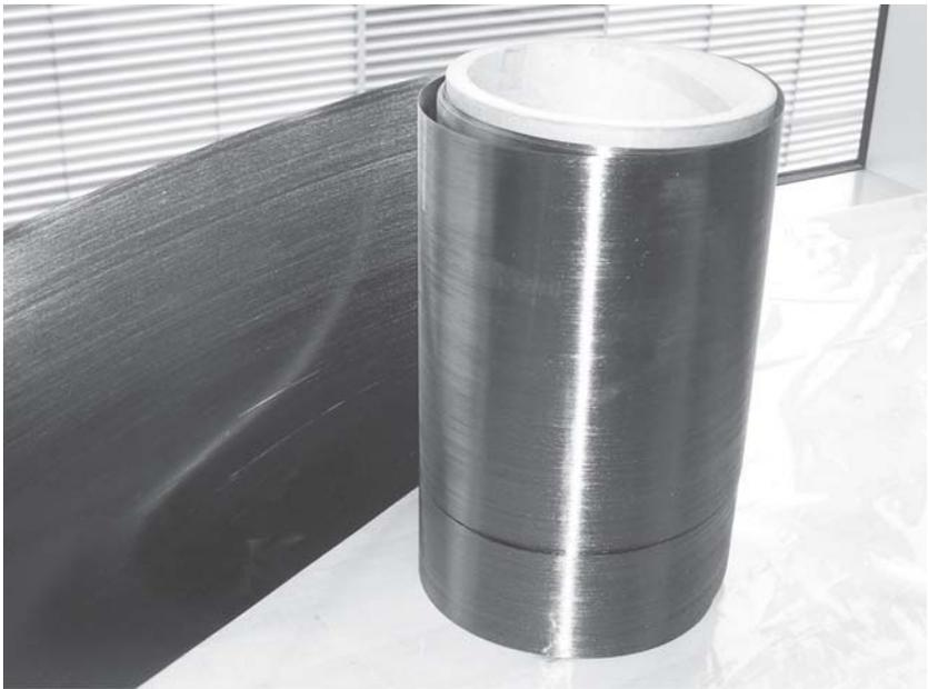
**FIGURE 4.4** A roll and a sheet of carbon/epoxy prepreg.
