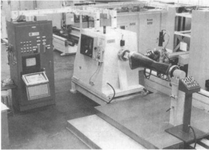
**Fig. 5.6** An automatic tape placement system in use at Bell Helicopter from Automated Dynamics Corporation literature.
