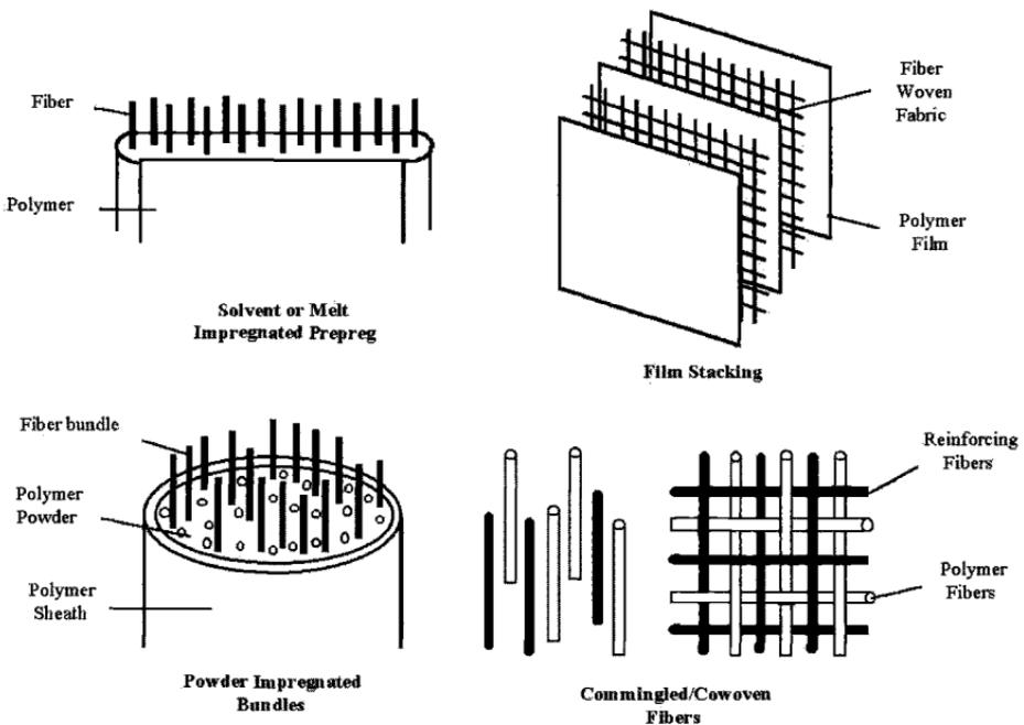
Fig. 5.33 Intermediate material forms for thermoplastic composites.
