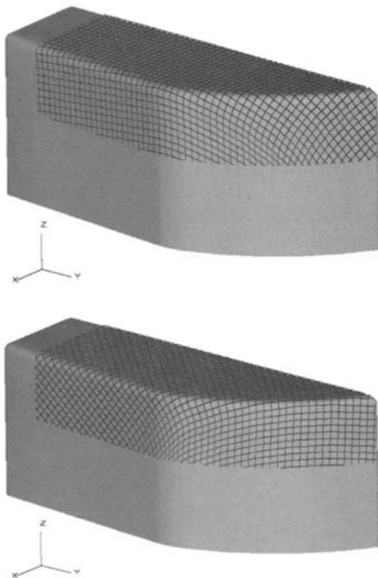
**Fig. 5.25 Kinematic draping predictions for different fabric orientations.**
