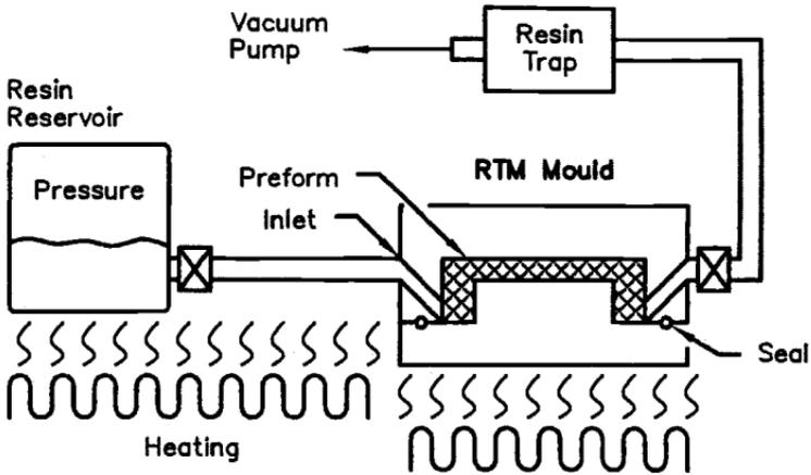
Fig. 5.13 Resin transfer molding (RTM) process.
