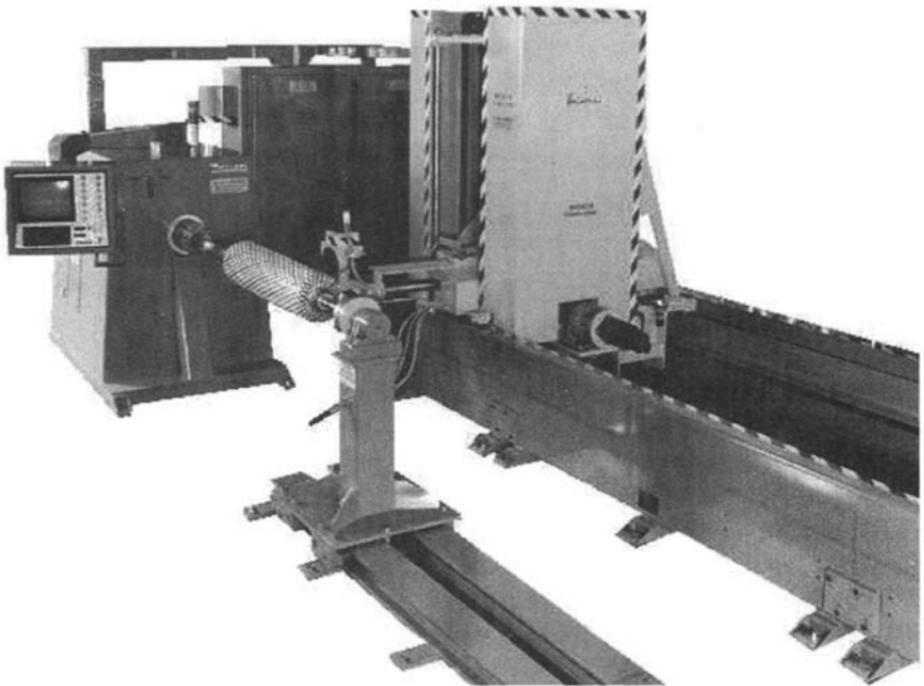
**Fig. 5.19** Filament winding machine. Courtesy McClean-Anderson, Schofield, Wisconsin.
