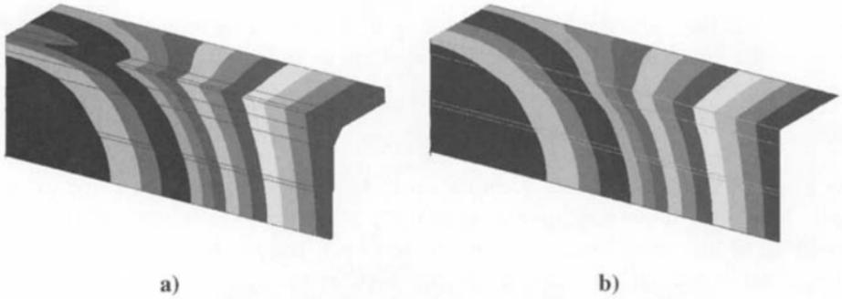
**Fig. 5.28** Sequential predicted flow fronts for RTM of a composite I-beam (quarter section). Resin inlet is at lower left. a) Three-dimensional flow simulation; b) two-dimensional flow simulation.
