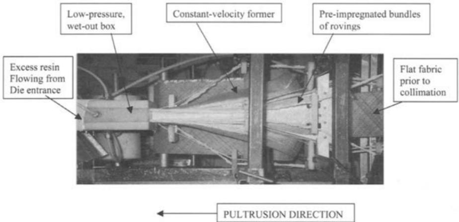
**Fig. 5.23 Infeed system for a pultrusion process.**
