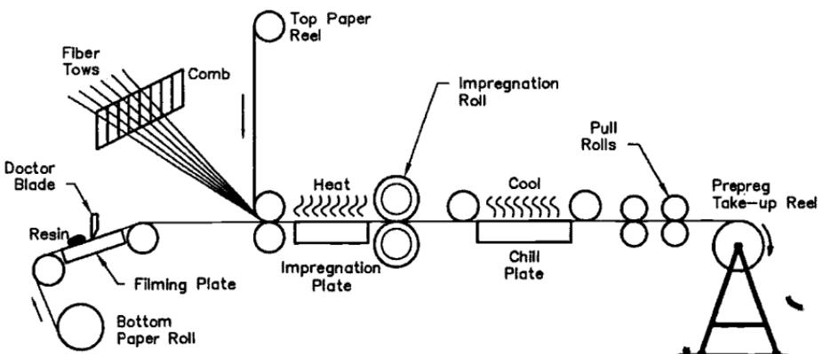
Fig. 5.2 Schematic illustration of hot-melt film pre-pregging process. Adapted from Ref. 2.
