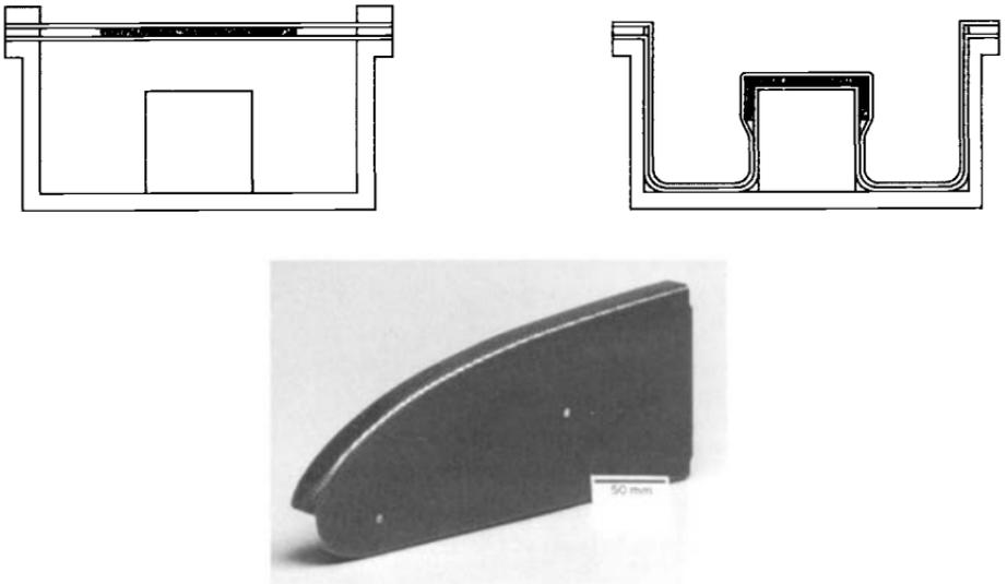
Fig. 5.4 Schematic diagram of the diaphragm-forming process; below, carbon fiber-epoxy rib made using this process.
