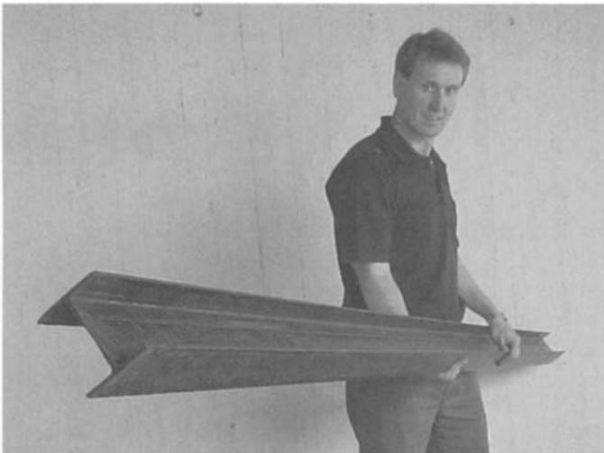
**Fig. 5.24** Prototype, structural I-beam, produced using carbon fiber tows and NCFs with an epoxy resin system. Courtesy of CRC-ACS Ltd, Australia.
