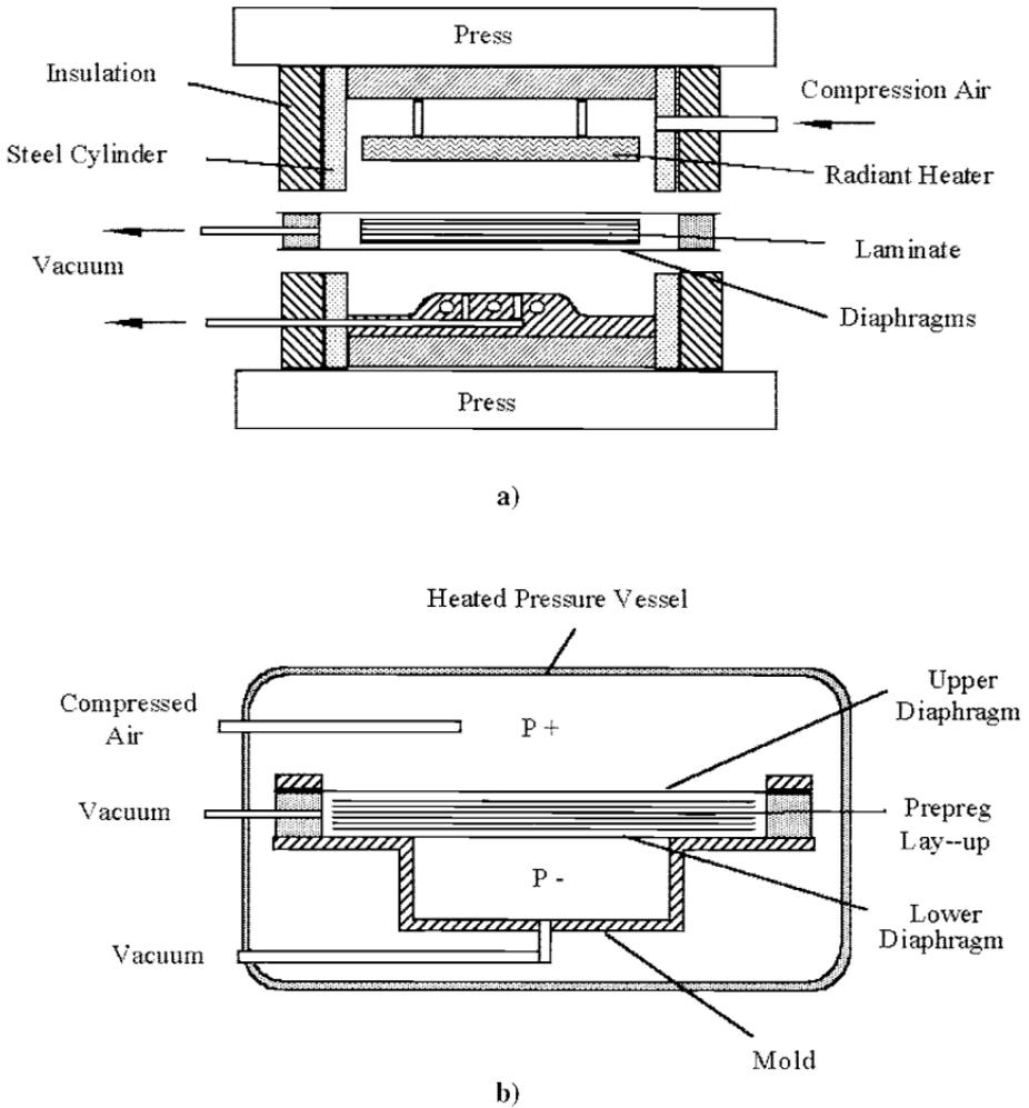
**Fig. 5.35 Diaphragm forming a thermoplastic composite part: a) in autoclave; b) in mold.**
