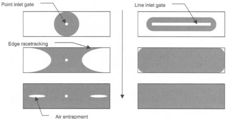
**Fig. 5.15** Alternative gating arrangements for the RTM process, showing possible defects.
