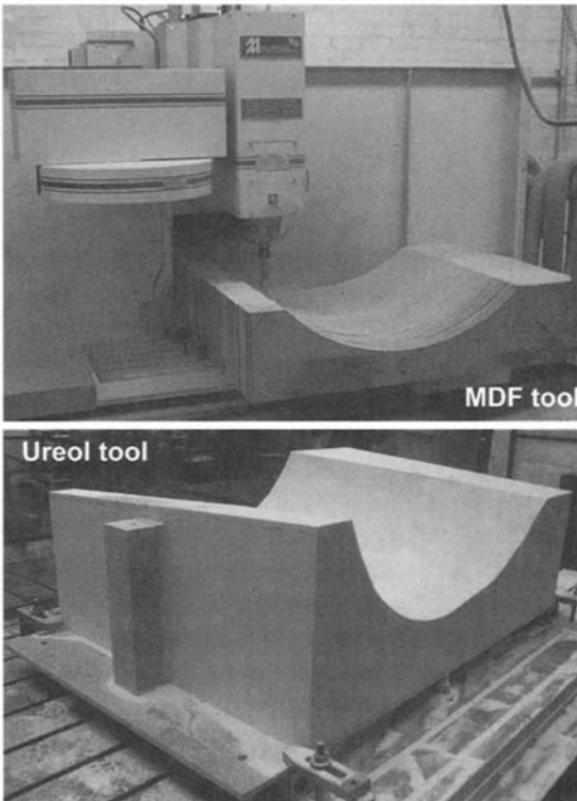
**Fig. 5.30** Medium-density fiberboard (MDF) and Ureol tooling.
