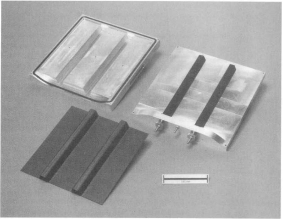
**Fig. 5.1** Matched-die mold and resulting top-hat stiffened component.
