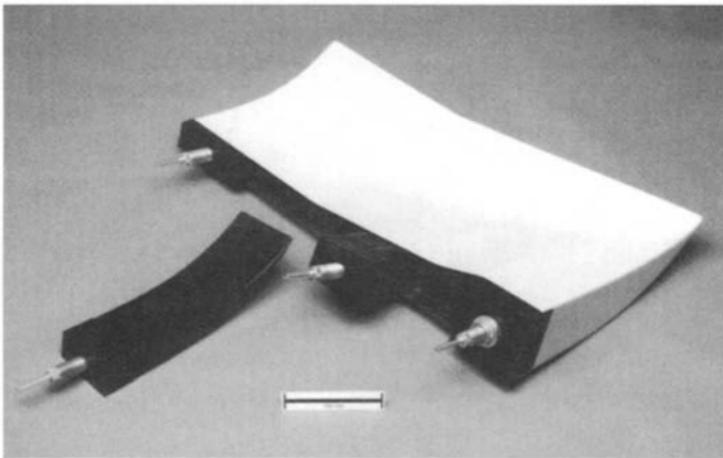
Fig. 5.31 Airpad brand inflatable tooling.
