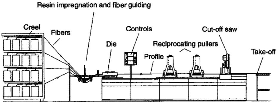
**Fig. 5.22 Schematic diagram of basic pultrusion machine (Reference 11).**
