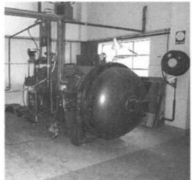
**Fig. 5.8** Layout of an autoclave and, *right*, a small typical autoclave.
