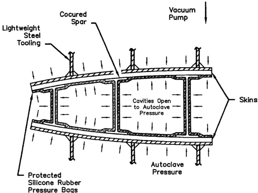
**Fig. 5.11** Schematic diagram of the tooling used to make a cocured carbon/epoxy wing structure, using rubber bladder expansion for internal pressurization. Adapted from Ref. 3.
