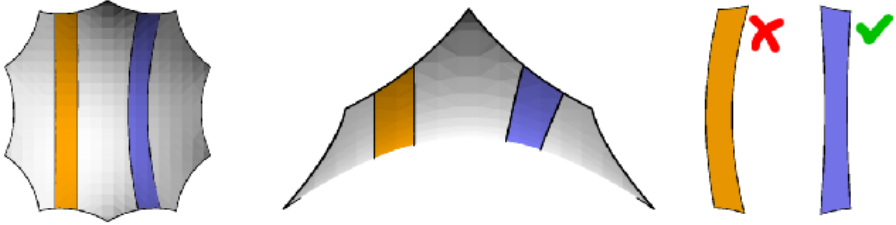
Fig. 2. Non-geodesic (lighter cloth), and geodesic (darker cloth) patterns
