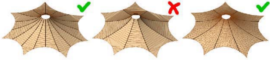
Fig. 4. Planarisation: (a) Large structure simple triangle development, (b) Small structure triangle development, (c) Small structure deformation minimising flattening
