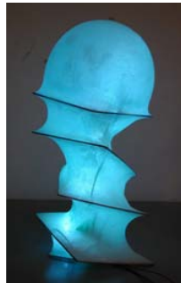
Fig. 6. Rigidized inflatable structure (A. Pronk)
