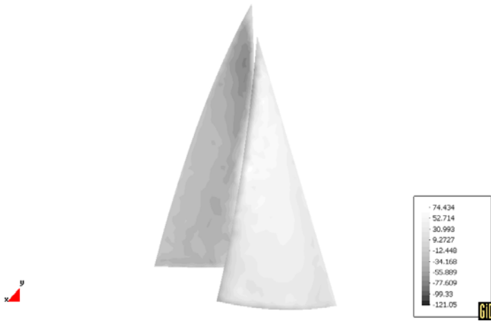
Fig. 4. Interaction of a genoa and a main sail - pressures at the end of the coupled analysis
