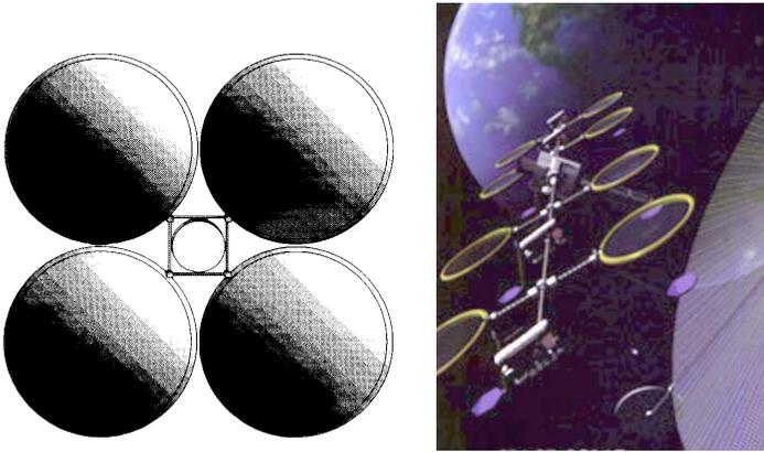
**Fig. 4.** Concept for a solar sailing spacecraft with four 2,500-m<sup>2</sup> saillets.(left); the “Sun Tower” solar power station builds on gossamer structures: supporting tori and flexible Fresnel-lens concentrators (right) (NASA picture)
