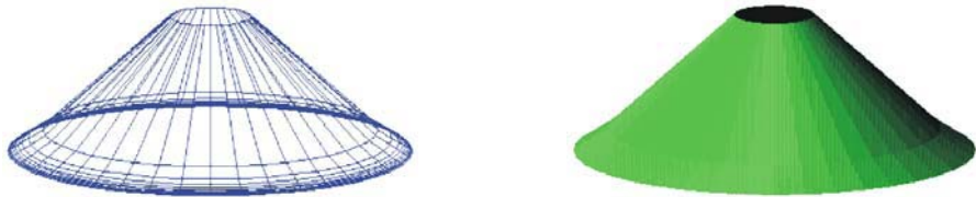
Fig. 2. Catenoid with anisotropic pre-stress (meridian/ring=3/1).
