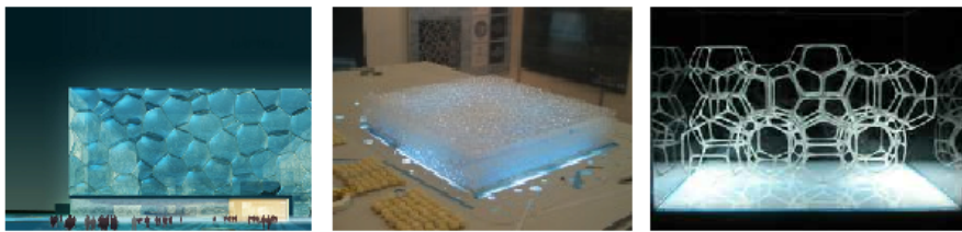
Figs. 44-46. The Rendering, model and structure model shows the three dimensional arrangement of the polyhedral structure, a common natural pattern seen in water bobbles and organic cells. The building envelope acts as an very efficient green house where 90% area. [Ove Arup Pty Ltd, www.ptw.com.au]
