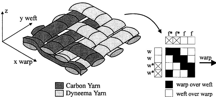
3.3 Extended checkerboard pattern of a hybrid 2 × 2 twill weave unit cell. The w and f type yarns are Dyneema® fibres, and the w\* and f\* type yarns are carbon fibres.
