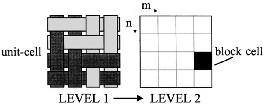
3.6 Schematic of a hybrid twill weave unit cell (level 1) and a block cell (level 2).
