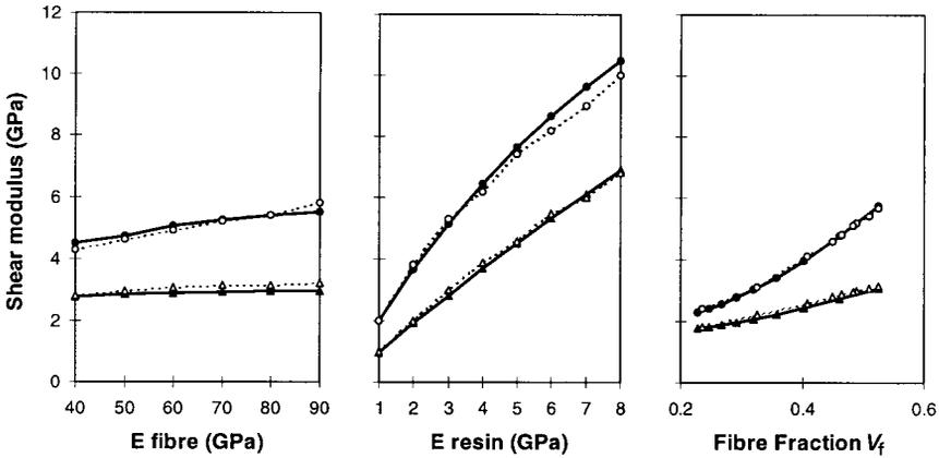
3.11 Predicted shear moduli for the benchmark composite: comparing results from an FEM study [24] and our CEM calculations (material: glass-epoxy plain weave).  $\blacktriangle$   $G_{yz} = G_{zx}$  (CEM);  $\bullet$   $G_{xy}$  (CEM);  $\triangle$   $G_{yz} = G_{zx}$  (FEM);  $\circ$   $G_{xy}$  (FEM).
