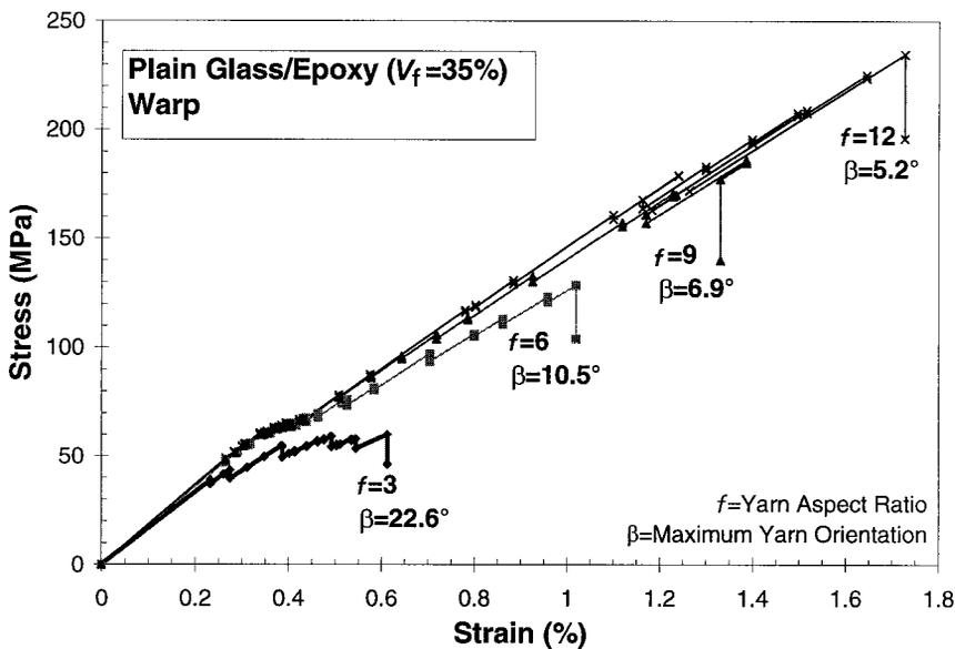
3.13 Predicted warp stress–strain curves as a function of the yarn aspect ratio  $f$ .
