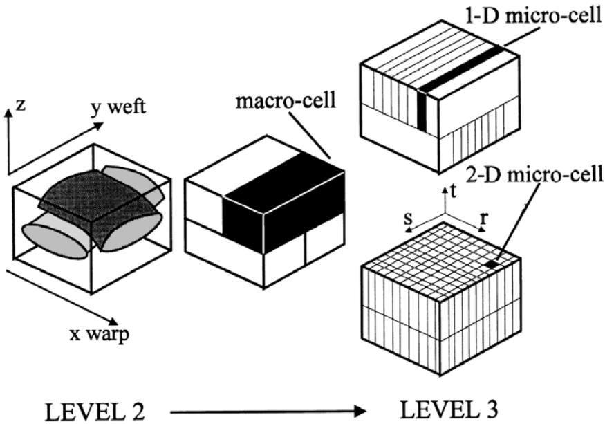
3.7 Schematic of a block cell or macro-cell (level 2) and a micro-cell (level 3).
