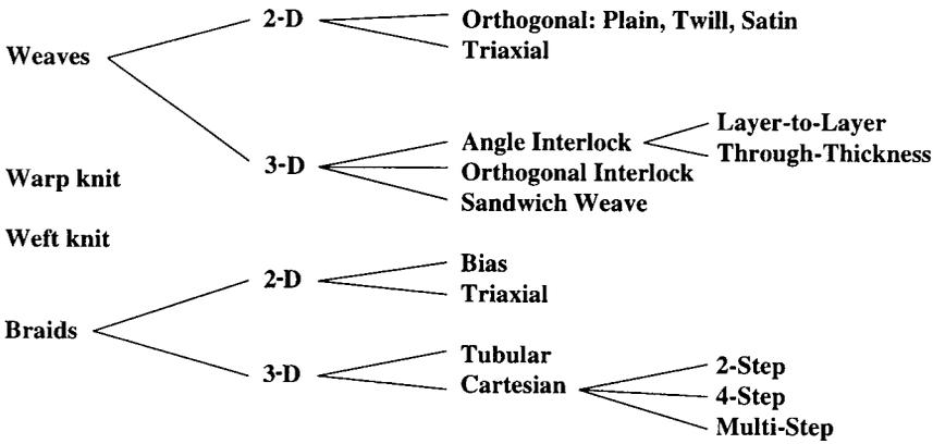
3.1 Classification of textile preforms for composite structures [3].
