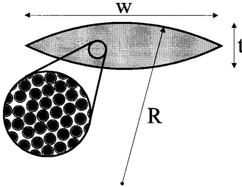
3.4 Lenticular yarn cross-section.  $W$  is width of yarn,  $t$  is yarn thickness,  $R$  is radius of curvature.
