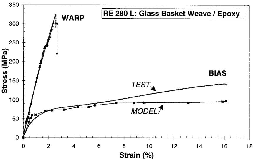
3.15 Theoretical and experimental stress-strain curves in warp and bias directions.
