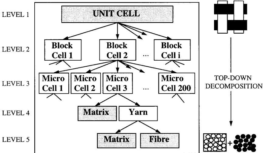
3.5 Multilevel decomposition of woven fabric composites: top-down.
