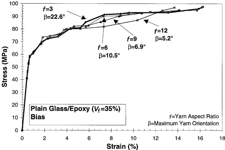
3.14 Predicted bias stress–strain curves as a function of the yarn aspect ratio  $f$ .
