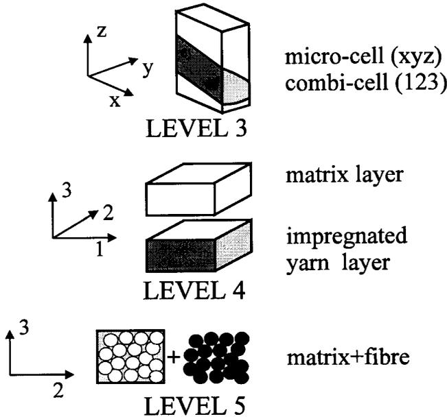
3.8 Schematic of a micro-cell or combi-cell (level 3), matrix and yarn layers (level 4) and a unidirectional lamina with fibre and matrix phases (level 5).
