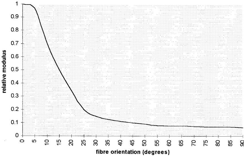
9.1 Typical variation of modulus with fibre orientation.
