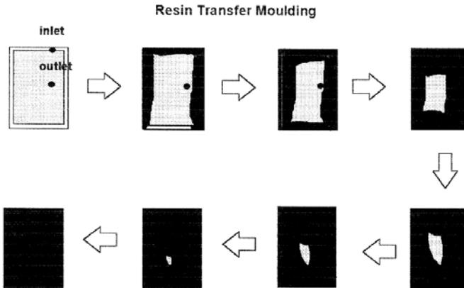
9.8 Sequence of mould filling using peripheral gating and off-centre vacuum exit.
