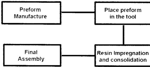
9.7 Liquid moulding of composites using preforms.
