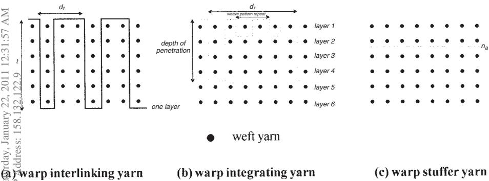
(a) warp interlinking yarn (b) warp integrating yarn (c) warp stuffer yarn
