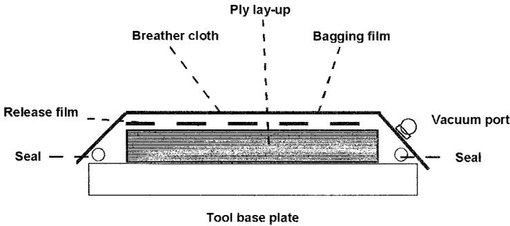
9.2 Vacuum bagging process for the production of composites.
