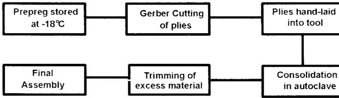
9.3 Route for composites production using the autoclave process.
