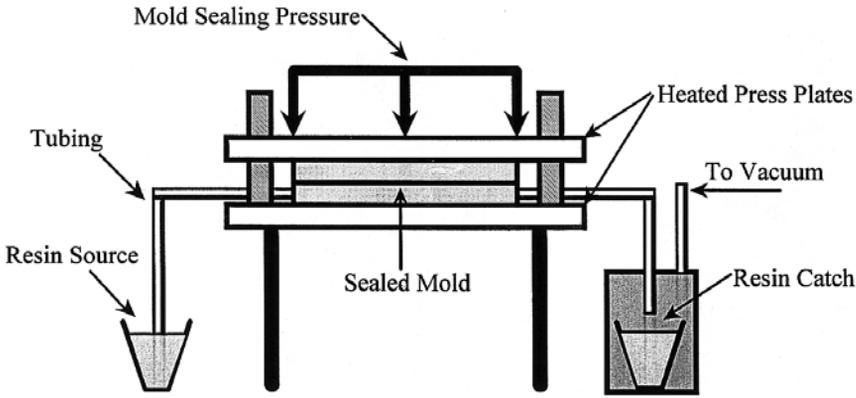
7.12 Schematic of typical RTM set-up for braid consolidation.
