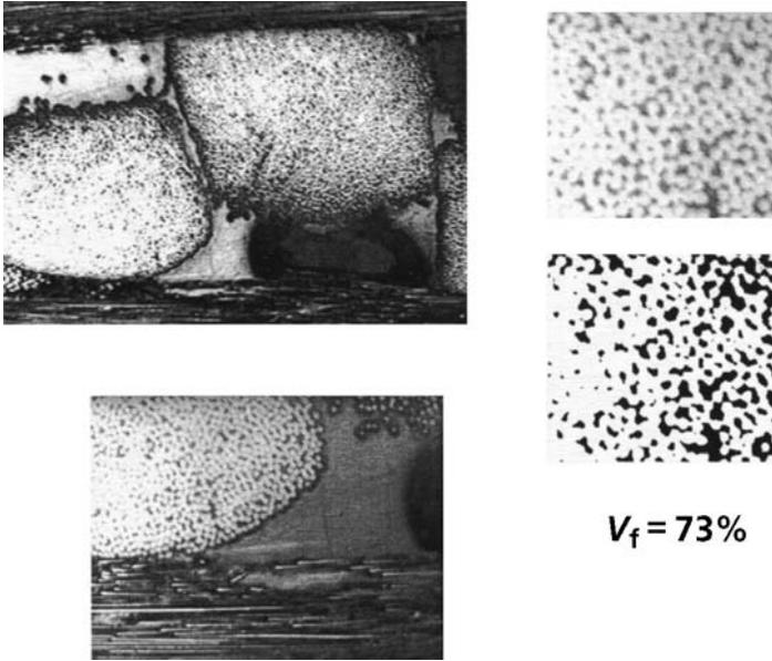
7.16 Measurement of the fiber volume fractions for the four-step  $1 \times 1$  Kevlar braider, transversely inserted carbon fiber, hybrid composite sample.
