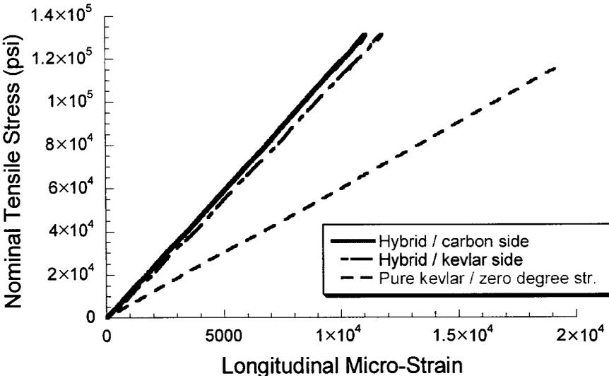
7.18 Nominal tensile stress vs. longitudinal strain for pure Kevlar and Kevlar/carbon hybrid tension samples.
