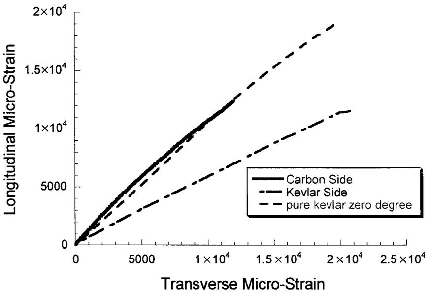
7.17 Longitudinal vs. transverse strain in pure Kevlar and Kevlar/carbon hybrid tension samples.
