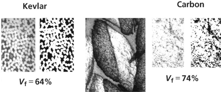
7.15 Measurement of fiber volume fractions for the two-sided braided hybrid composite sample through digital analysis.
