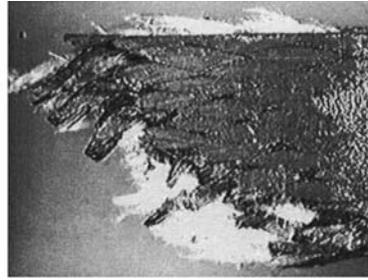
7.19 Typical fracture of braided composite specimens (left) and fracture across the shear face in the Kevlar/carbon hybrid sample (right) (compliments of the Center for Composite Materials, University of Delaware).
