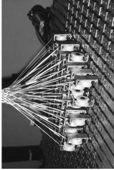
7.9 A Cartesian (four-step) pneumatic braider with axial yarn insertion (compliments of the Center for Composite Materials, University of Delaware).
