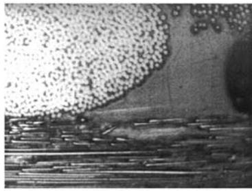
7.14 Cross-sectional microstructure of a four-step braided composite with transverse carbon tow insertion.
