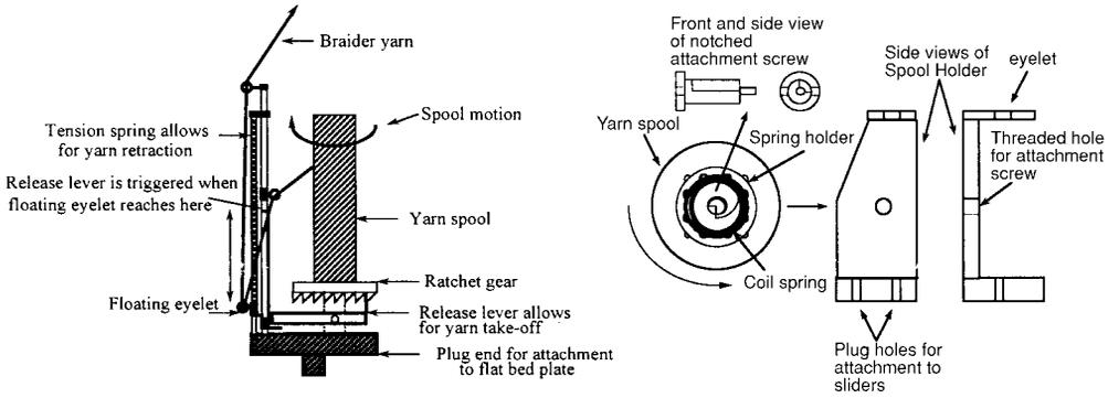
7.11 Schematics of conventional and adapted yarn carriers utilized in braiding 2-D and 3-D preforms, respectively (adapted yarn carrier schematics compliments of Atlantic Research Corporation).
