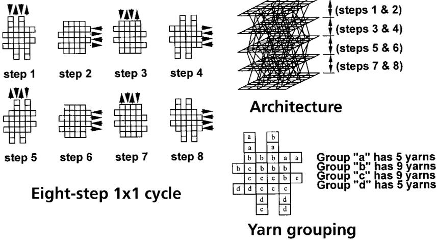
7.7 Sample multiple step cycle showing idealized architecture (repeat geometry) and yarn grouping.
