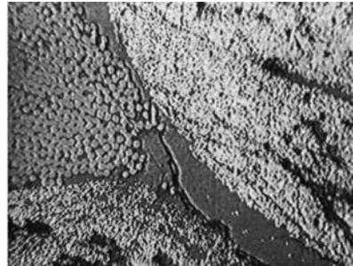
7.20 Micrographs showing crack initiation at a void within the intertow regions and propagation along the matrix/tow interface and crack arrest at the Kevlar interface.
