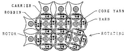
7.5 Method of advanced 3-D solid braiding (compliments of Toyoda Automatic Loom Works, Ltd).
