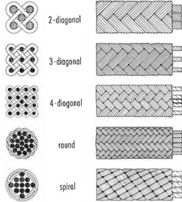
7.4 Solid braid fabrication and geometry.
