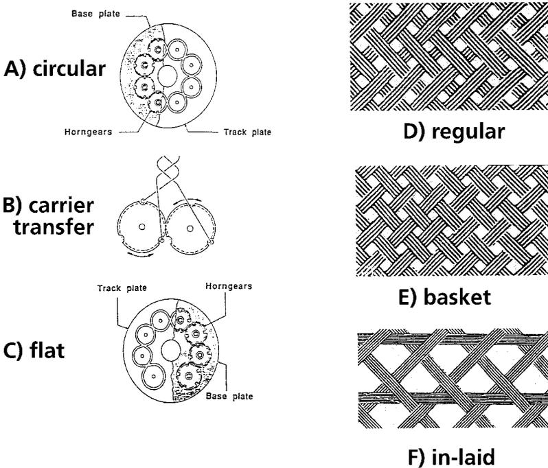
7.1 Mechanisms and samples of 2-D braids after [1].
