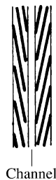
Figure 2.5. Carbon nanofiber with the carbon layers oriented like a fishbone. The structure is like a stack of ice cream cones with the tip of each cone cut off, thus resulting in a hollow channel at the center
