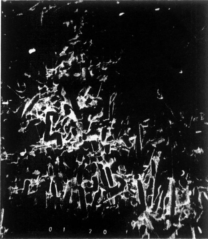
**FIGURE 3.15** Fracture surface of a randomly oriented discontinuous fiber composite showing the evidence of fiber pullout.
