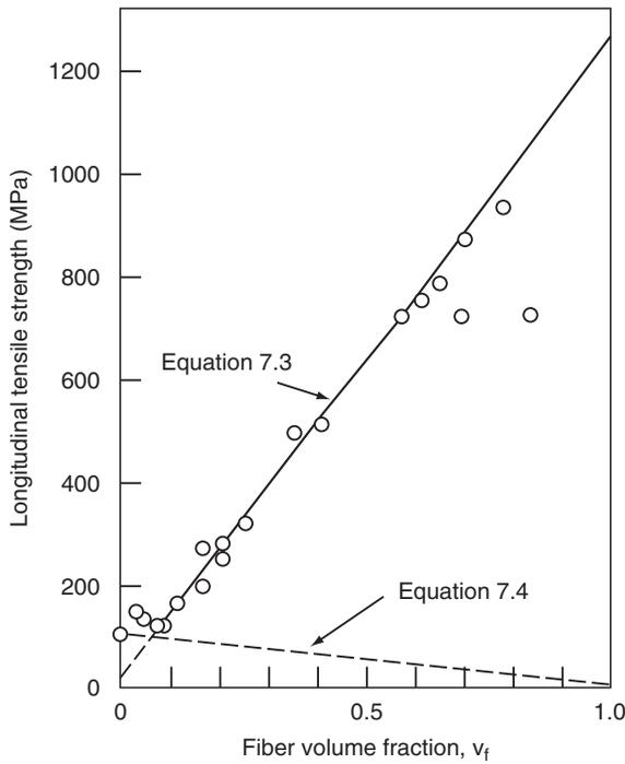
**FIGURE 7.2** Longitudinal tensile strength variation of a unidirectional continuous tungsten fiber/copper matrix composite at various fiber volume fractions. (Adapted from Kelly, A. and Davies, G.J., *Metall. Rev.*, 10, 1, 1965.)
