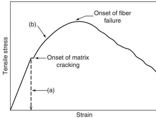
**FIGURE 7.10** Schematic tensile stress–strain diagrams of ceramic matrix composites.
