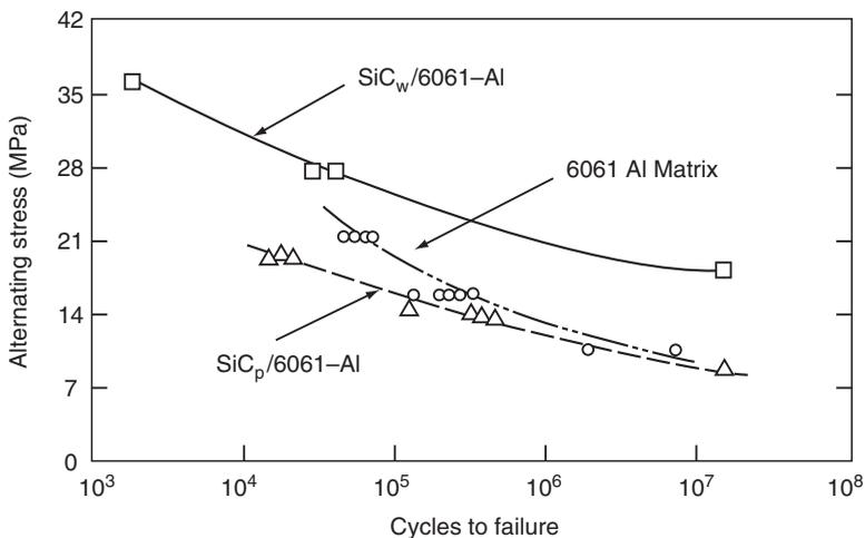
**FIGURE 7.5** *S-N* curves for  $\text{SiC}_w$ - and  $\text{SiC}_p$ -reinforced 6061 aluminum alloy. (Adapted from Rack, H.J. and Ratnaparkhi, P., *J. Metals*, 40, 55, 1988.)
