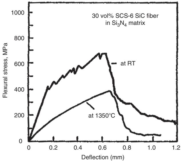
**FIGURE 7.14** Flexural stress–deflection diagrams of unidirectional 30 vol% SiC (SCS-6)-reinforced hot-pressed  $\text{Si}_3\text{N}_4$ . (Adapted from Thomson, B. and LeCostaonec, J.F., *SAMPE Q.*, 22, 46, 1991.)
