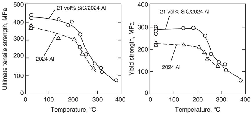
**FIGURE 7.6** Effects of increasing temperature on the ultimate tensile strength and yield strength of unreinforced and 21 vol% SiC-reinforced 2024 aluminum alloy. (Adapted from Nair, S.V., Tien, J.K., and Bates, R.C., *Int. Metals Rev.*, 30, 275, 1985.)
