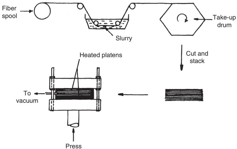
**FIGURE 7.15** Powder consolidation process for manufacturing CMC.
