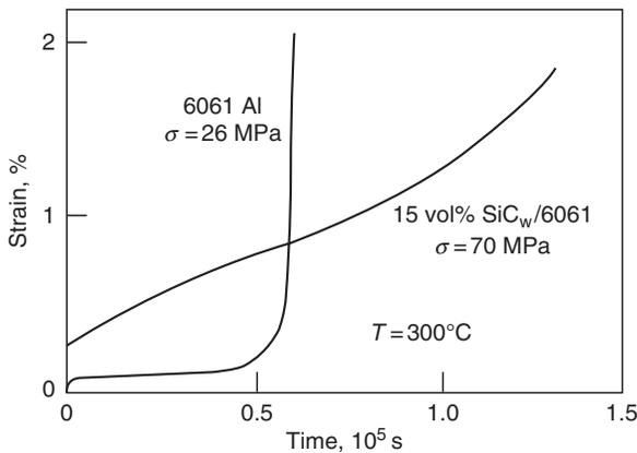
**FIGURE 7.7** Comparison of creep strains of unreinforced and 15 vol% SiC<sub>w</sub>-reinforced 6061 aluminum alloy. (Adapted from Morimoto, T., Yamaoka, T., Lilholt, H., and Taya, M., *J. Eng. Mater. Technol.*, 110, 70, 1988.)
