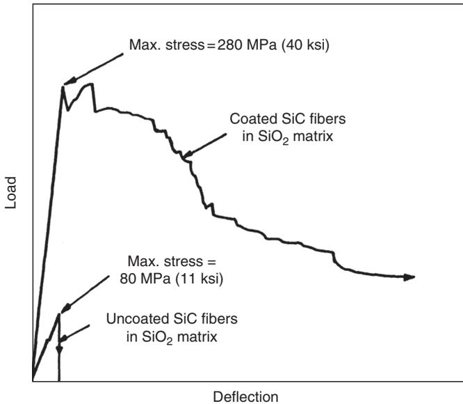
**FIGURE 7.13** Effect of fiber surface coating on the room temperature flexural load-deflection diagrams of SiC (Nicalon)-reinforced SiO<sub>2</sub>. (Adapted from Rice, R.W. and Lewis, D., III, *Reference Book for Composites Technology*, Vol. 1, S.M. Lee, ed., Technomic Pub. Co., Lancaster, PA, 1989.)
