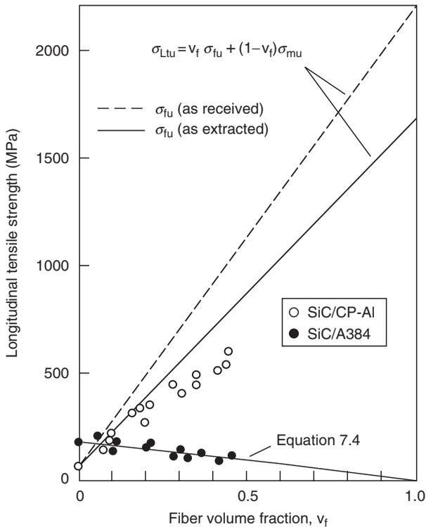
**FIGURE 7.3** Longitudinal tensile strength variation of a unidirectional continuous SiC fiber-reinforced high-purity aluminum and A384 aluminum alloy composites at various fiber volume fractions. (Adapted from Everett, R.K. and Arsenault, R.J., eds., *Metal Matrix Composites: Processing and Interfaces*, Academic Press, San Diego, 1991.)
