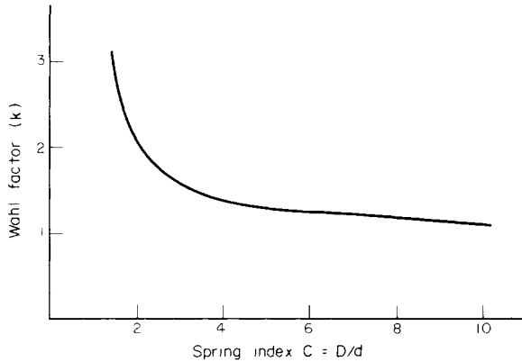
Fig. 12.6. Wahl correction factors for maximum shear stress.
