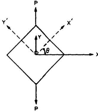
Fig. 8.31. Alternative coordinates to which strains may be referred.
