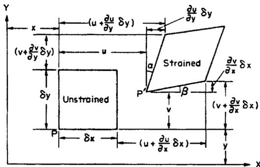
Fig. 8.30. Deformations under load in the XY plane.
