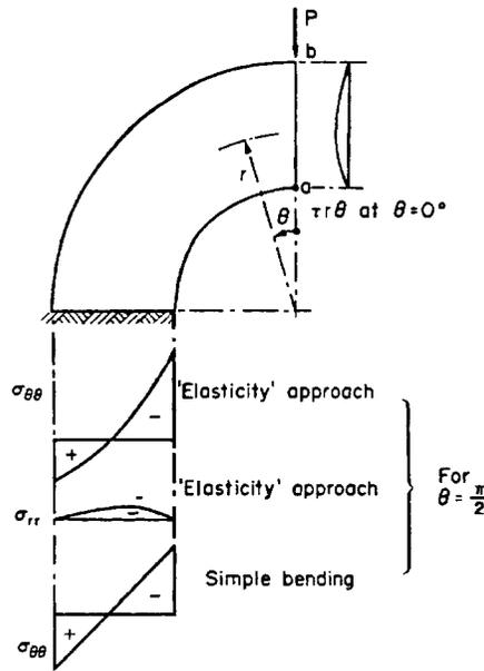
Fig. 8.34. Shear loading of a curved cantilever.
