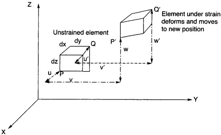
Fig. 8.29. Deformation of a cubical element under load.
