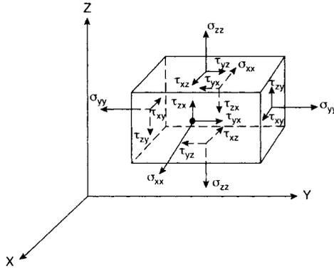
Fig. 8.1. The cartesian stress components.
