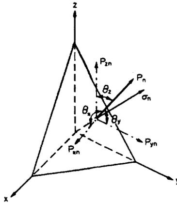
Fig. 8.7. Line of action of resultant stress.
