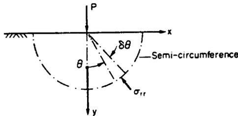
Fig. 8.39. Concentrated load on a semi-infinite plate.
