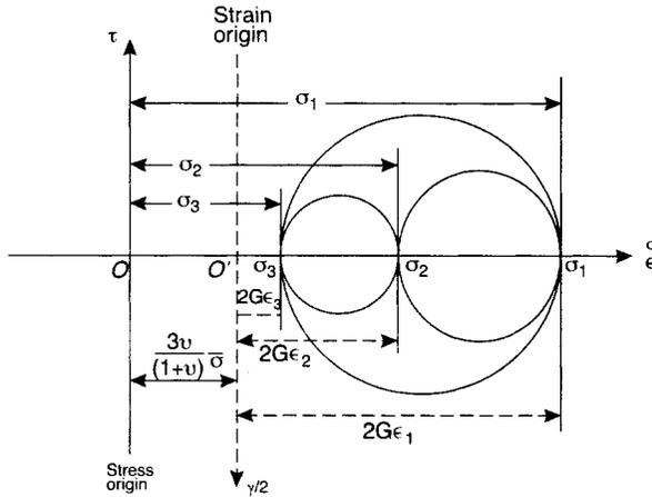
Fig. 8.12. The “combined Mohr diagram” for three-dimensional stress and strain systems.
