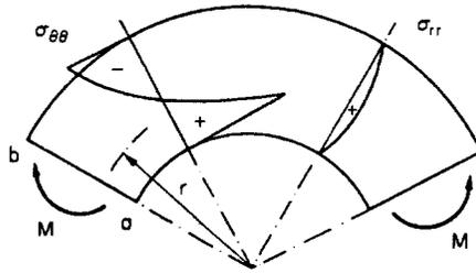
Fig. 8.33. Pure bending of a curved beam.
