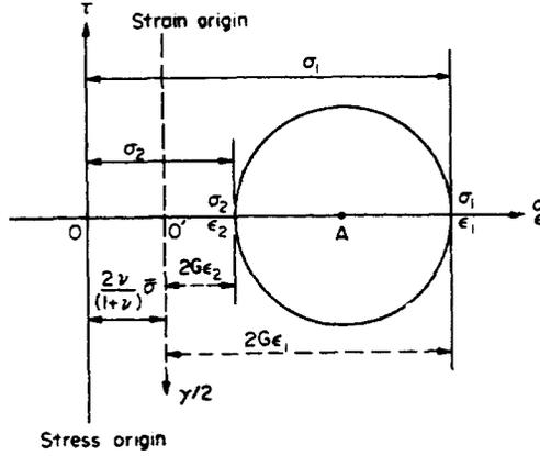
Fig. 8.13. Combined Mohr diagram for two-dimensional stress and strain systems.
