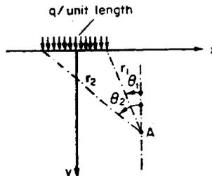
Fig. 8.41. A distributed force on a semi-infinite plate.
