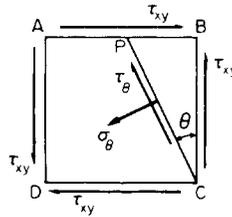
Fig. 13.2. Stresses on an element subjected to pure shear.
