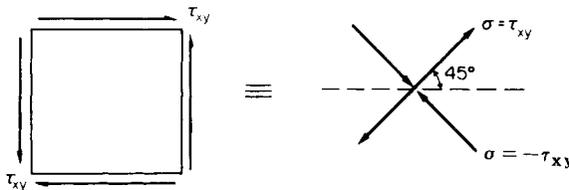
Fig. 13.3. Direct stresses due to shear.
