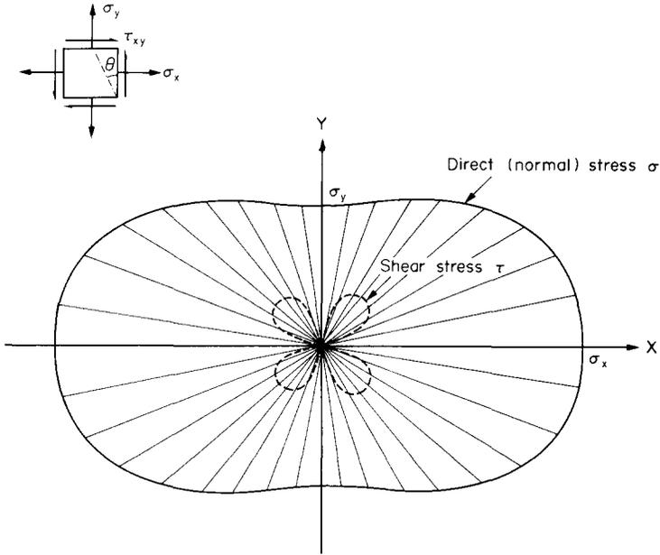
Fig. 13.15. Polar plot of stress distribution under typical biaxial applied stress system.
