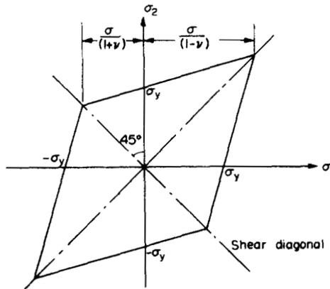
Fig. 15.7. Maximum principal strain failure envelope.
