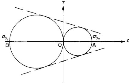
Fig. 15.2. Simplified Mohr theory on  $\sigma$ - $\tau$  axes.
