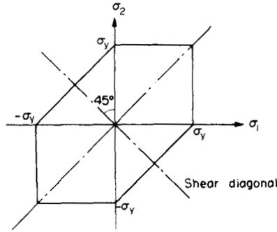
Fig. 15.6. Maximum shear stress failure envelope.
