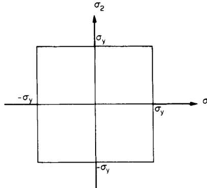
Fig. 15.5. Maximum principal stress failure envelope (locus).
