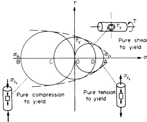
Fig. 15.1. Mohr theory on  $\sigma$ - $\tau$  axes.
