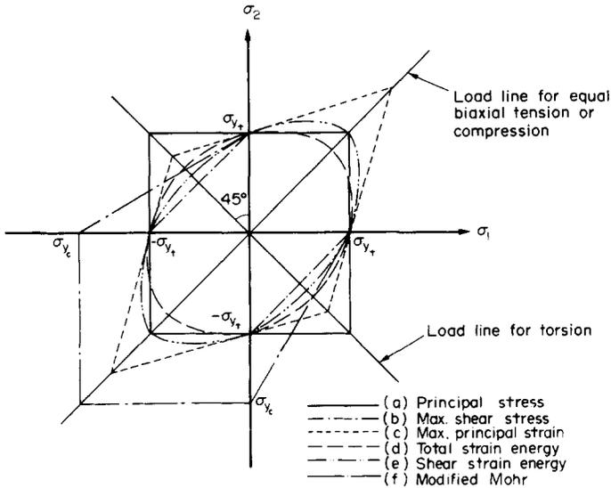
Fig. 15.12. Combined yield loci for the various failure theories.
