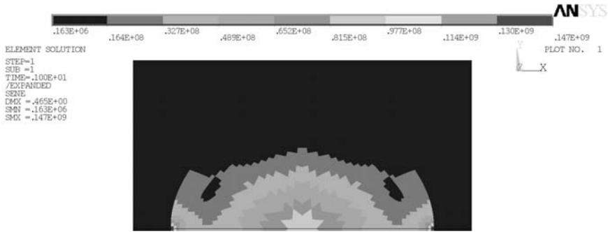
**Figure 2.97.** Relative error of the strain energy determination  $\chi$ <sup>22</sup>
